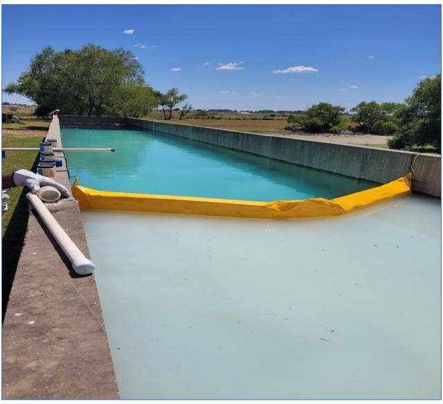
Figure 11. Floating Turbidity Barrier Evaluation Test System.
