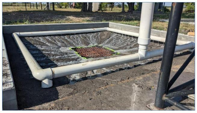
Figure 8. Soil Surface Drop Inlet Evaluation Test System.
