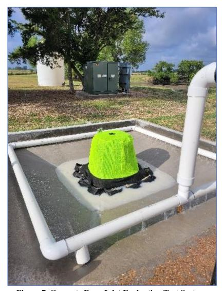
Figure 7. Concrete Drop Inlet Evaluation Test System.
