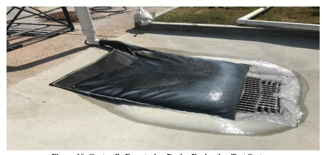
Figure 10. Geotextile Dewatering Device Evaluation Test System.
