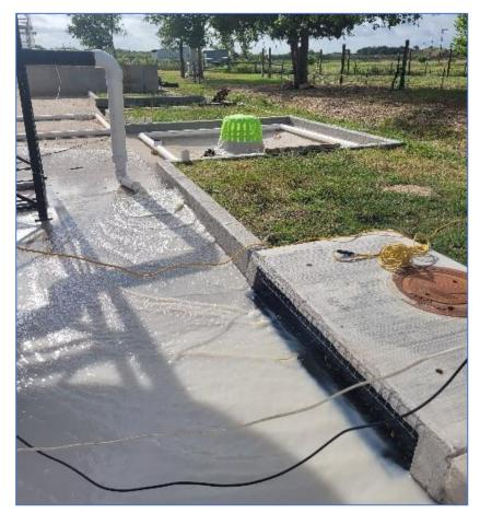
Figure 6. Curb/Gutter Protection Evaluation Test System.
