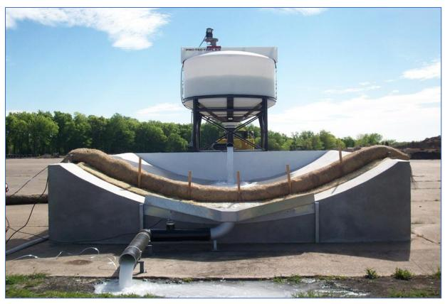
Figure 9. Channel/Perimeter Protection Evaluation Test System.
