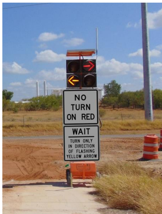
Figure 24. Proceed Left Four-Section Stacked DAD.
