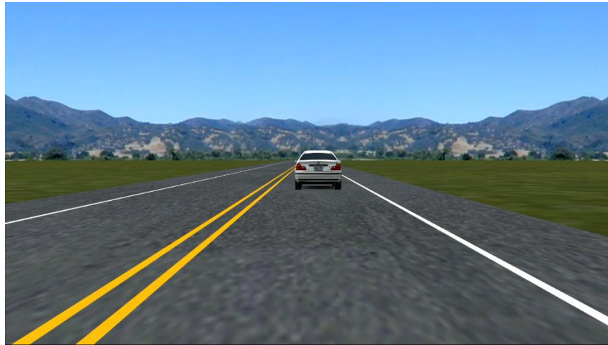
Figure 8. Standard 1-ft Centerline Striping Image—Treatment 1.
