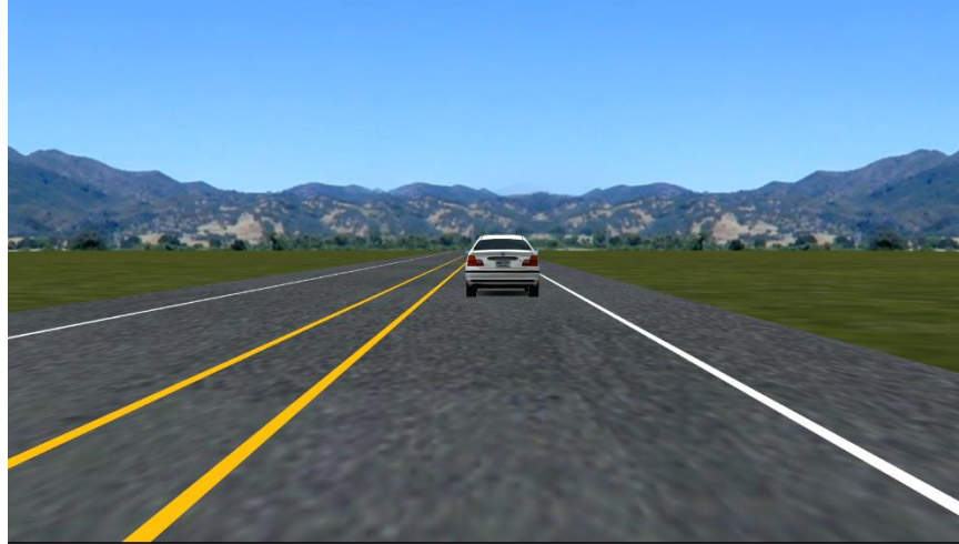
Figure 10. Experimental 4-ft Centerline Buffer Image—Treatment 3.
