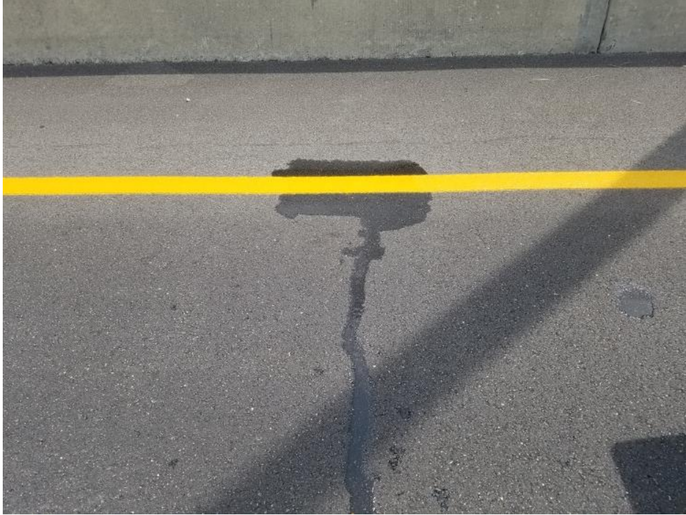
Figure 1. Yellow Marking after Wet Retroreflectivity Evaluation.
