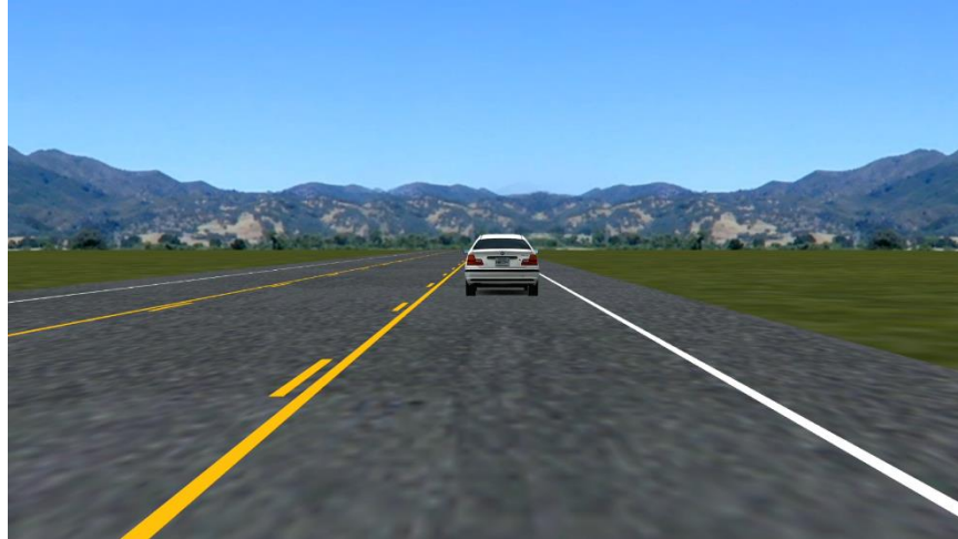
Figure 13. TWLTL 16-ft Centerline Striping Image—Treatment 6.
