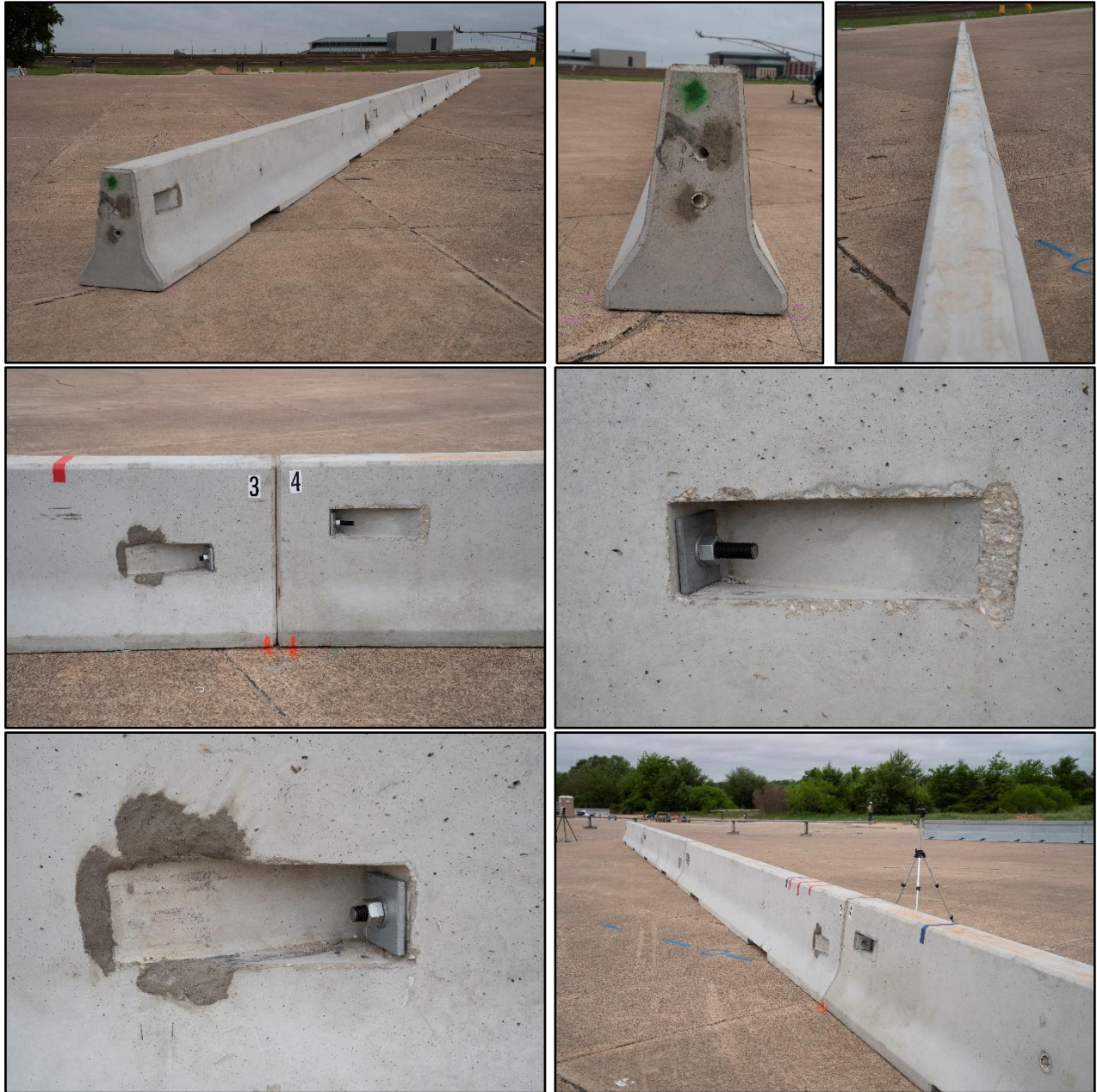
Figure 2.2. F-Shape PCB with X-Bolt Connection prior to Testing.
