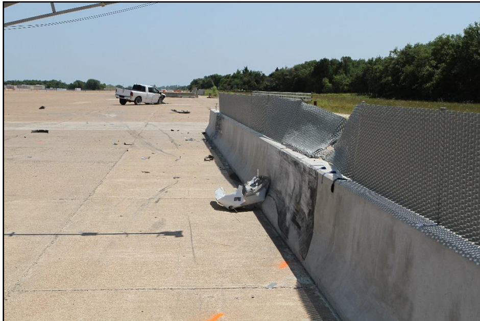
Figure 8.6. Screen-Safe ® Glare Screen on F-Shape Barrier after Test at Impact Location, Test 440822-01-4.
