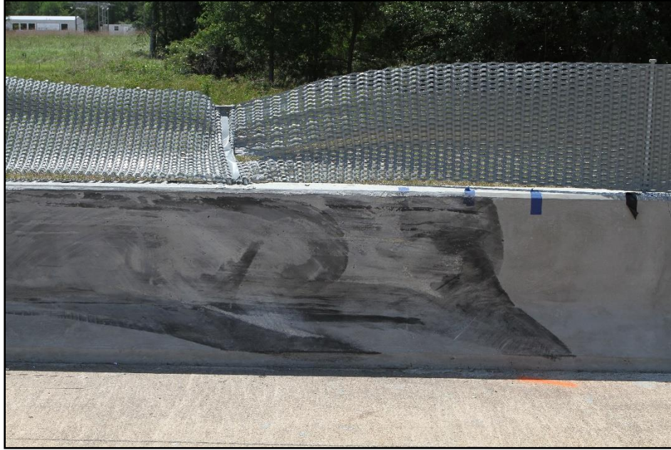
Figure 8.7. Screen-Safe® Glare Screen on F-Shape Barrier after Test at the Joint of Posts 6 and 7, Test 440822-01-4.
