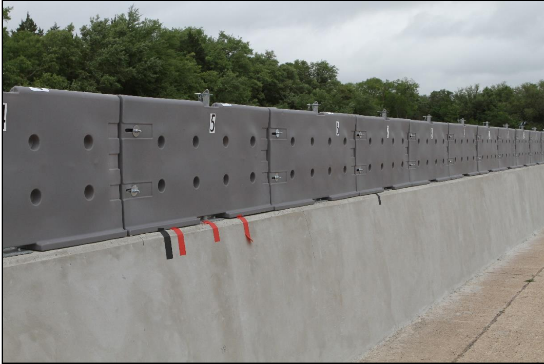
Figure 2.6. Impact Side of Armorcast® Gawk Screen on Single-Slope Barrier prior to Testing.
