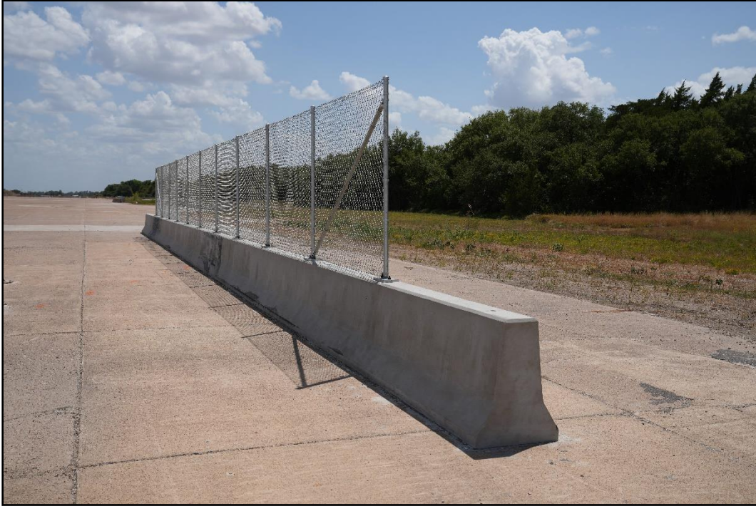
Figure 2.14. Chain-Link Fence on F-Shape Barrier prior to Testing.
