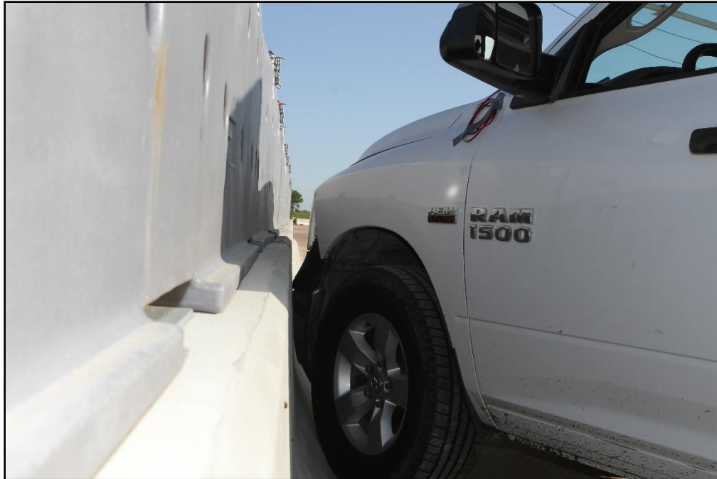
Figure 7.3. Armorcast® Gawk Screen on F-Shape Barrier/Test Vehicle Impact Location, Test 440822-01-3.
