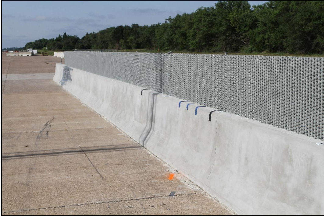
Figure 2.12. Impact Side of Screen-Safe® Glare Screen on F-Shape Barrier prior to Testing.
