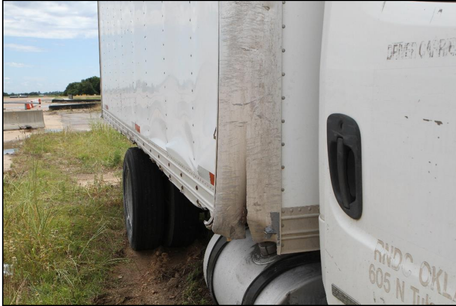
Figure 6.9. Rear Impact Side of Test Vehicle after Test 440822-01-2.
