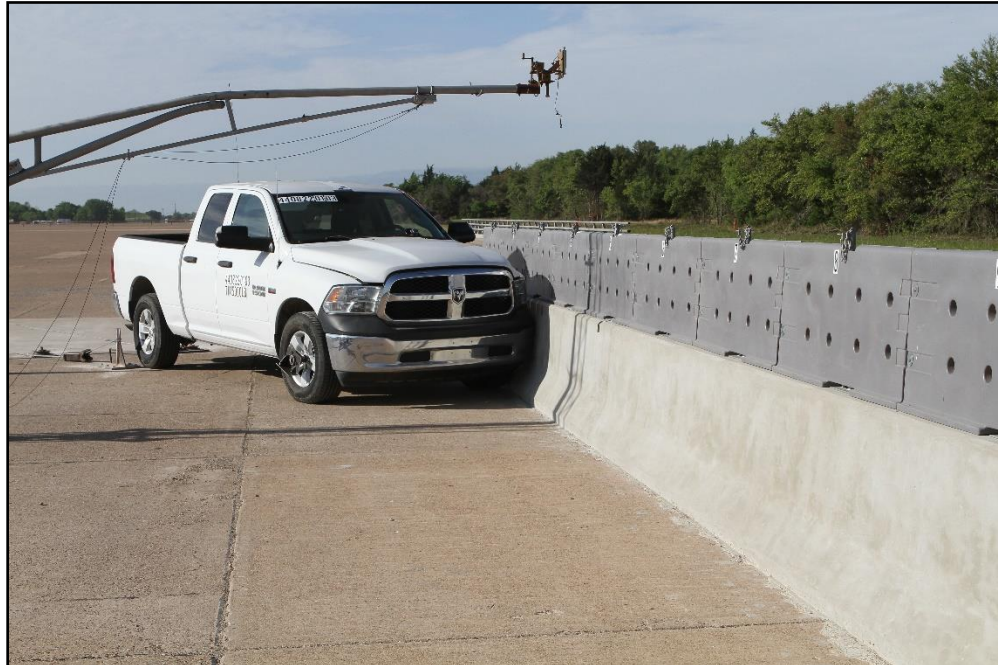
Figure 7.2. Armorcast® Gawk Screen on F-Shape Barrier/Test Vehicle Geometrics for Test 440822-01-3.
