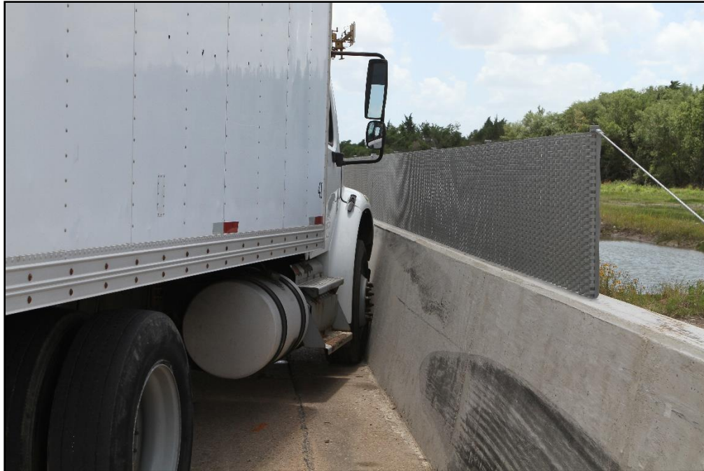
Figure 6.3. Screen-Safe® Glare Screen on Single-Slope Barrier/Test Vehicle Impact Location for Test 440822-01-2.
