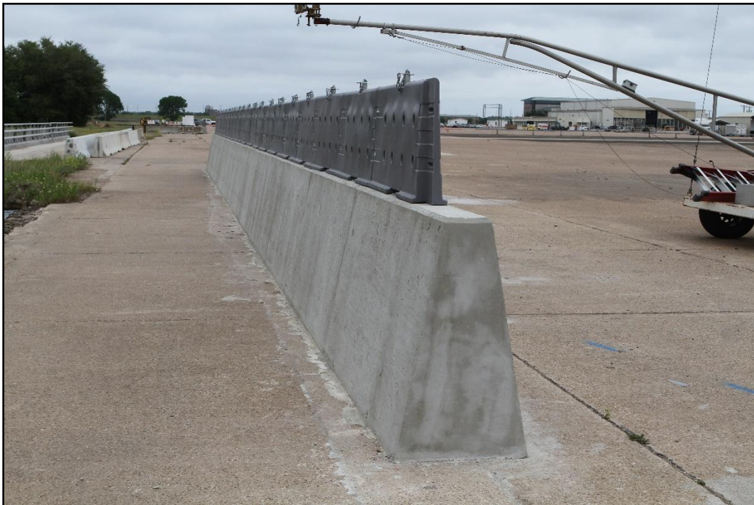
Figure 2.7. Field Side of Armorcast® Gawk Screen on Single-Slope Barrier prior to Testing.
