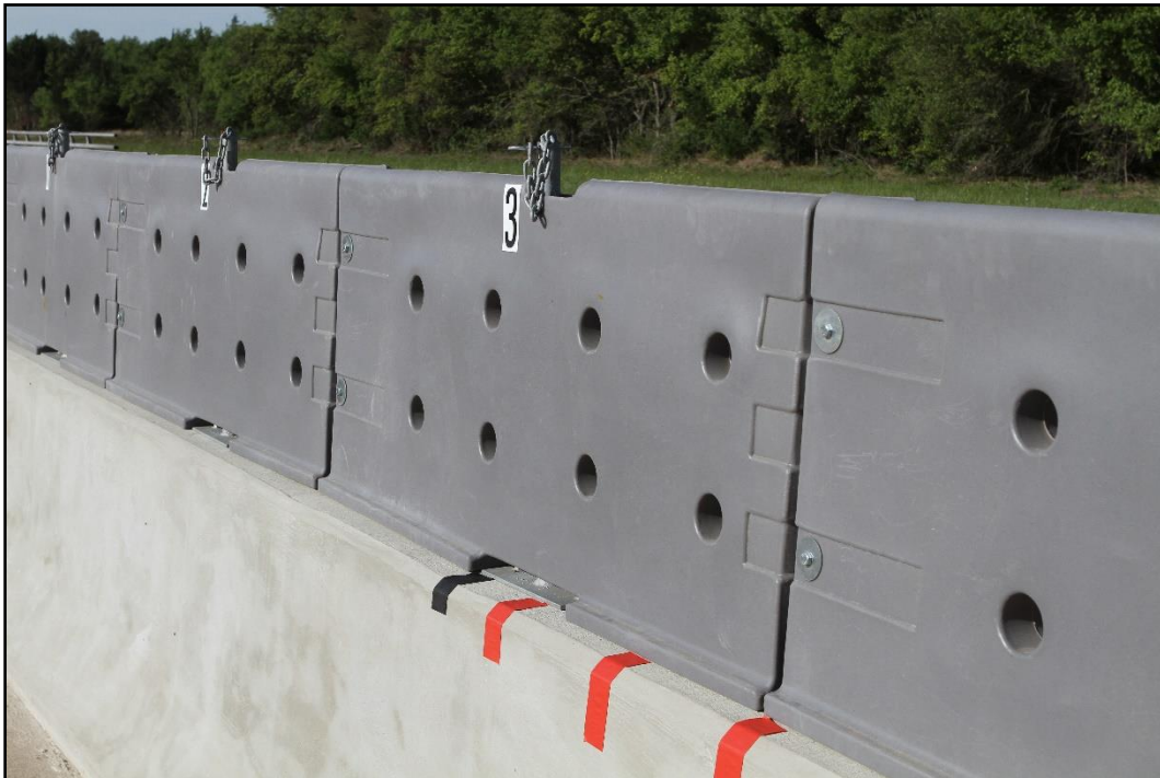
Figure 2.11. Impact Side of Armorcast® Gawk Screen on F-Shape Barrier prior to Testing.
