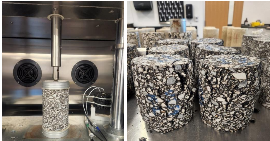
Figure 84. FN Test (Left) and Specimens after Testing (Right).
