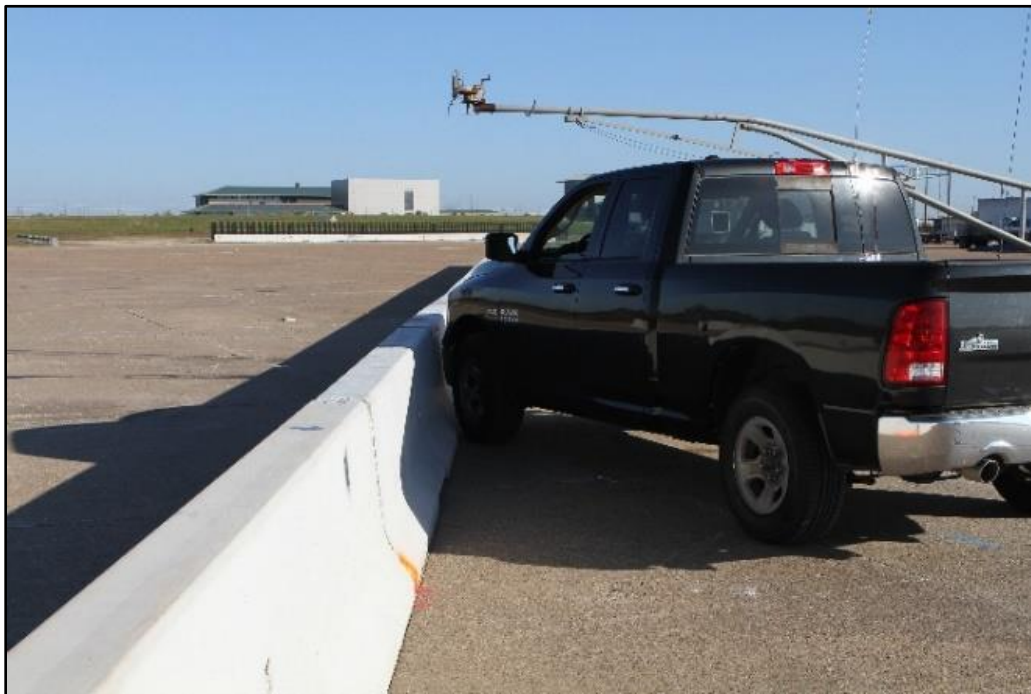
Figure 5.2. Damaged Portable Concrete Barriers/Test Vehicle Geometrics for Test No. 440592-1, Rear View.
