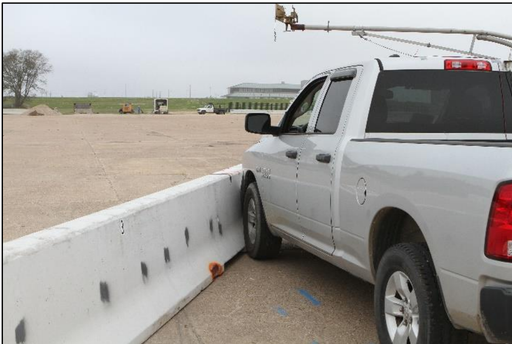
Figure 6.2. Damaged Portable Concrete Barriers/Test Vehicle Geometrics for Test No. 440592-2, Rear View.
