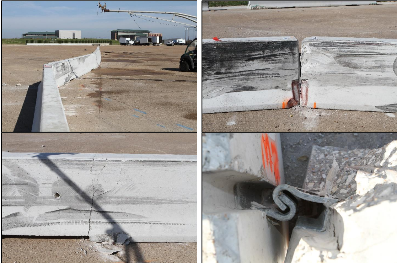
Figure 8.11. Damaged Portable Concrete Barrier after Test No. 440592-2.
