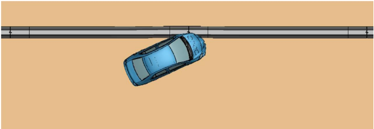
c. t = 0.33 s, event = car redirected by the barrier
