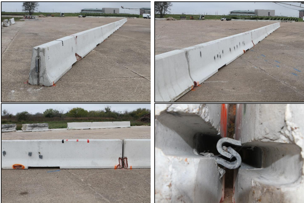
Figure 8.2. Damaged Portable Concrete Barrier before Test No. 440592-2.
