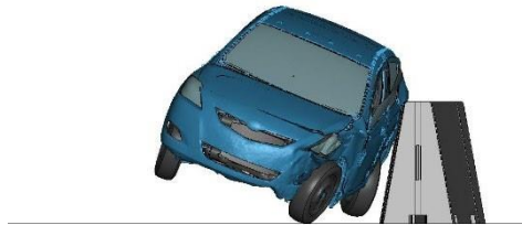
c. t = 0.45 s, event = front right tire touches ground
