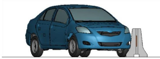
a. t = 0.10 s, event = front right tire contacts the barrier
