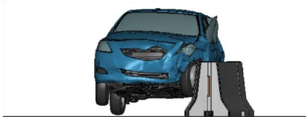
b. t = 0.23 s, event = rear right tire contacts the barrier, window pane snags against the barrier
