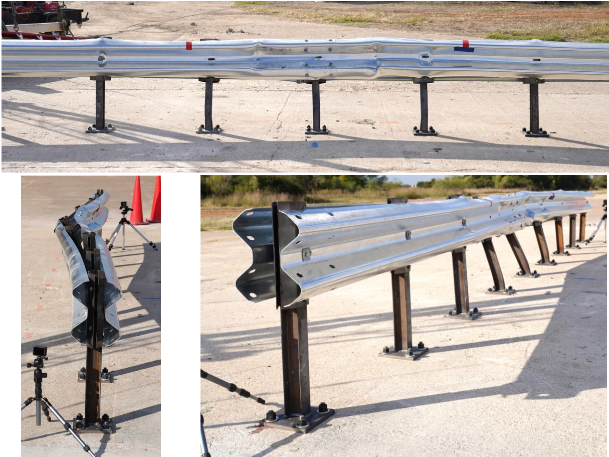
Figure 2.14. Installation after Test 440521-01-B3.
