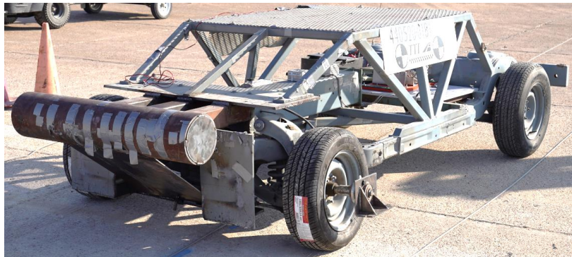
Figure 2.4. Test Bogie Vehicle with Rigidized Pipe Nose.
