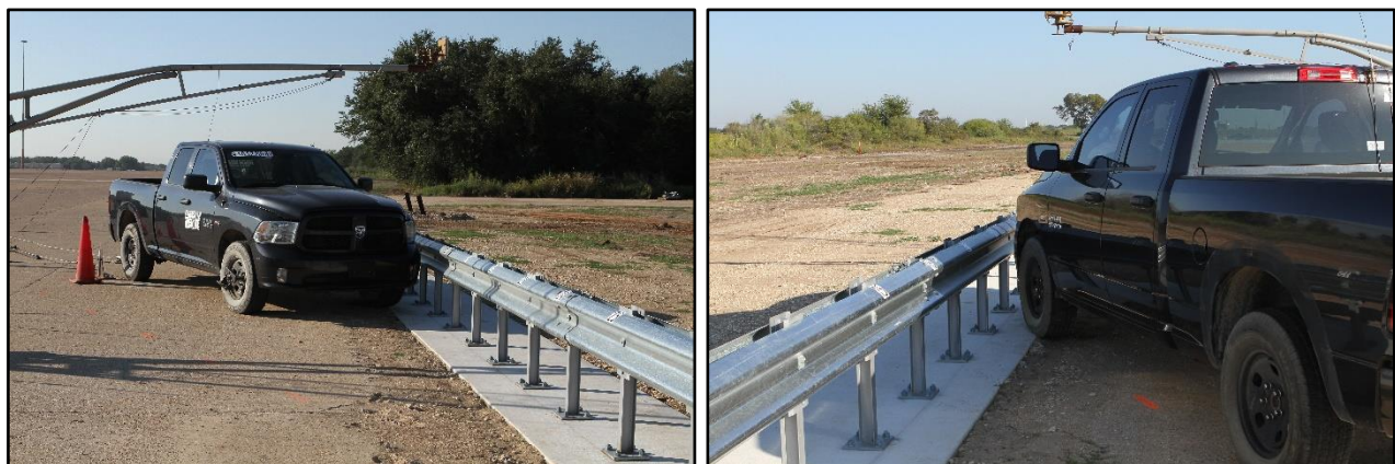
Figure 7.1. Surface-Mounted Median Guardrail/Test Vehicle Geometrics for Test 440522-01-2.
