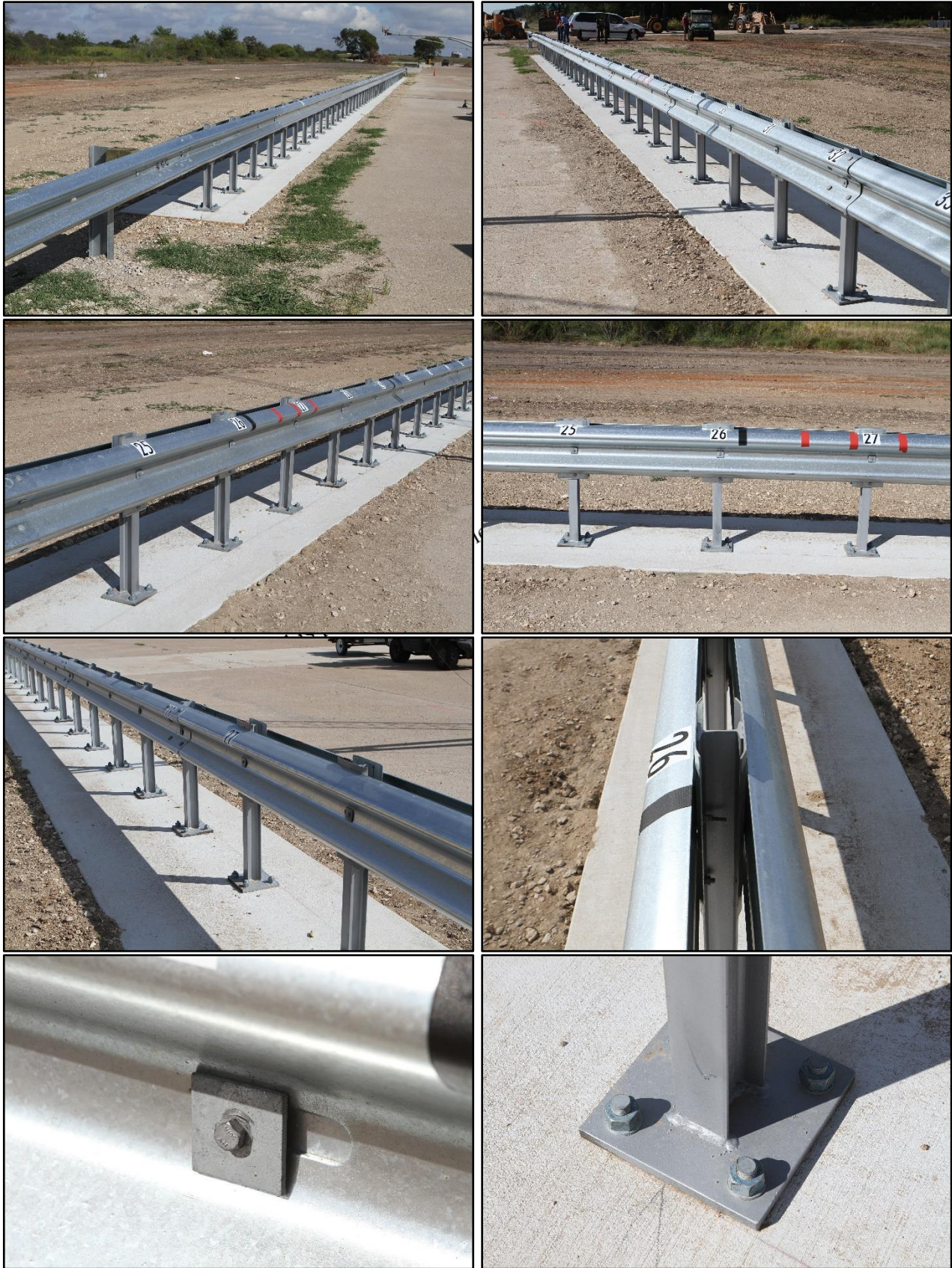
Figure 3.2. Surface- Mounted Median Guardrail prior to Testing.
