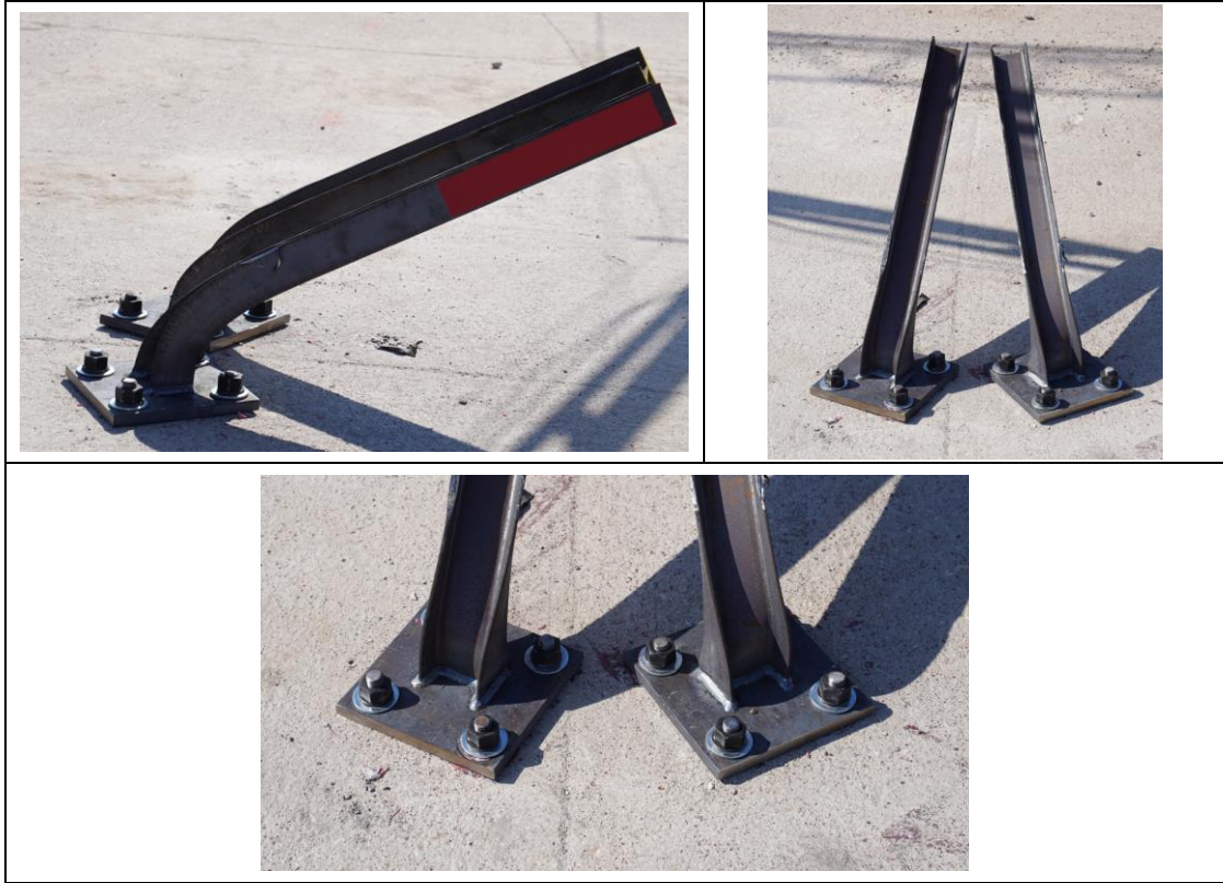
Figure 2.12. Posts after Test 440521-01-B2.
