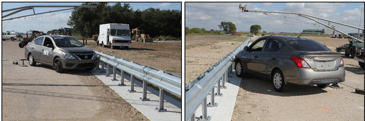
Figure 6.1. Surface-Mounted Median Guardrail/Test Vehicle Geometrics for Test 440522-01-01.
