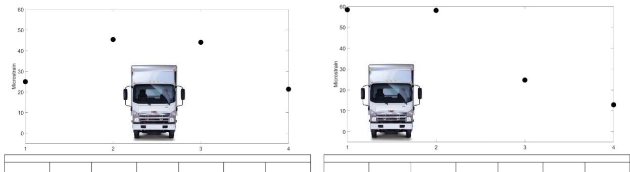
Figure 3.53. Examples of Midspan Strain Lateral Distribution.
