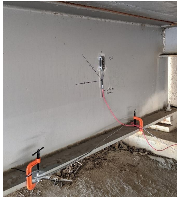
(b) Use C-Clamp for Cable Management
