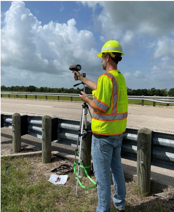
(a) Speed Measurement with a Radar Gun
