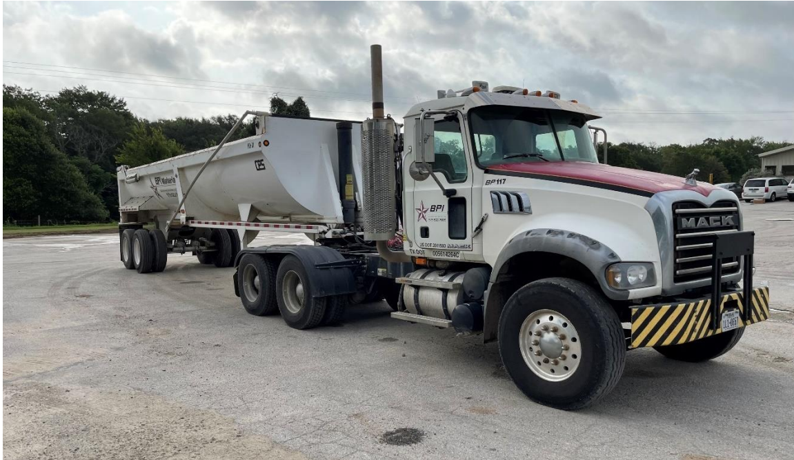
Figure 5.23. Calibration Truck for Bridge #2.
