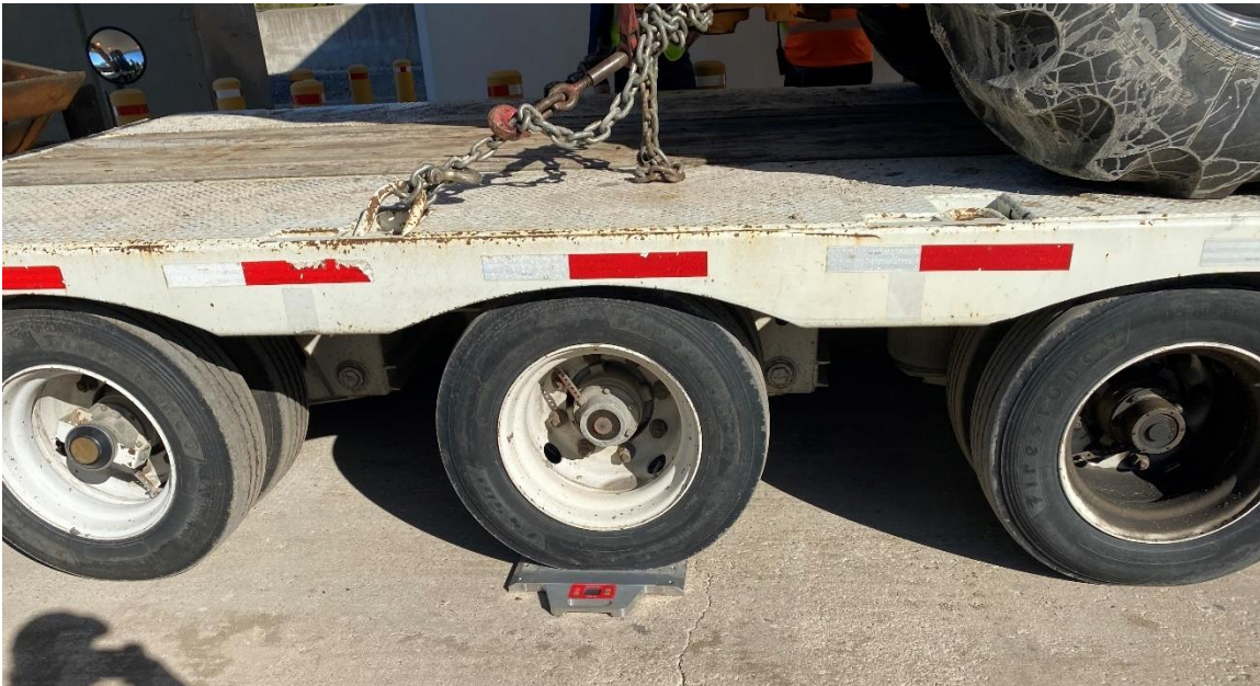
Figure 8.20. Truck Weight Measurement.
