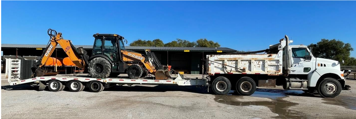
Figure 5.37. Calibration Truck B for Bridge #3.
