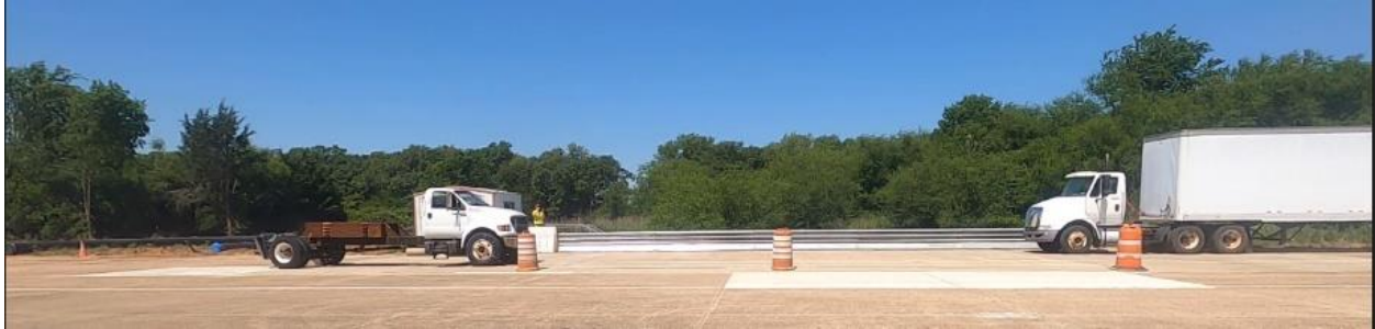
(a) Two Vehicles Entered the RELLIS Bridge from Opposite Directions
