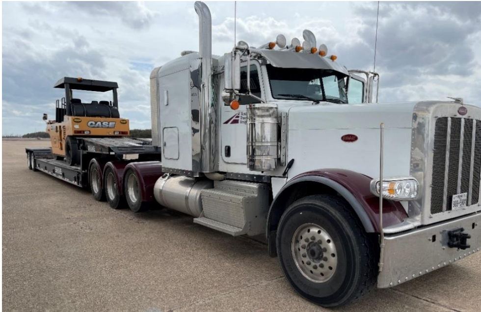
Figure 5.8. TTI Tractor-Trailer Loaded with a Roller Compactor.
