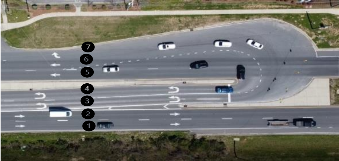
Figure 68. Lane Numbers for the East Side U-turn at Sardis Church Road Site.
