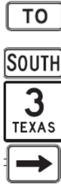
Source: TMUTCD 2014 Edition, Parts from Figure 2D-4 and Figure 2D-6, page 151 and 156. Figure 137. Example of a Trailblazer Route Marker Assembly (59).
