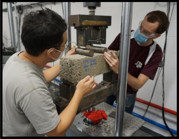
(c) Preparation for MoR Testing
