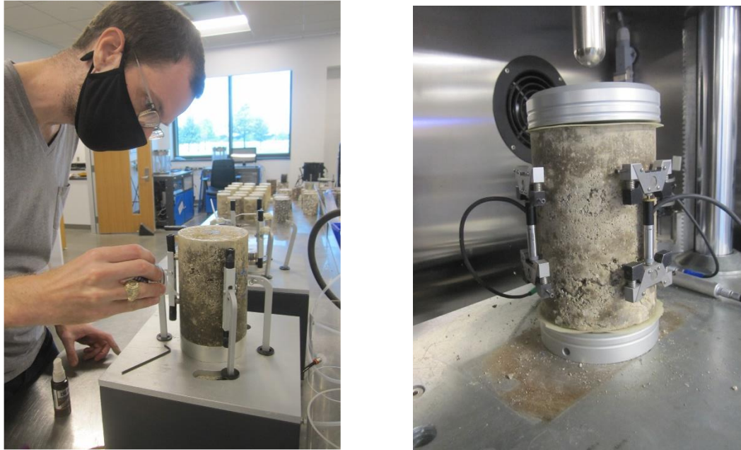
Figure 26. Preparation and Setup for Mr Testing.
