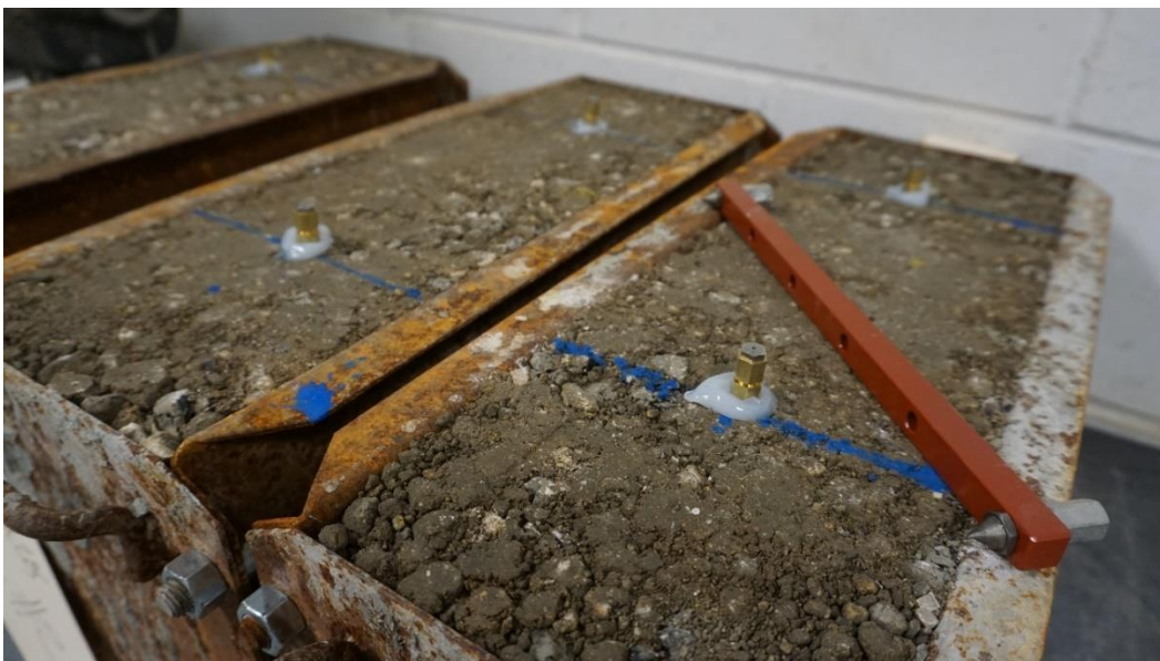
Figure 27. Gauge Studs with Zero Bars for Shrinkage Measurement.
