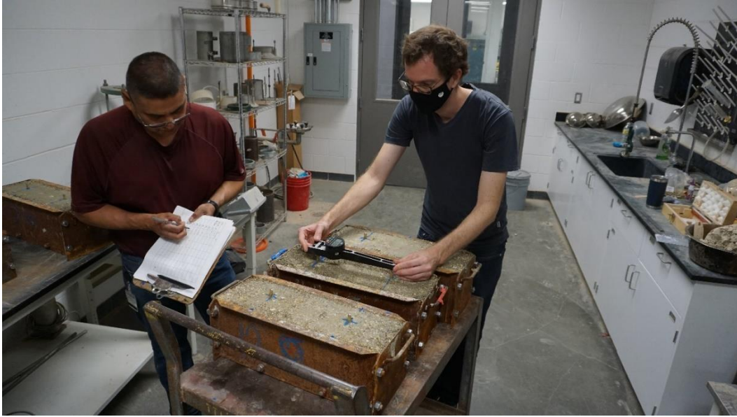
Figure 28. Shrinkage Measurement on MoR Specimens.
