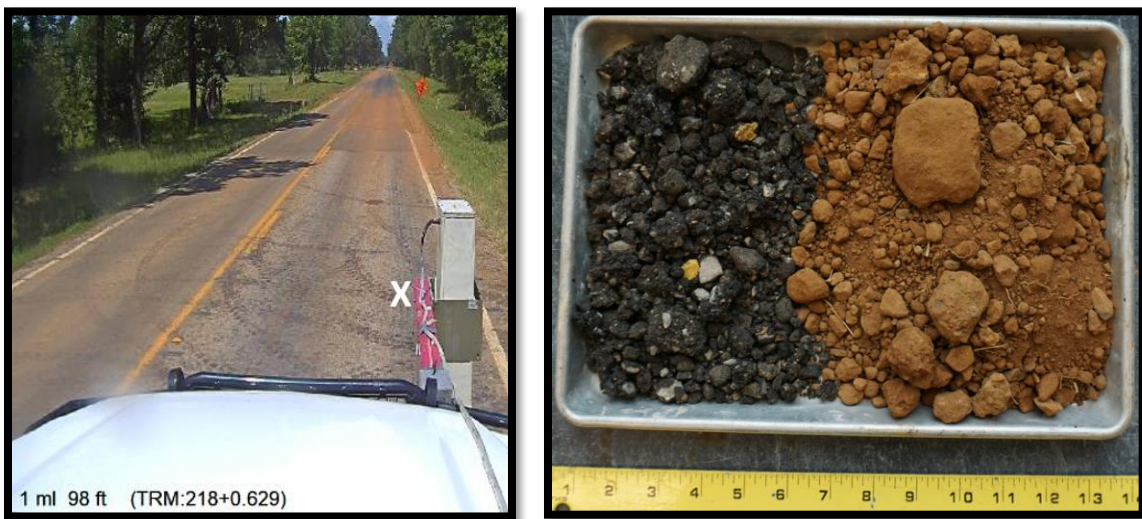
Figure 8. US 259 Roadway Sample Location (Left) and RAP and Salvage Base (Right).
