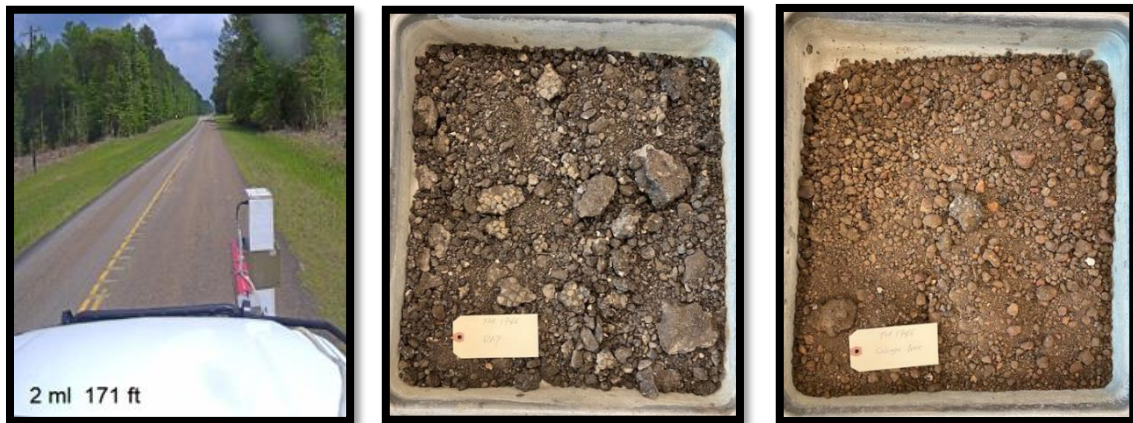
Figure 5. FM 1746 Roadway Sample Location (Left), RAP (Center) and Salvage Flexible Base (Right).
