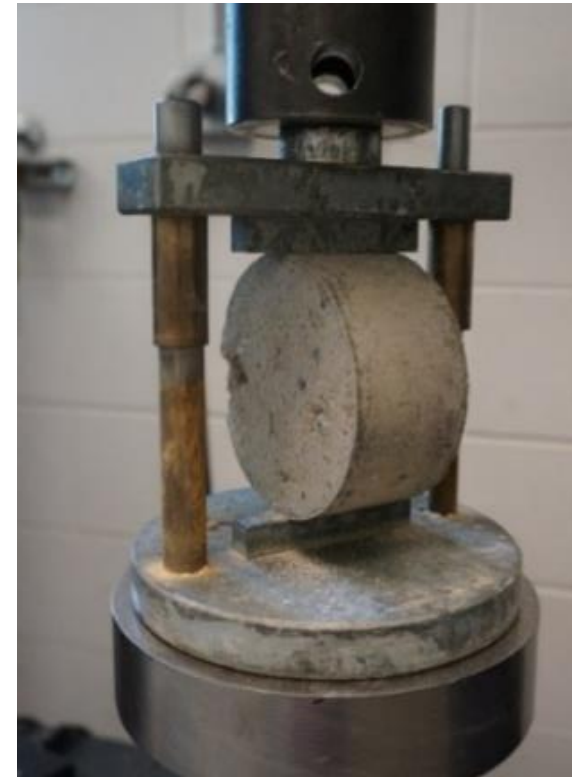
Cement-treated base specimen for rapid mix design
