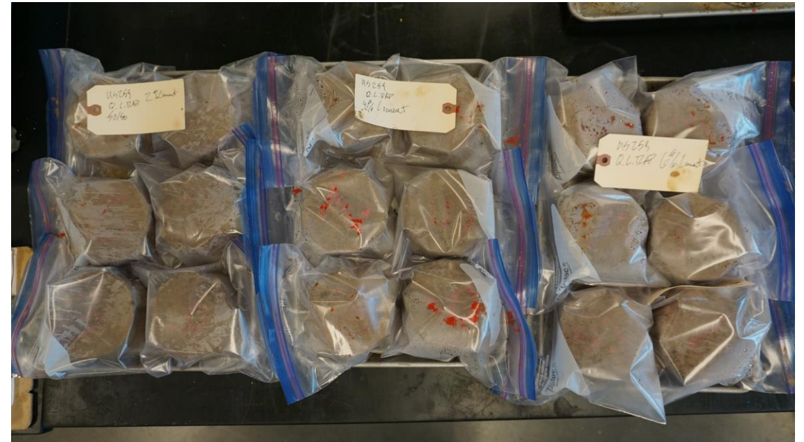
Cement-Treated Specimens Sealed in Zip-Top Bags for Curing during Mixture Design
