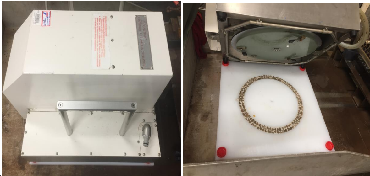
Figure 4-10. DFT on Aggregate Ring—(a) Top View and (b) Side View.
