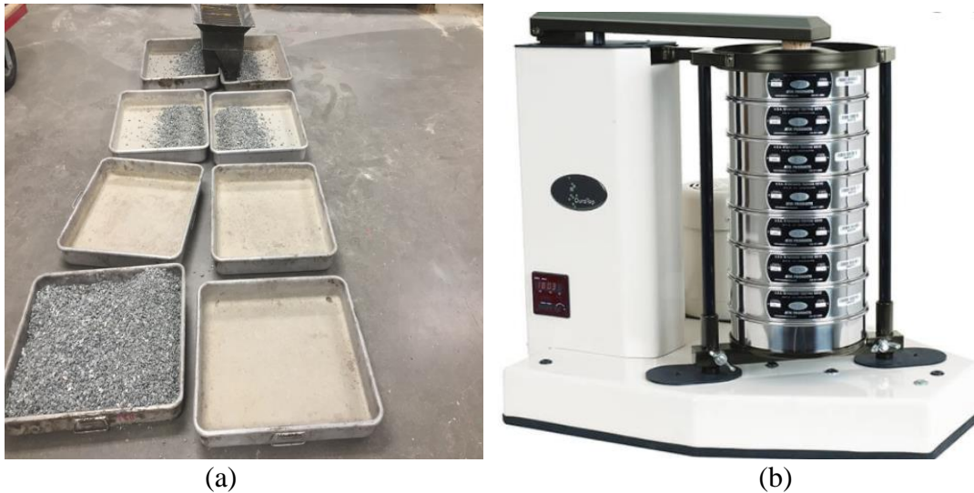
Figure 4-2. Sieve Analysis Test—(a) Sampling and (b) Equipment.
