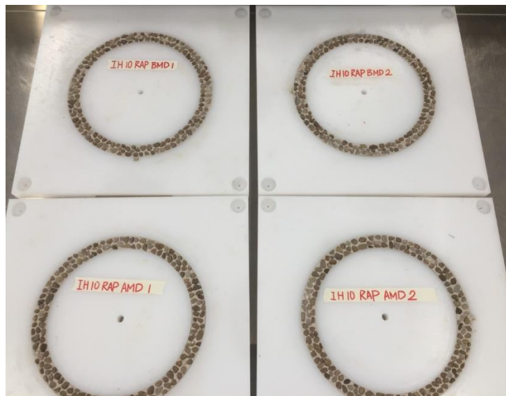
Figure 4-22. IH 10 RAP Aggregate Rings.
