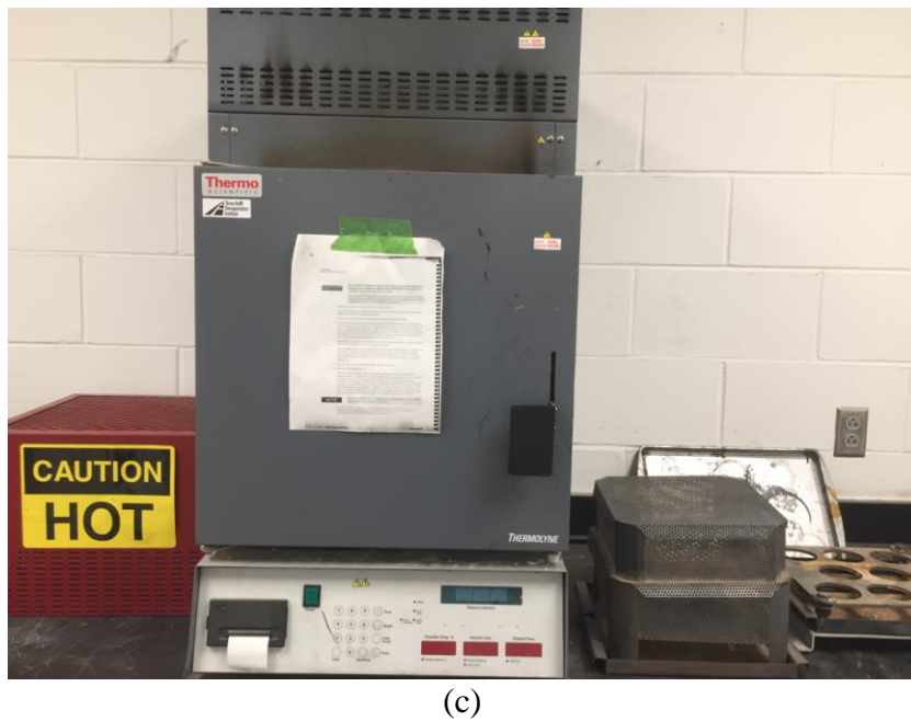
Figure 4-1. Ignition Test—(a) RAP Material Splitting, (b) Sample, and (c) Furnace.
