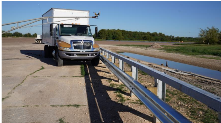
Figure 2. MASH TL-4 Guardrail with 10000S Test Vehicle.
