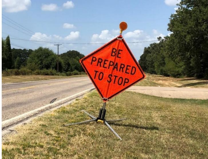
Figure 17. Flashing Warning Light Added to BPTS Sign.
