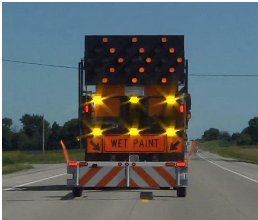
Figure 6. Iowa DOT Truck-Mounted Audible Attenuator System (80).
