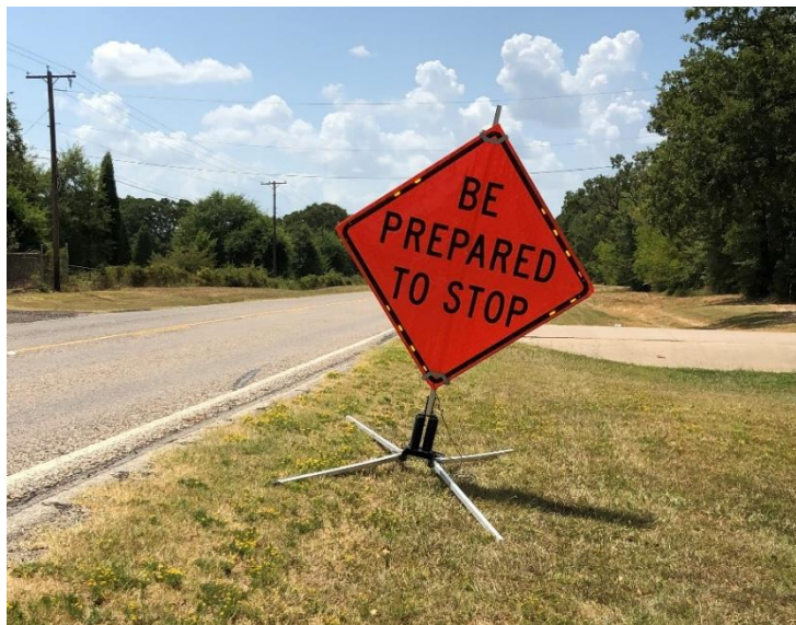
Figure 18. LED Lights Added to the Border of a BPTS Sign.
