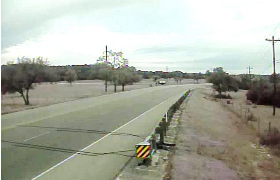
Figure 8. Traffic Counter/Classifier Road Tube Deployment.
