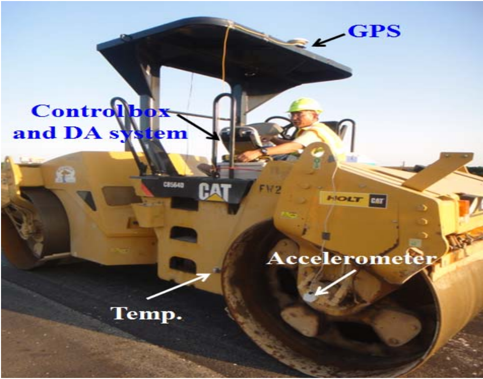
Figure 3. TTI's Complete Compaction Monitoring System.
