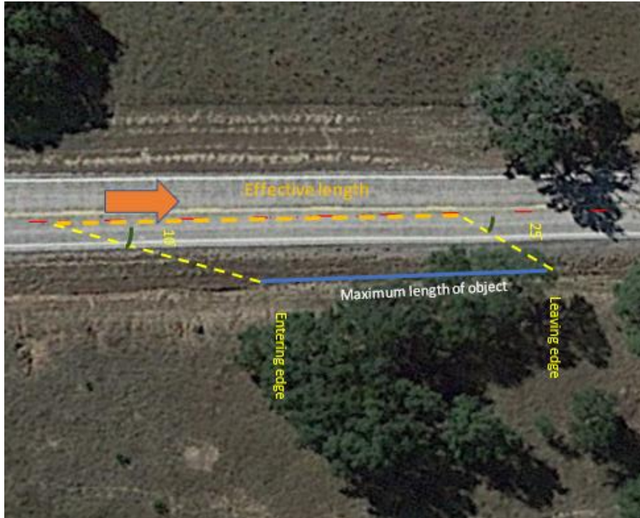
Figure 12. Equivalent Length of Influence Example for a Cluster of Trees.
