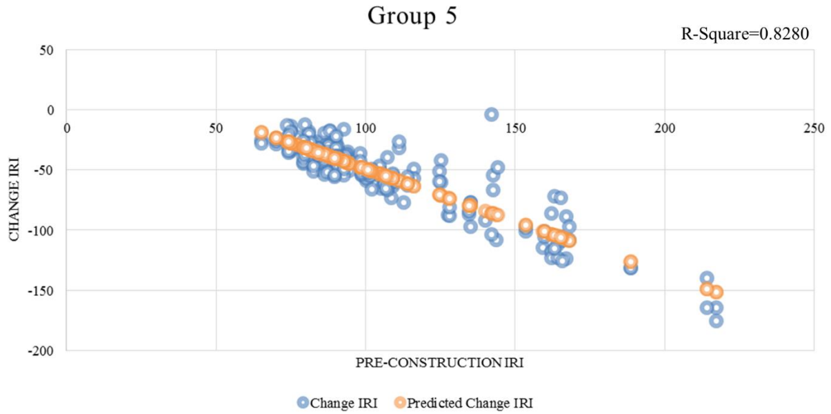
Figure 43. Group 5 Regression Equation Plot (Mill and Overlay Greater than or Equal to 1.5 in.).
