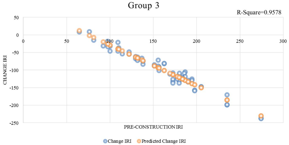
Figure 41. Group 3 Regression Equation Plot (Scarify with Overlay Projects Greater than or Equal to 1.5 in.).
