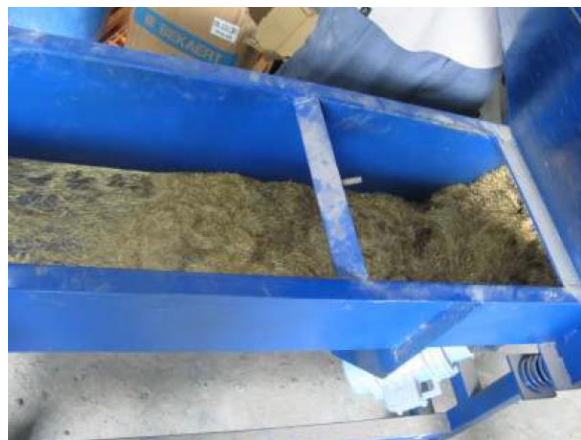
(b) Added fibers into a mixer via a feeder
