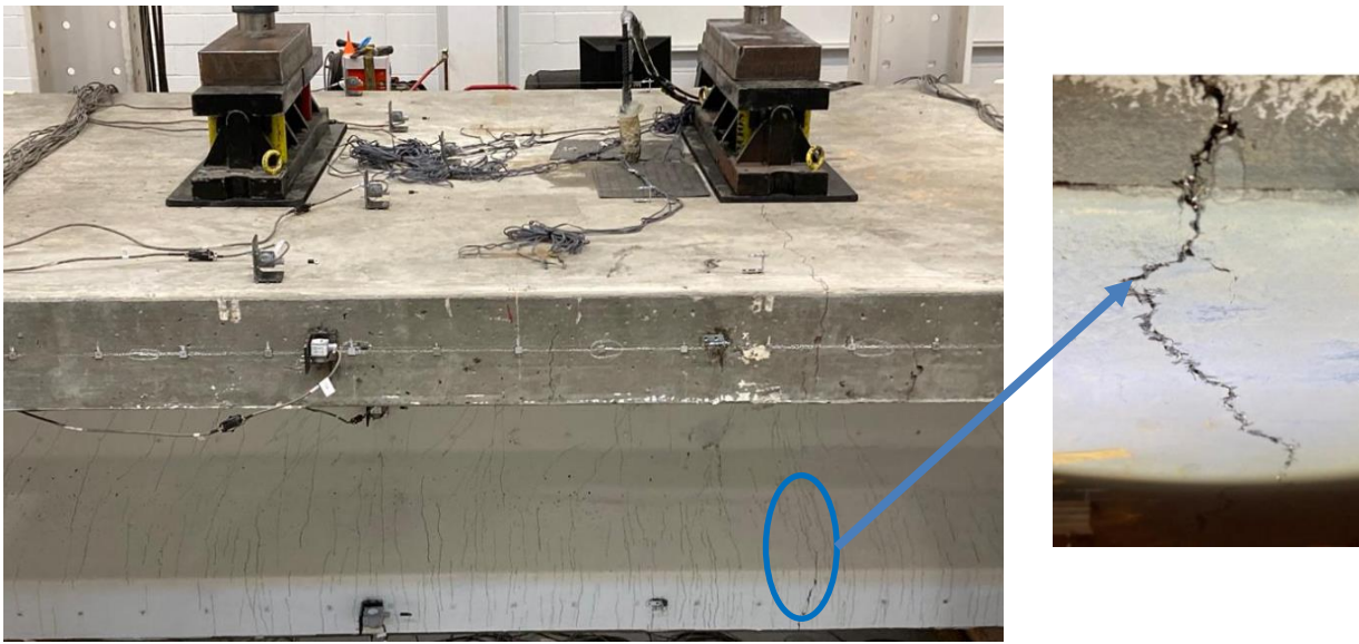
(a) Cracks Formed at Midspan
