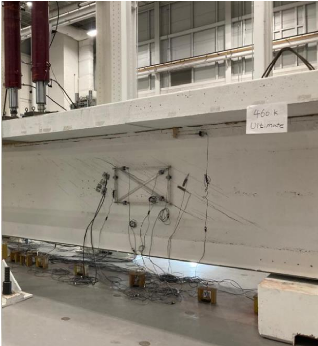
Figure 6.47. Tx54 Shear Test 1: Shear Span of Reinforced End at Failure.
