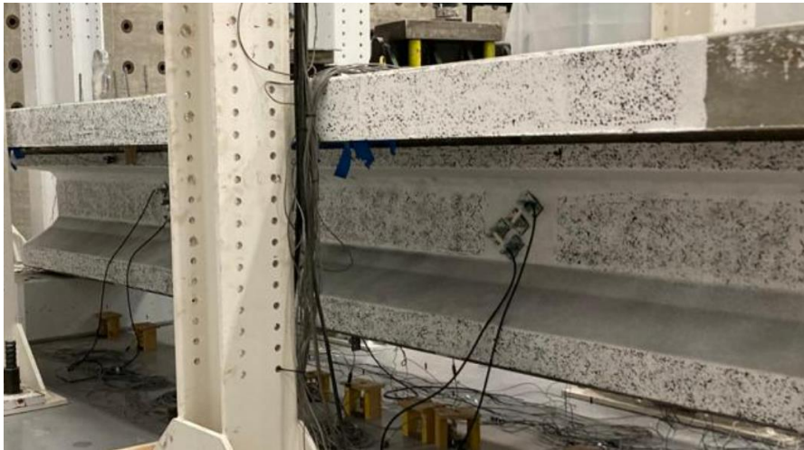
(c) South Face with KSG (Reinforced West End)
