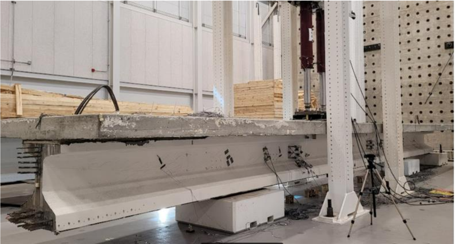
Figure 6.6. Tx34-2 Test Setup and Instrumentation for Shear Test 2 (North Face, Load near the Reinforced End).
