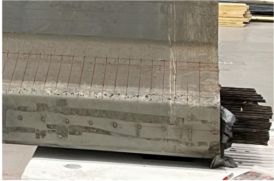
(b) Installed DEMEC Contact Seats
