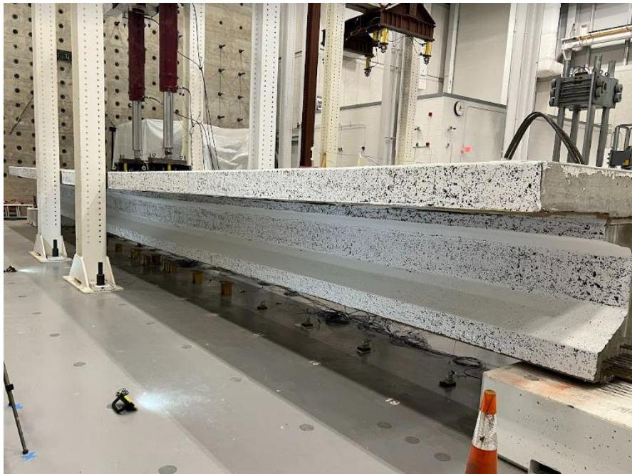
(b) Tx34-2 Test Setup (South Elevation)
