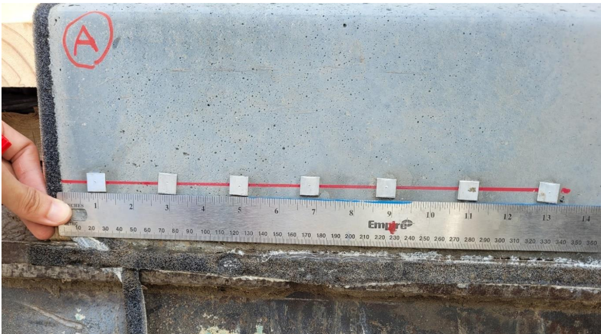
(b) Attached Aluminum DEMEC Points on Tx34-2
