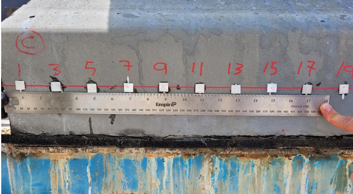
(a) Attached Aluminum DEMEC Points on Tx34-1
