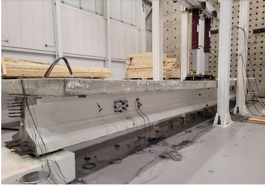
(a) Tx34-2 Test Setup (North Elevation)
