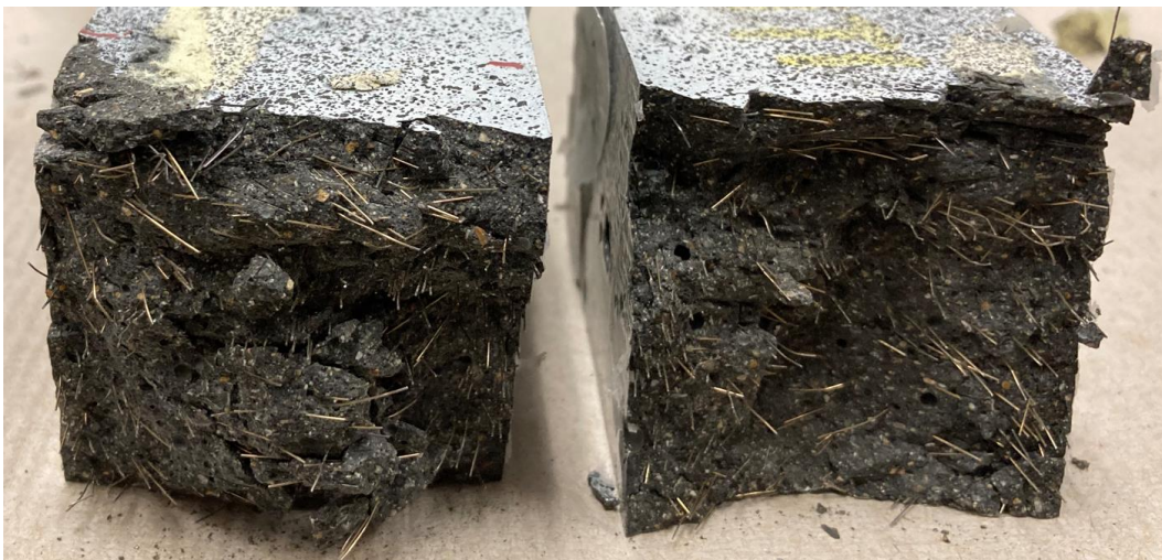
(b) As-Cast Orientation with Improved Fiber Distribution
