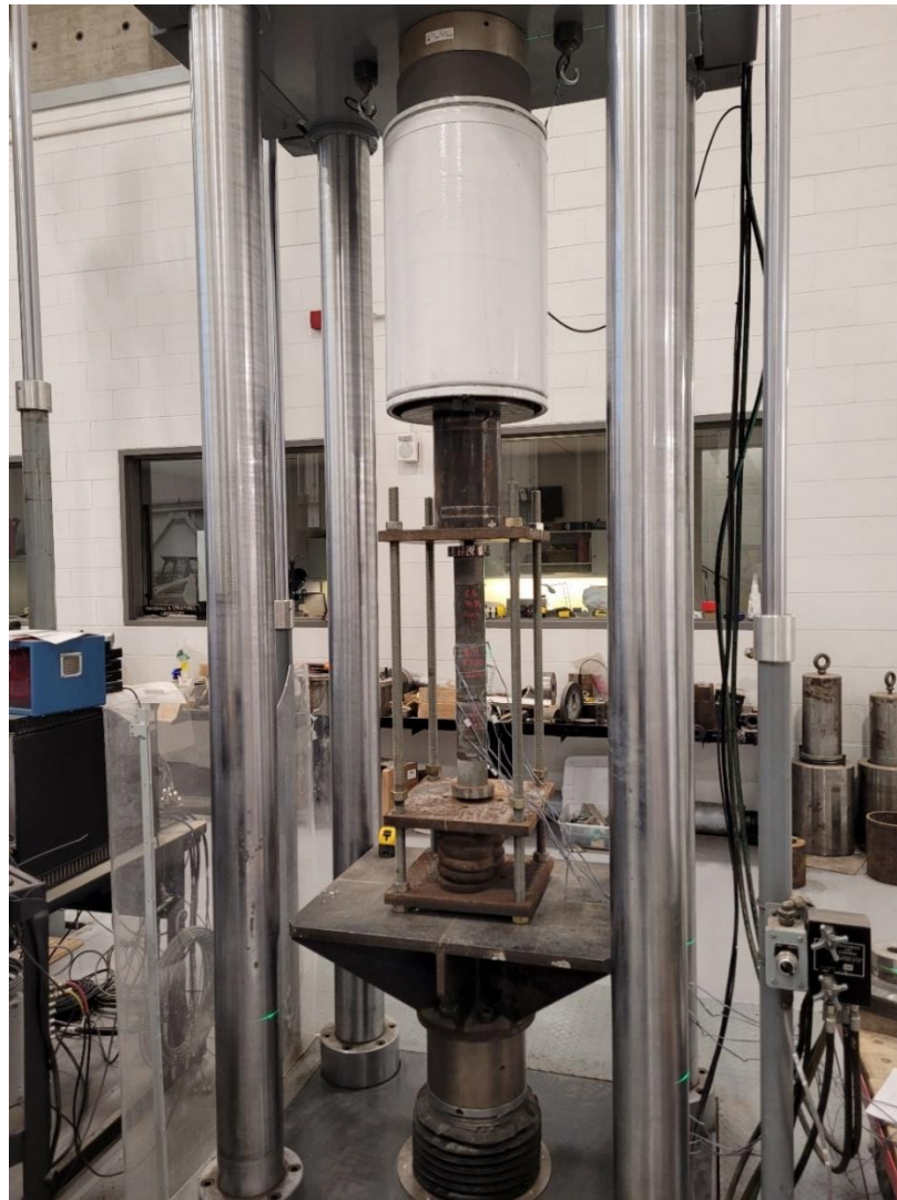
Figure 3.9. Loading a Creep Frame.
