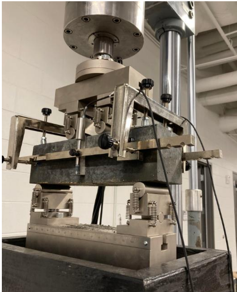
Figure 3.8. Inferred Tension Test Setup.
