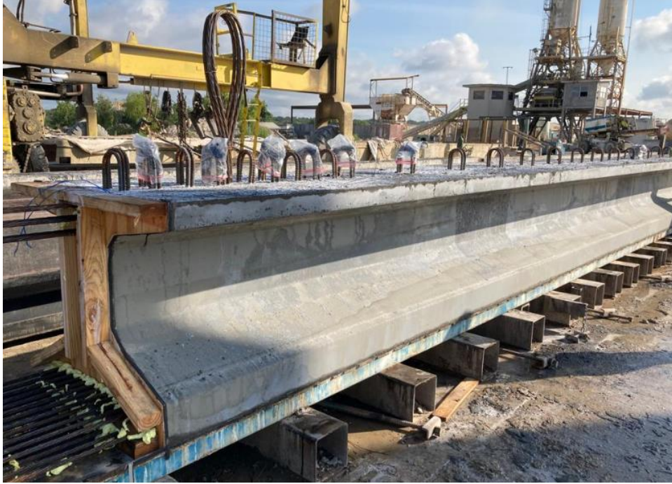
(a) Transition Lines between Batches
