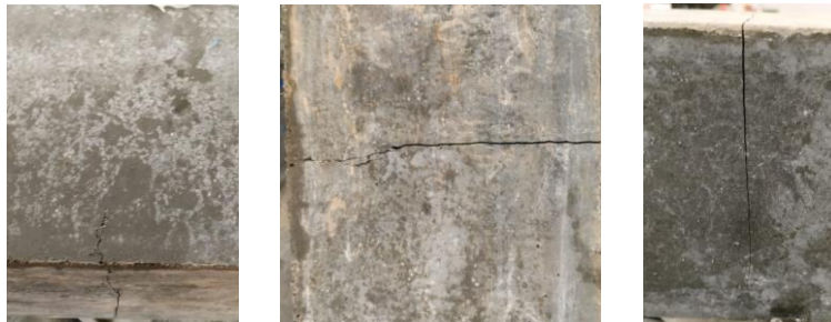
(d) ASTM orientation – left to right: Side face with fibers, bottom tensile face with segregated fibers, Side face with no fibers showing brittle failure
