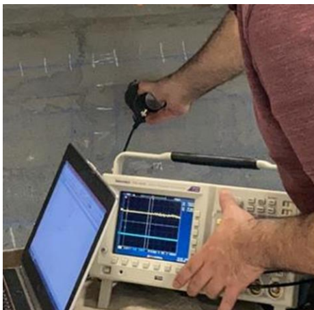
(c) UPV in Progress
