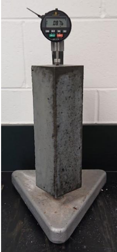
(a) Length Comparator with a Prism
