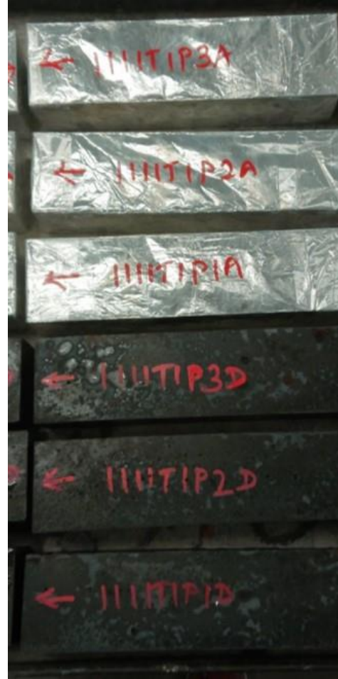
(b) Total Shrinkage and Autogenous Shrinkage Specimens
