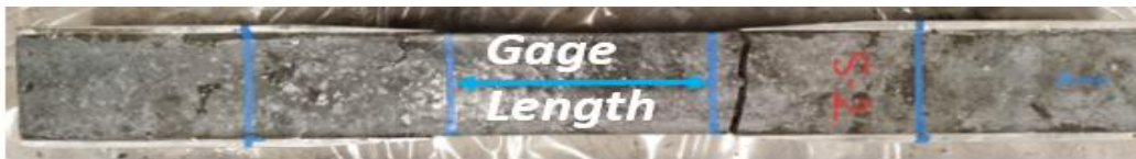
(c) Crack occurring outside the gage length
