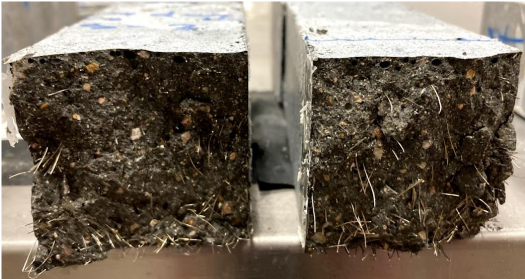
(b) Tx34-2 Tension Specimen—As-Cast Orientation with Improved Fiber Distribution
