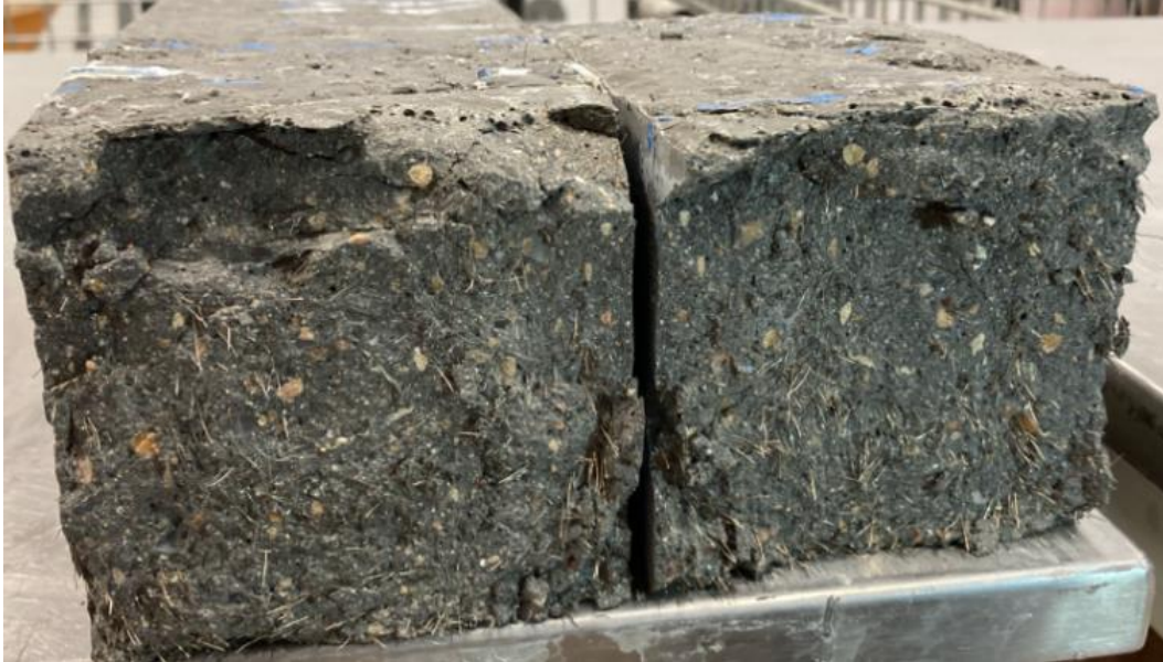
(a) As-Cast Orientation with Improved Fiber Distribution
