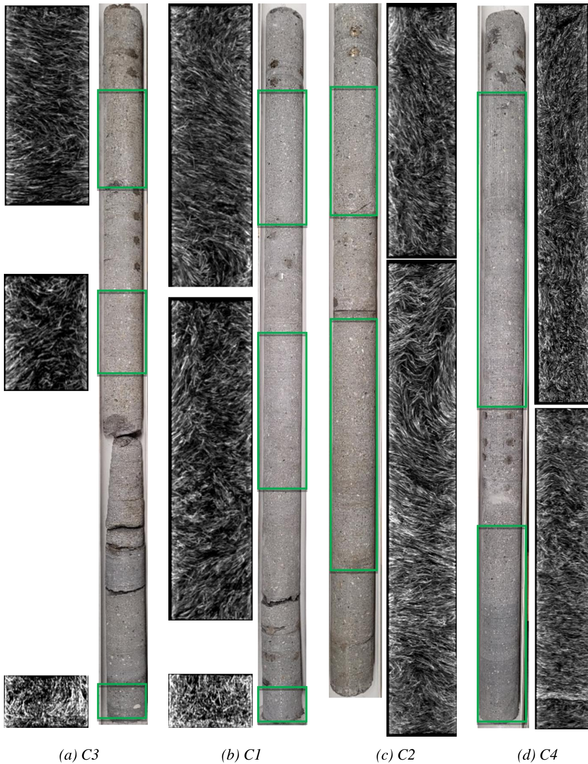
Figure 8.26. Comparison of Fiber Distribution of Tx54 Cores.
