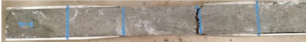
(b) Crack occurring on the gage length
