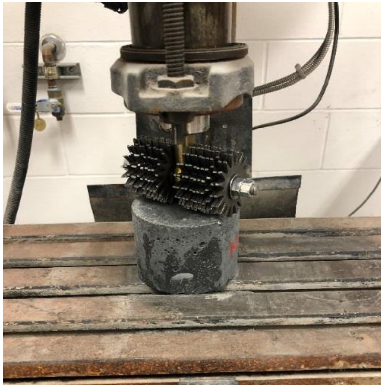
Figure 3.14. Abrasion Resistance Test Setup.
