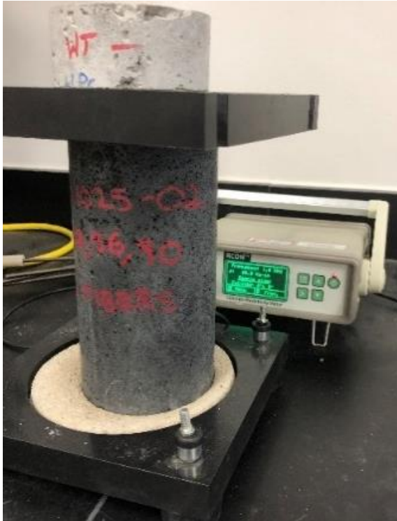
(a) Bulk Resistivity Testing
