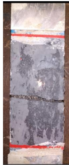
(c) Fibers bridging the crack
