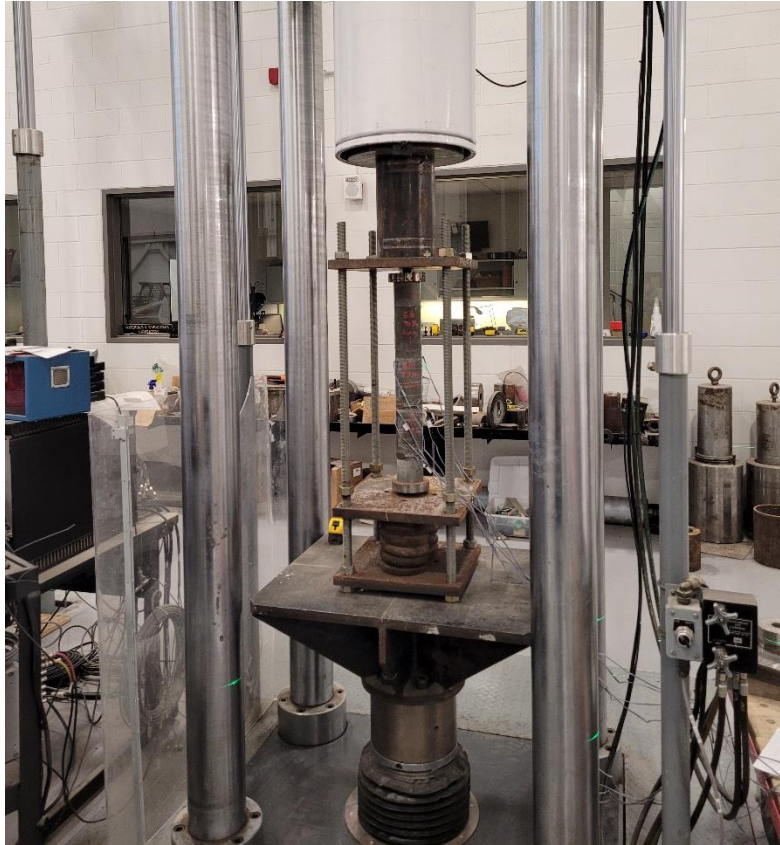
Figure 6.50. Loading a Creep Frame.
