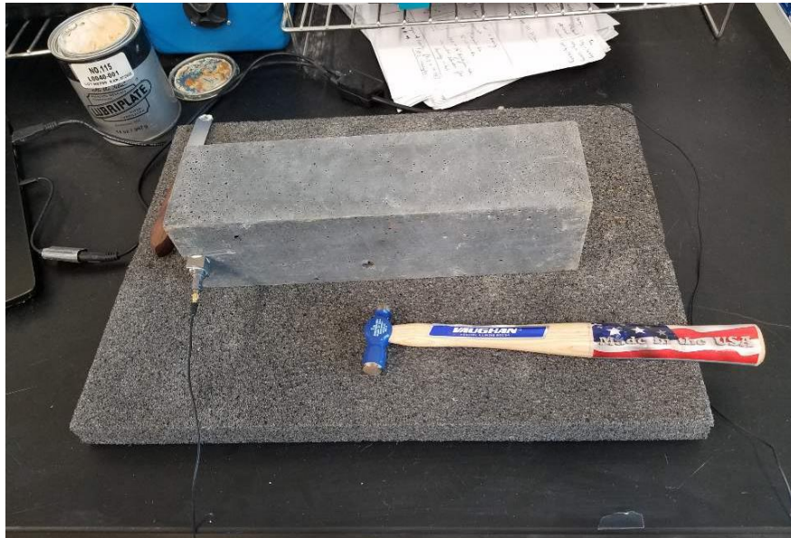
Figure 5.35. Fundamental Transverse Frequency Test Setup.
