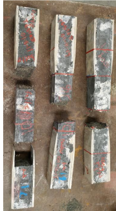
(b) Tested specimens with crack at the grips, within the gage length, and at bottom mounting screw
