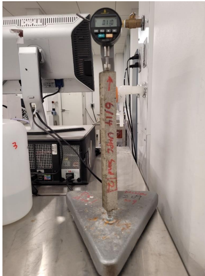
Figure 3.16. Length Change Measurement of ASTM C1260 (2014).
