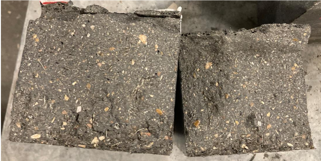
(a) Tx34-2 Flexure Specimen—As-Cast Orientation with Improved Fiber Distribution
