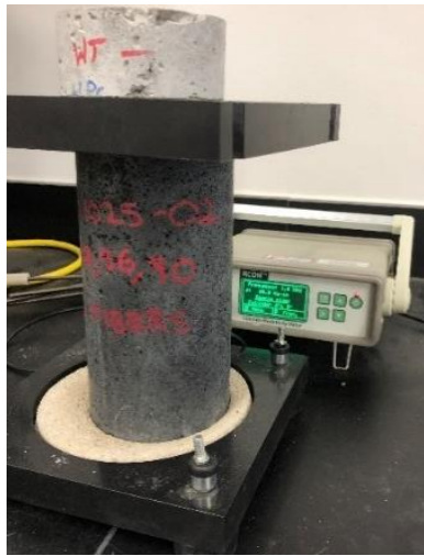
(a) Bulk Resistivity Testing
