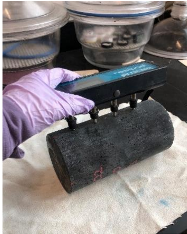
(b) Surface Resistivity Testing
