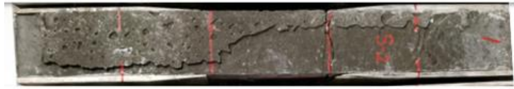
(b) Specimen 02 cracked on mounting screw
