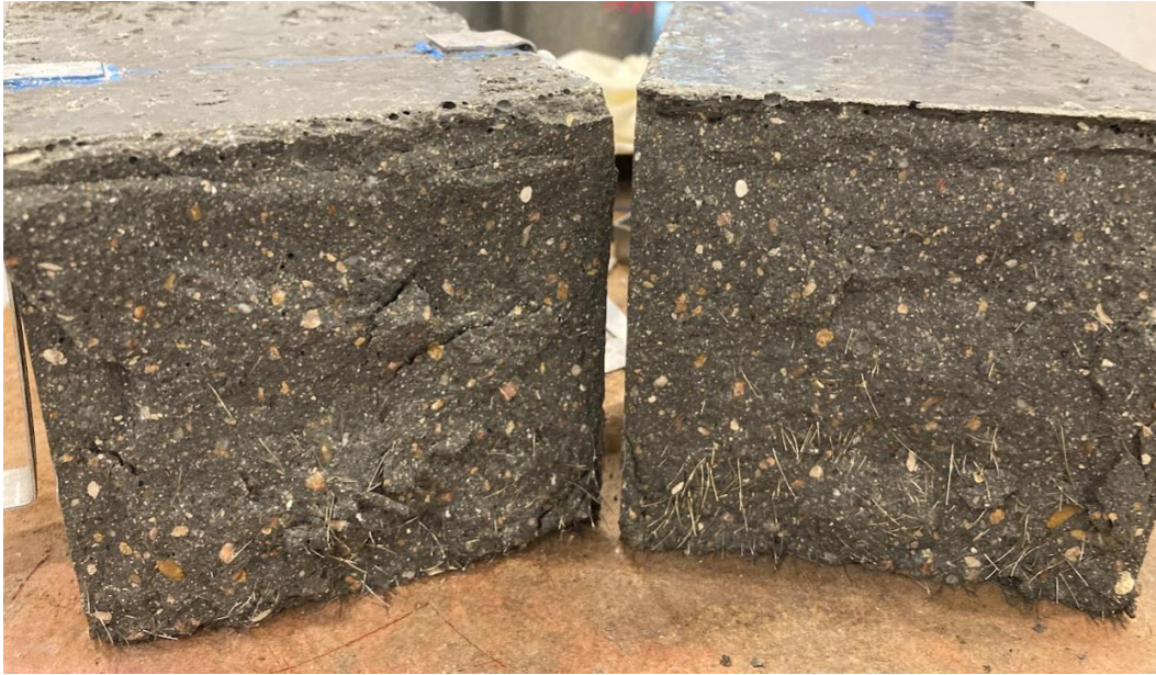
(a) As-Cast Orientation with Fibers Settled to the Bottom
