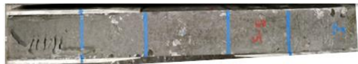
(e) Specimen 05 cracked within the grips
