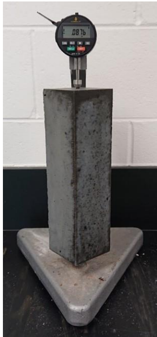
(a) Length Comparator with a Prism
