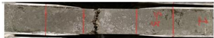
(c) Specimen 03 cracked within the gage length
