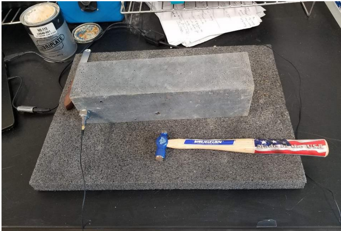
Figure 3.13. Fundamental Transverse Frequency Test Setup.
