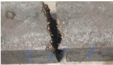
(b) As-cast specimen 05: Bottom tensile crack face
