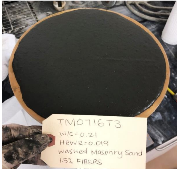
(b) Static flow spread
