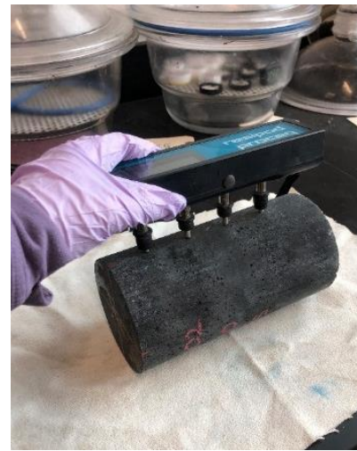
(b) Surface Resistivity Testing
