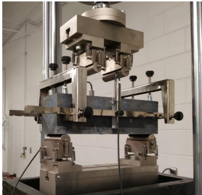
Figure 5.23. Inferred Tension Bending Test Setup.
