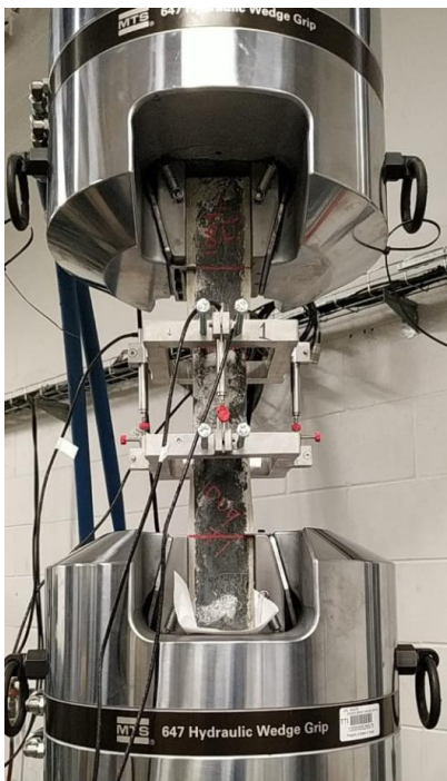
(a) Uniaxial Tensile Test Setup
