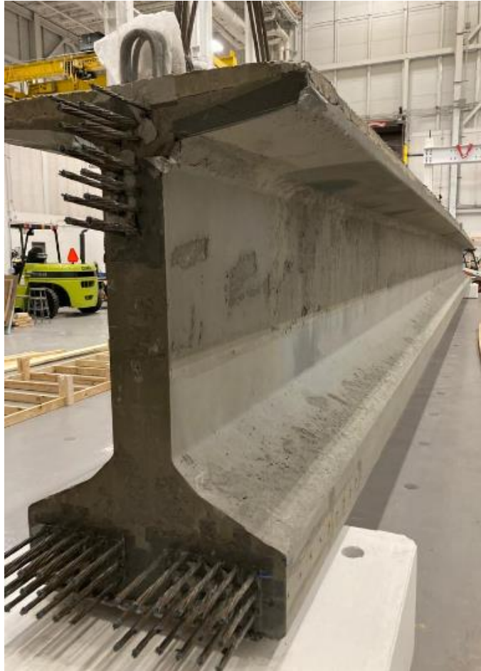
(b) SCC Topping in Top Flange and Surface Texture of UHPC Girder
