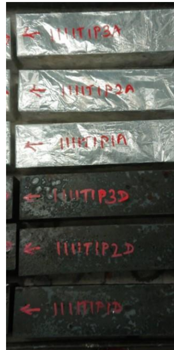
(b) Total Shrinkage and Autogenous Shrinkage Specimens
