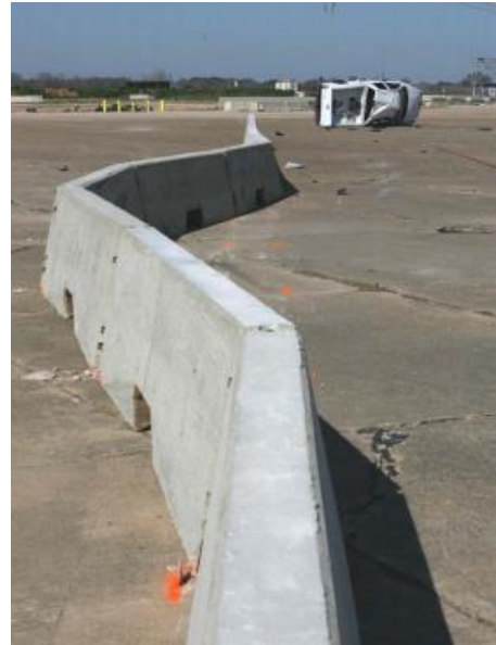
(c) Test Article after Impact
