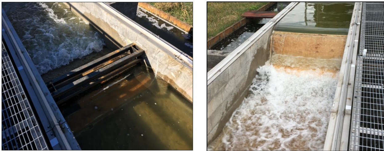
(a) Subcritical flow downstream of steel barrier (b) Supercritical flow downstream of weir barrier
