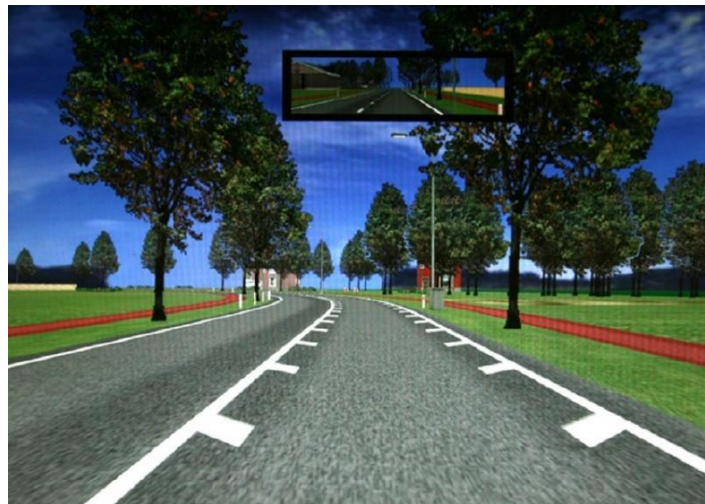
Figure 20. Herringbone-Pattern Optical Speed Bars (23).
