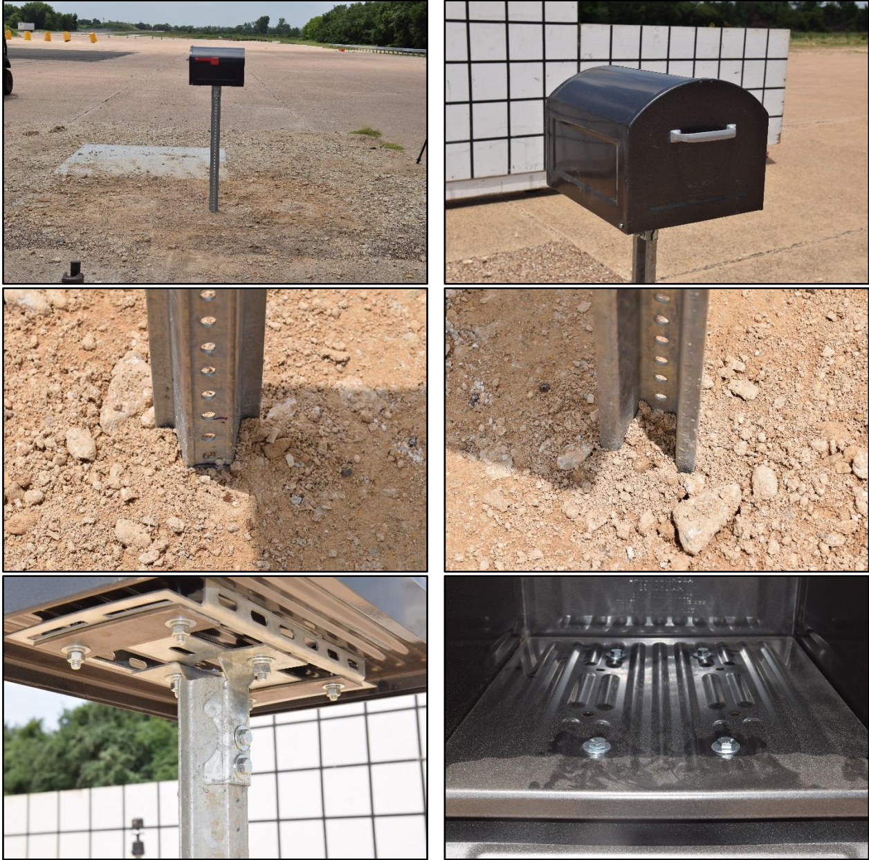
Figure 6.3. Mailbox prior to Test No. 469689-1-3.
