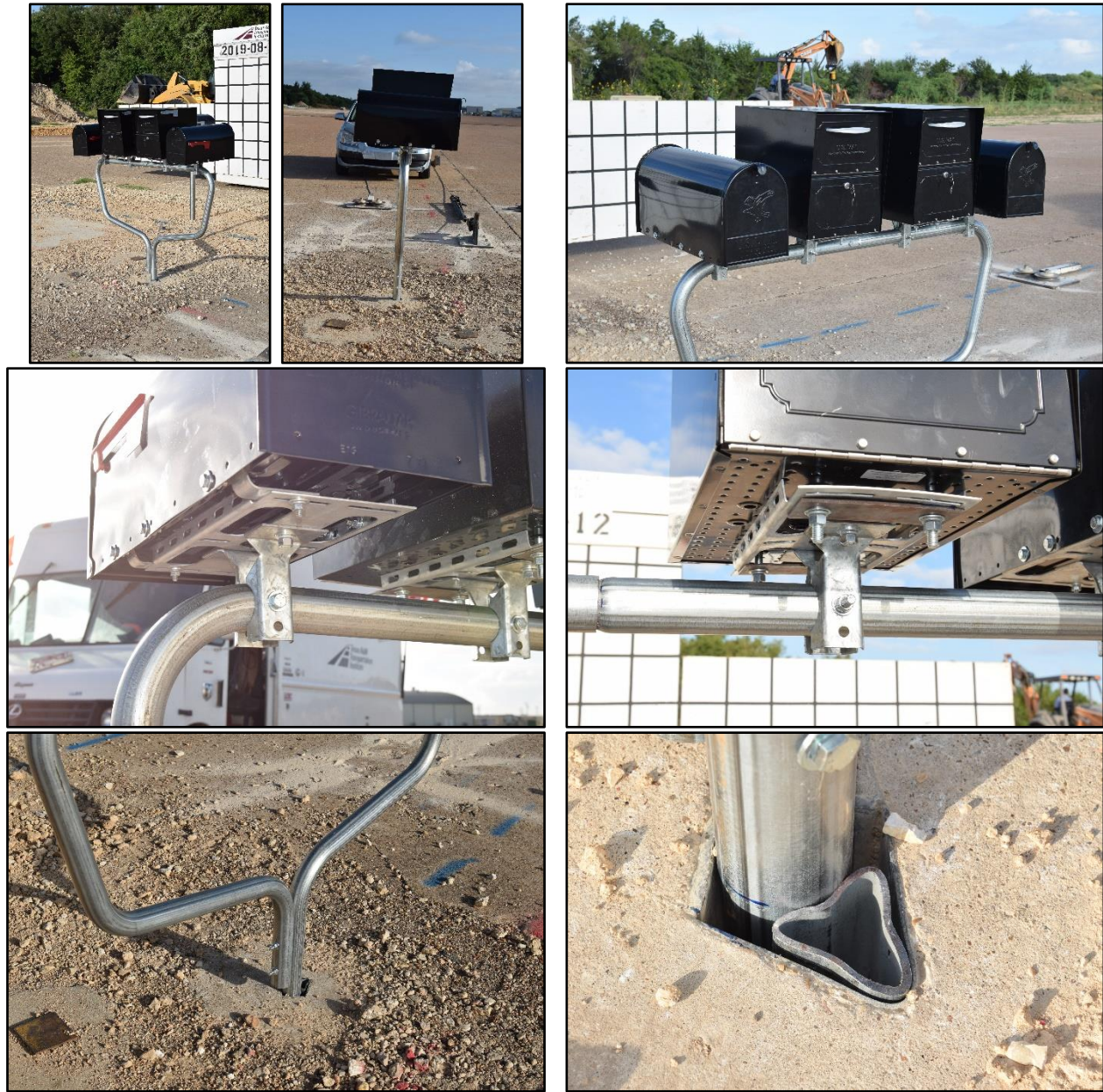
Figure 5.3. Multiple Mailboxes on Bent Pipe Support prior to Testing.
