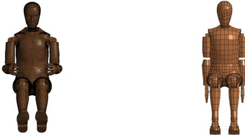
Figure 5.3. Comparison of Mesh Size for Detailed Dummy Model (Left) and Fast Dummy Model (Right).
