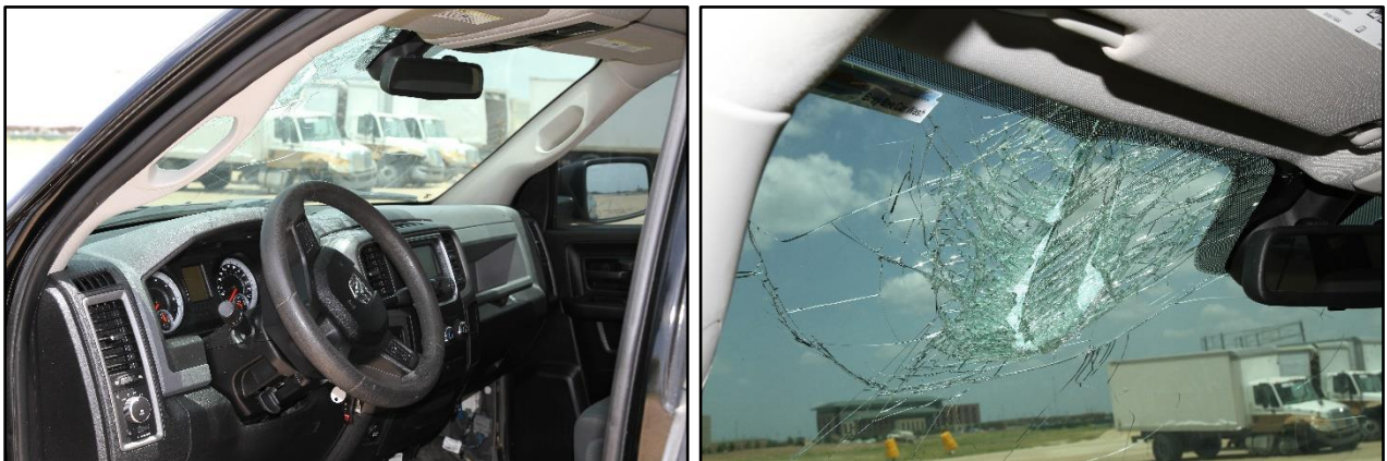
Figure 6.7. Interior of Test Vehicle after Test No. 469680-03-2B.
