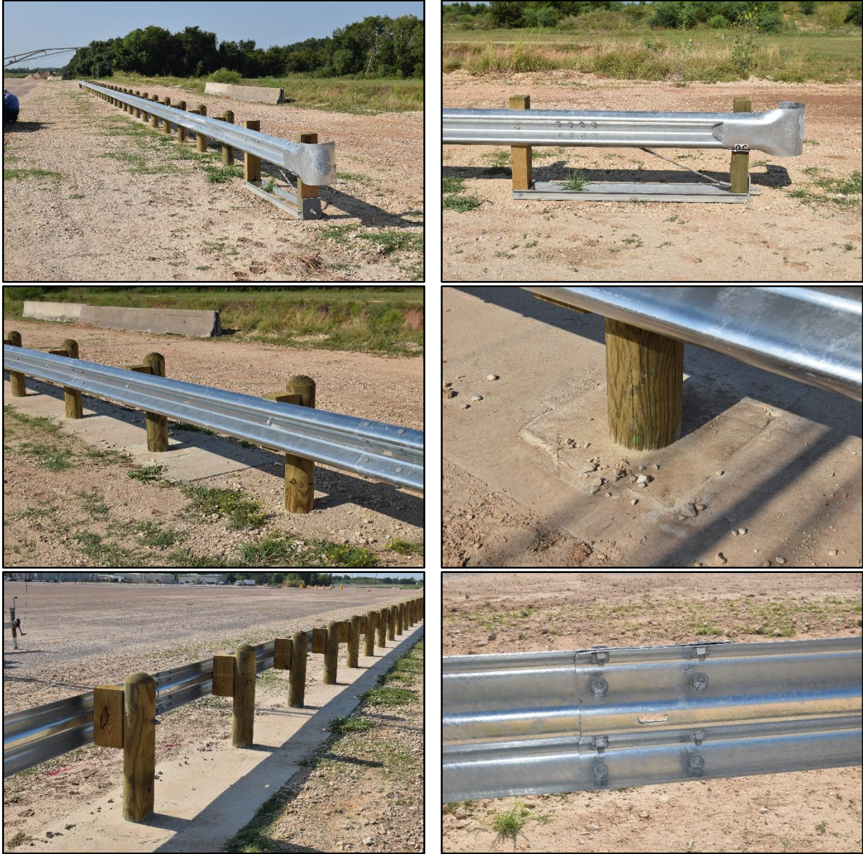
Figure 2.2. TxDOT W-Beam Guardrail with 7½-inch Diameter Round Wood Posts in Concrete Mow Strip prior to Testing.
