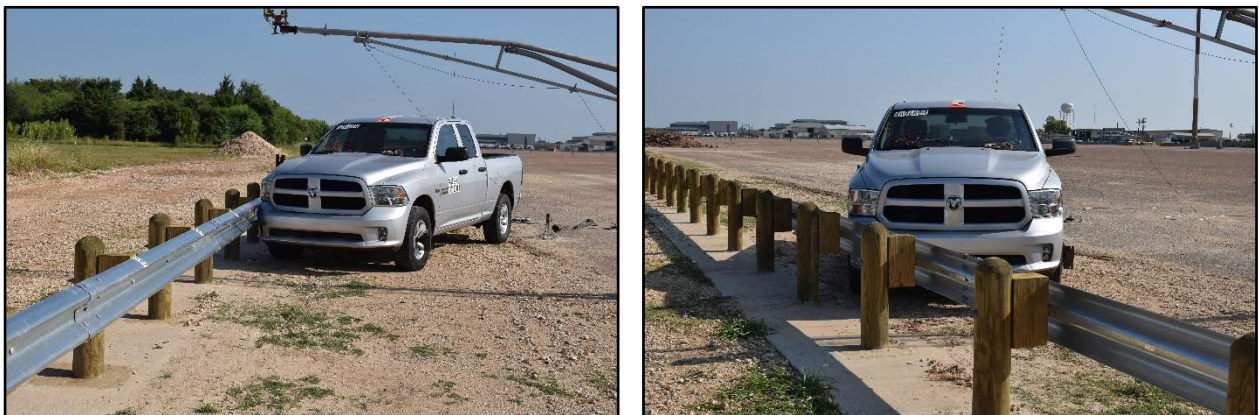
Figure 5.1. Test Installation/Test Vehicle Geometrics for Test No. 469689-4-1.
