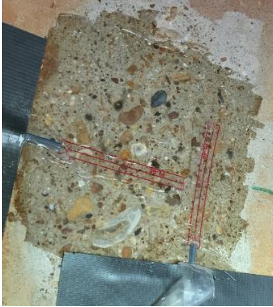
(a) Installed Strain Gauges
