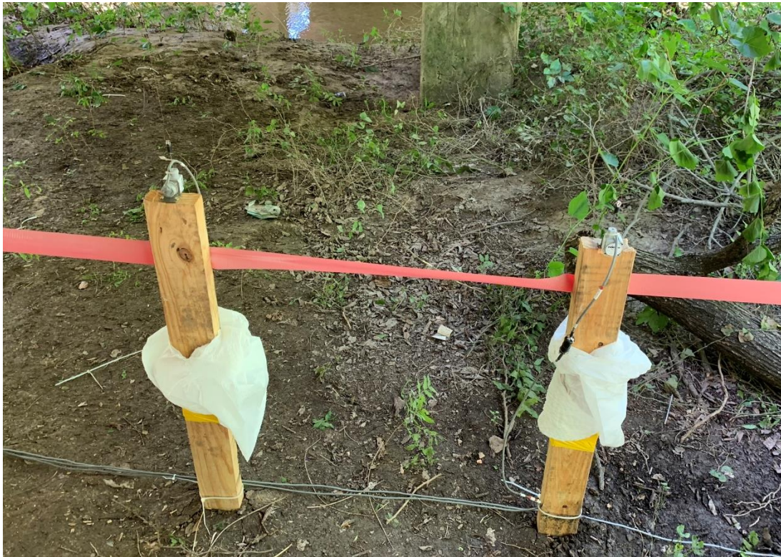
(c) Installed String Potentiometers
