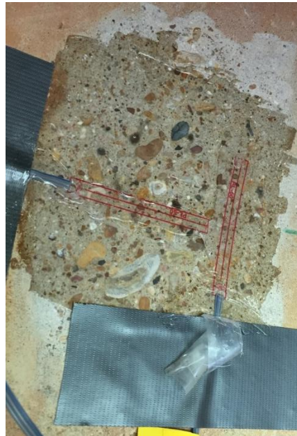
Figure 8.4. Close-Up of Strain Gauge Installation
