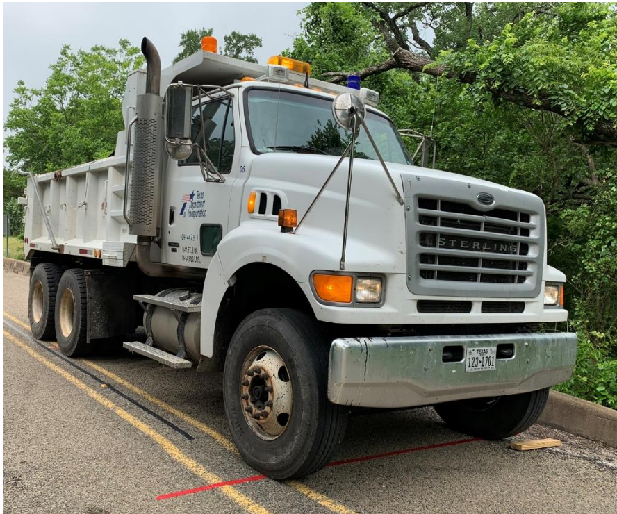
(b) Dump Truck Positioned for Static Test along Path 2
