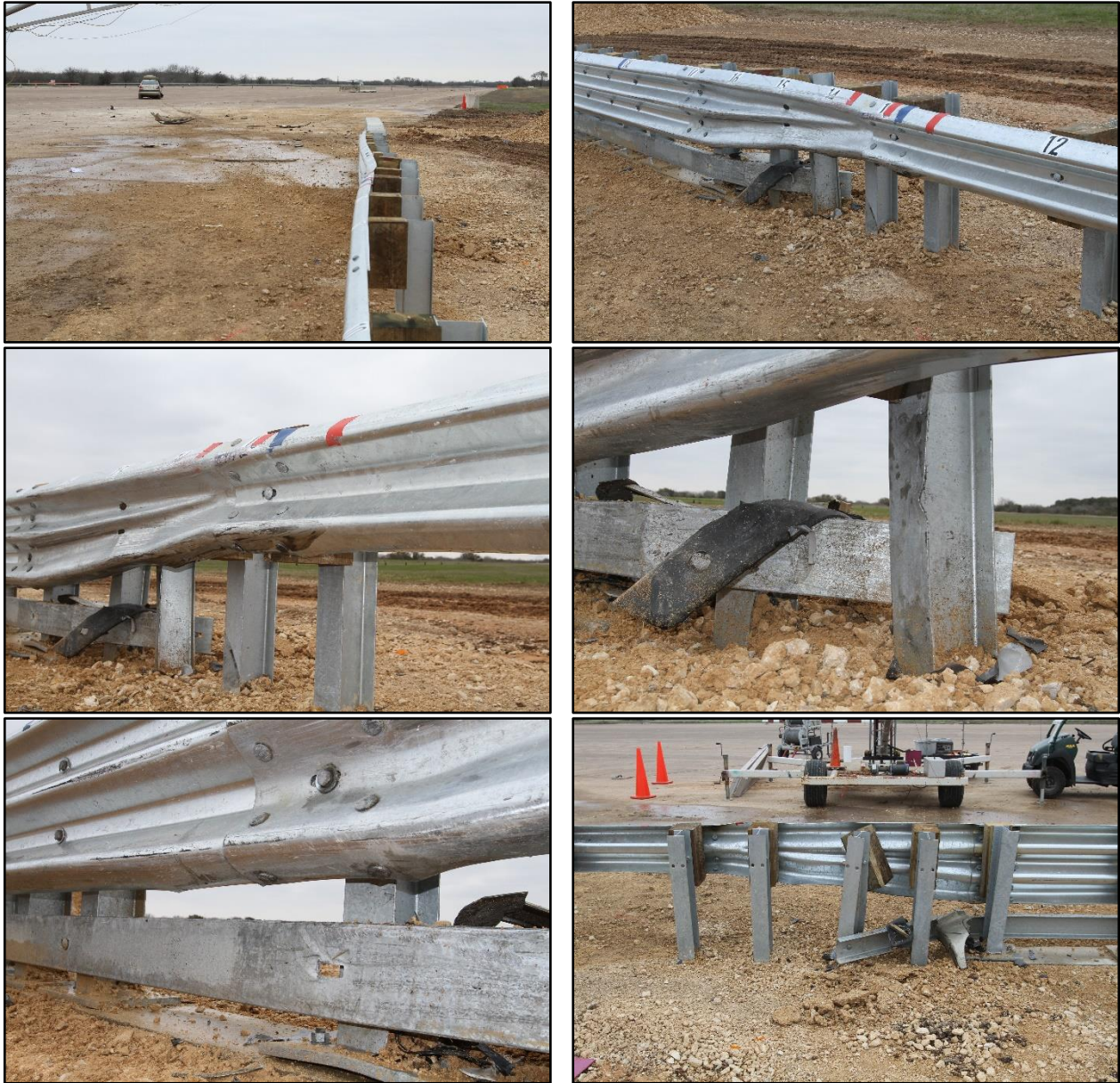
Figure 7.5. Upstream Transition after Test No. 469549-01-1.
