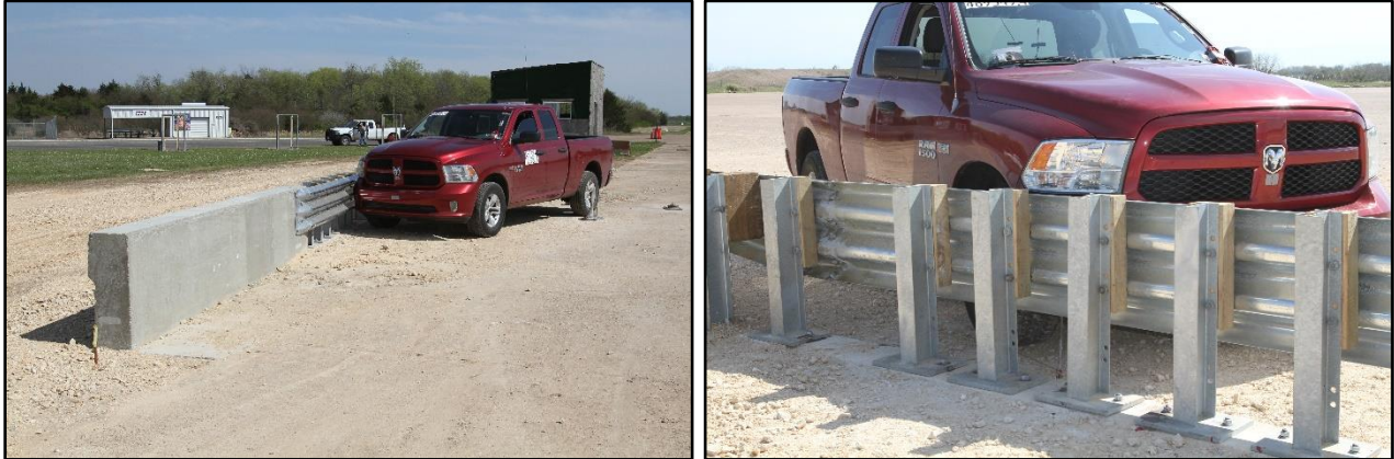
Figure 8.1. Downstream Transition/Test Vehicle Geometrics for Test No. 469549-01-4.
