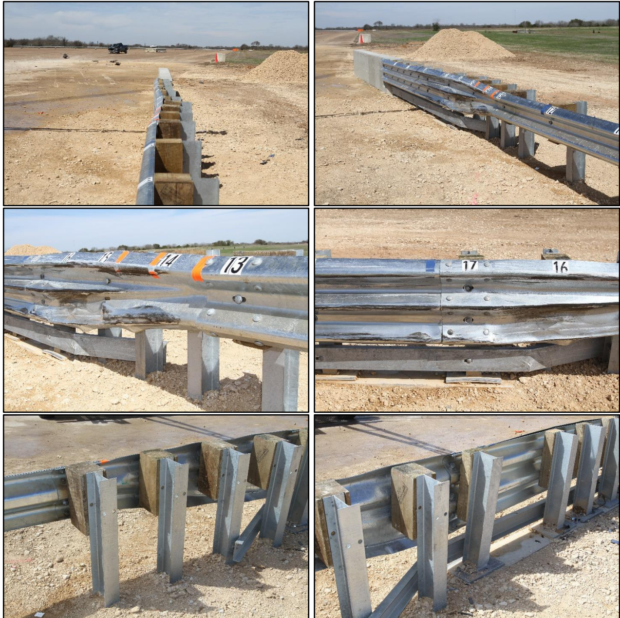
Figure 7.11. Upstream Transition after Test No. 469549-01-2.
