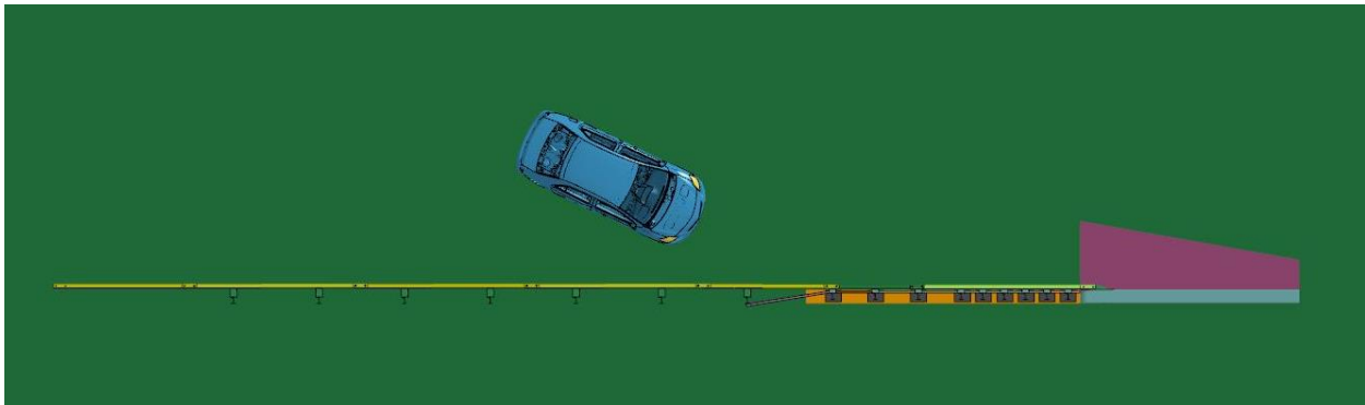
Figure 4.17. MASH 1100C Vehicle/Installation Setup – Top View.
