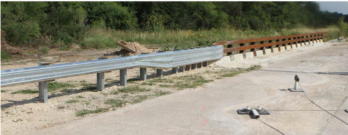
Figure 2.9. T131RC Bridge Rail Transition Impact View.
