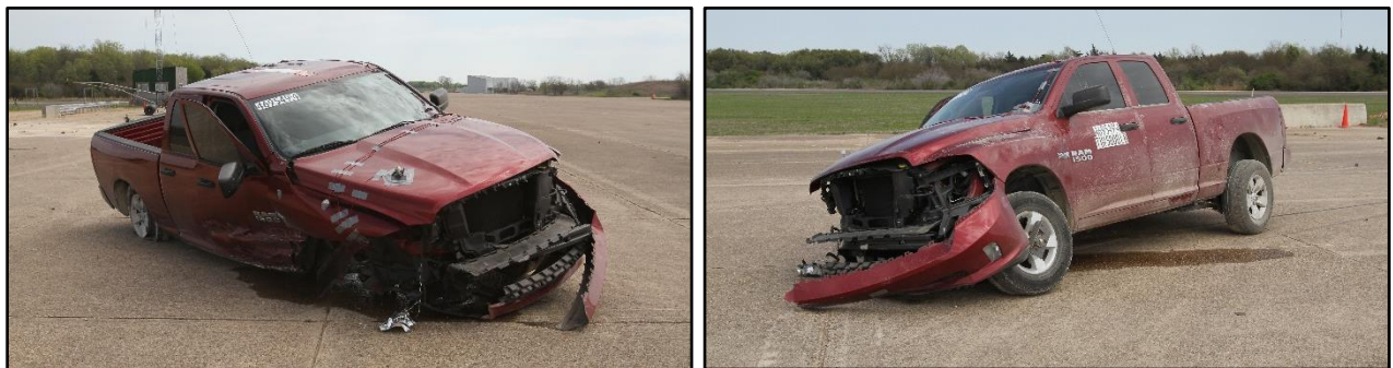
Figure 8.4. Test Vehicle after Test No. 469549-01-4.
