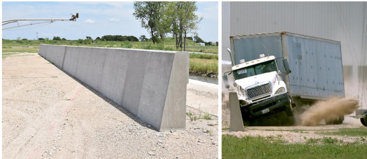
Figure 1. MASH Test 5-12 on 54-Inch-Tall SSCB with the Drilled Shaft Foundation.
