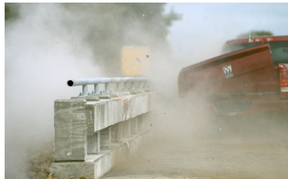
Figure B.2. Sequential Photographs for Test No. 469469-2-1 (Rear View).
