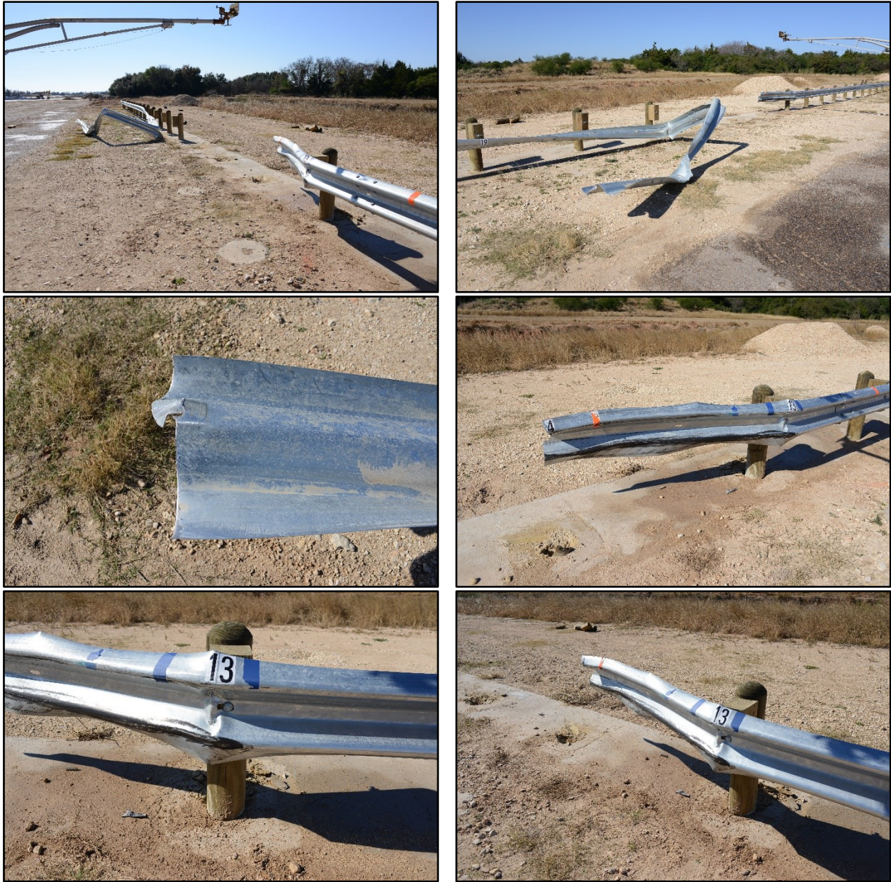
Figure 12.5. Round Wood Post Guardrail in a Concrete Mow Strip after Test No. 469469-11.
