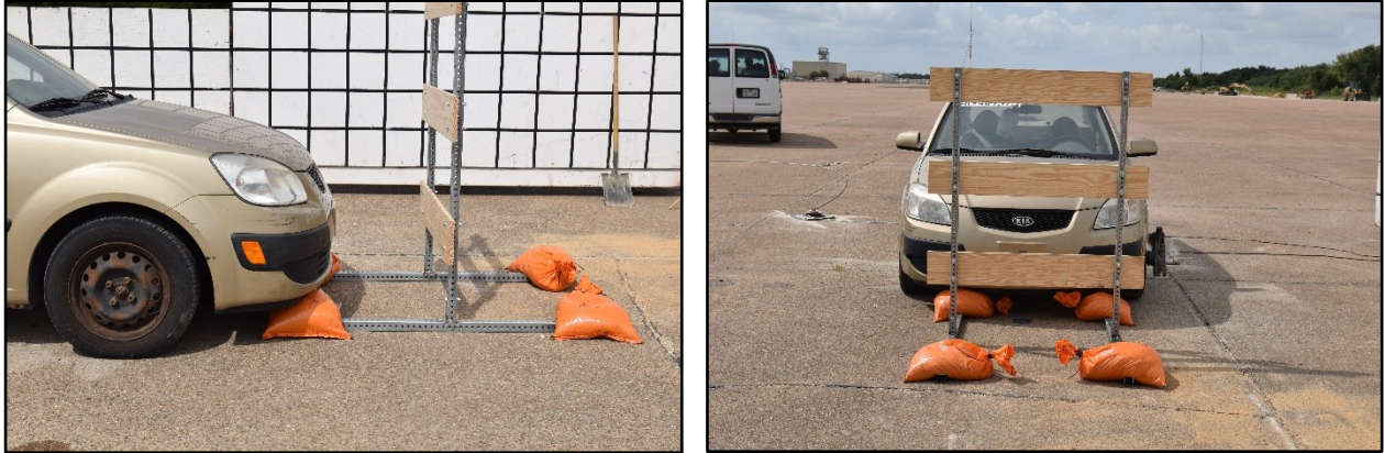
Figure 13.21. Type III Barricade/Test Vehicle Geometries for Test No. 469469-12-04.
