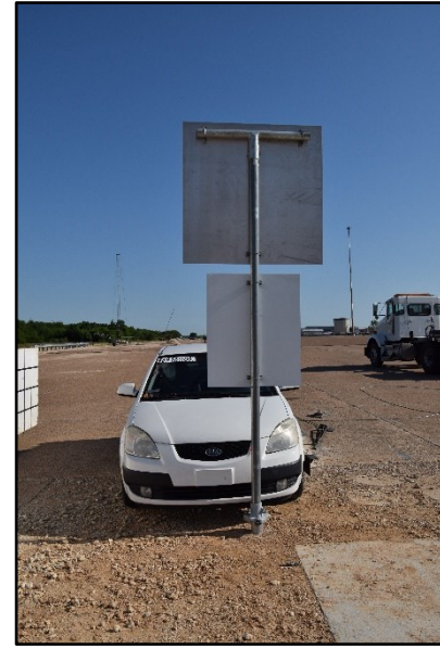
Figure 9.3. Burn Ban Sign with Slip Base Test Vehicle Geometries for Test No. 469469-08-01.
