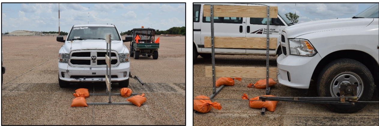
Figure 13.9. Type III Barricade/Test Vehicle Geometries for Test No. 469469-12-02.
