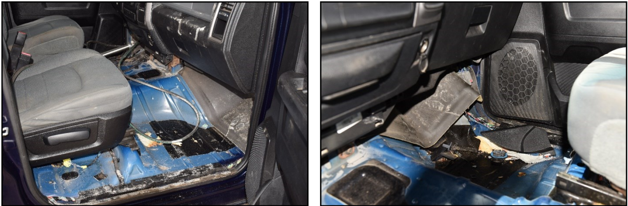
Figure 6.7. Interior of Test Vehicle for Test No. 469469-5 (before Test on Left; after Test on Right).
