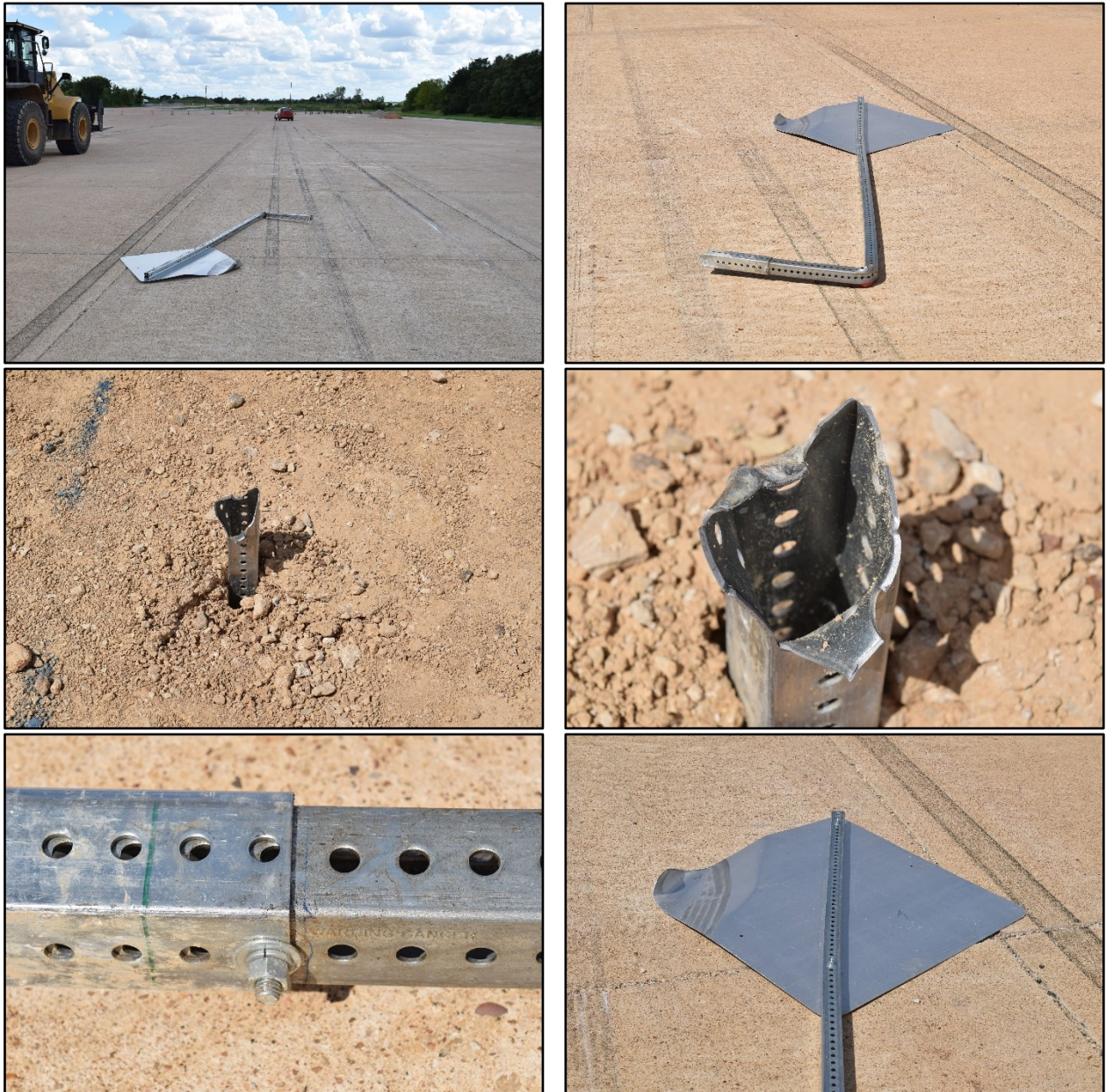
Figure 8.5. PSST Sign Support in Anchor Stub System after Test No. 469469-07-02.
