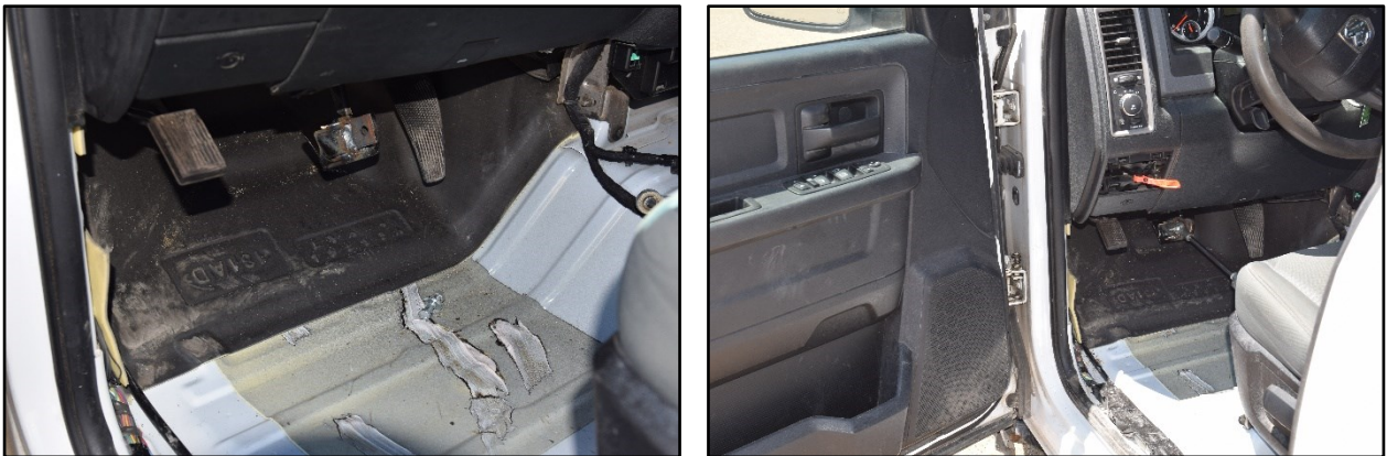
Figure 4.7. Interior of Test Vehicle for Test No. 469469-3-2 (before Test on Left; after Test on Right).
