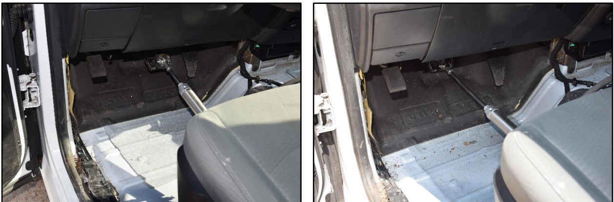
Figure 5.13. Interior of Test Vehicle for Test No. 469469-4-2 (before Test on Left; after Test on Right).
