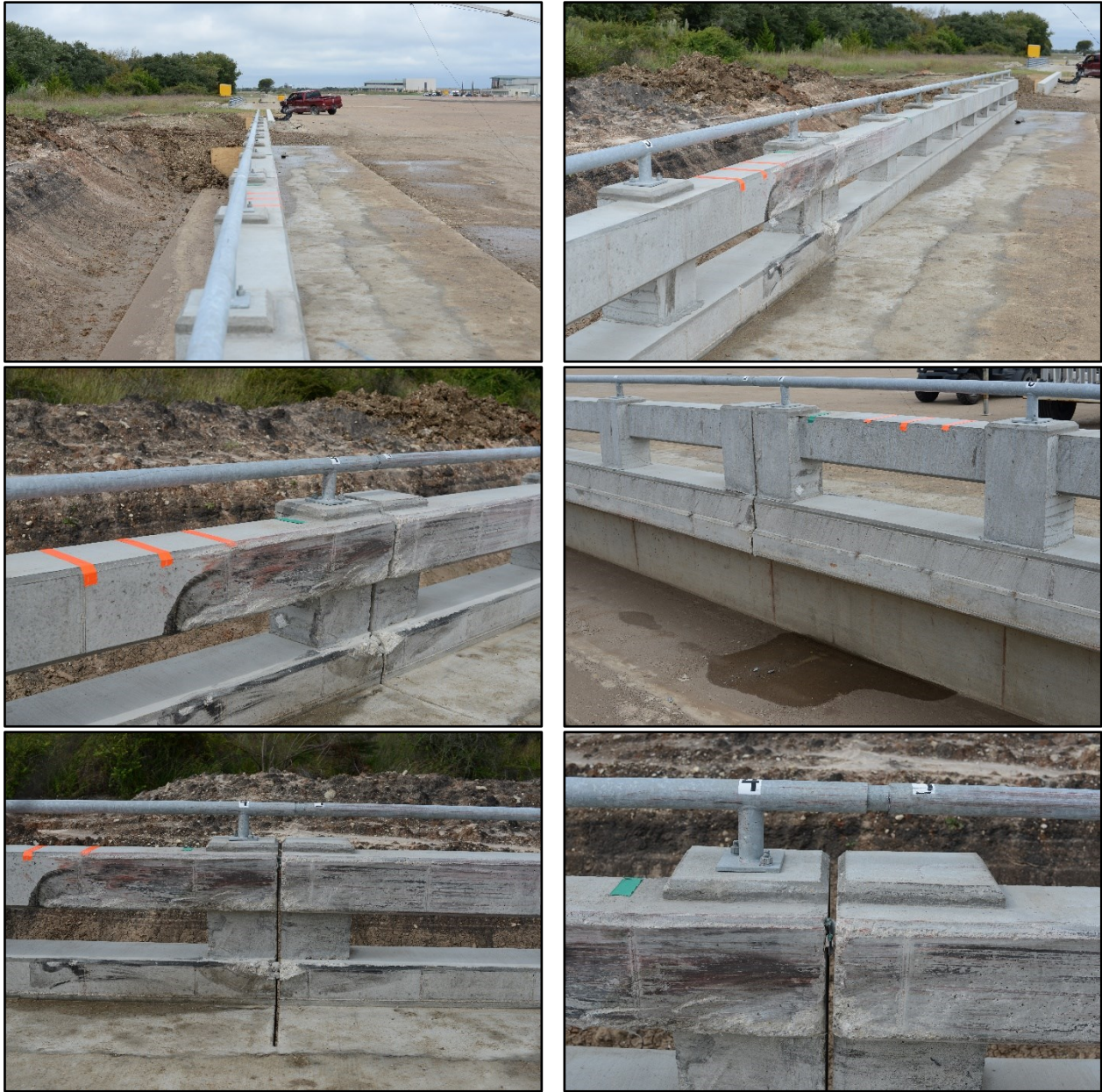
Figure 3.5. Modified C66 Bridge Rail after Test No. 469469-2-1.
