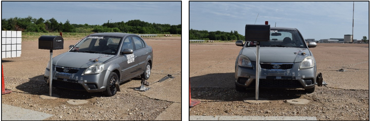
Figure 11.12. Extra-Large Mailbox on Thin-Wall Galvanized Tube with Type 2 Foundation/Test Vehicle Geometrics for Test No. 469469-10-2.
