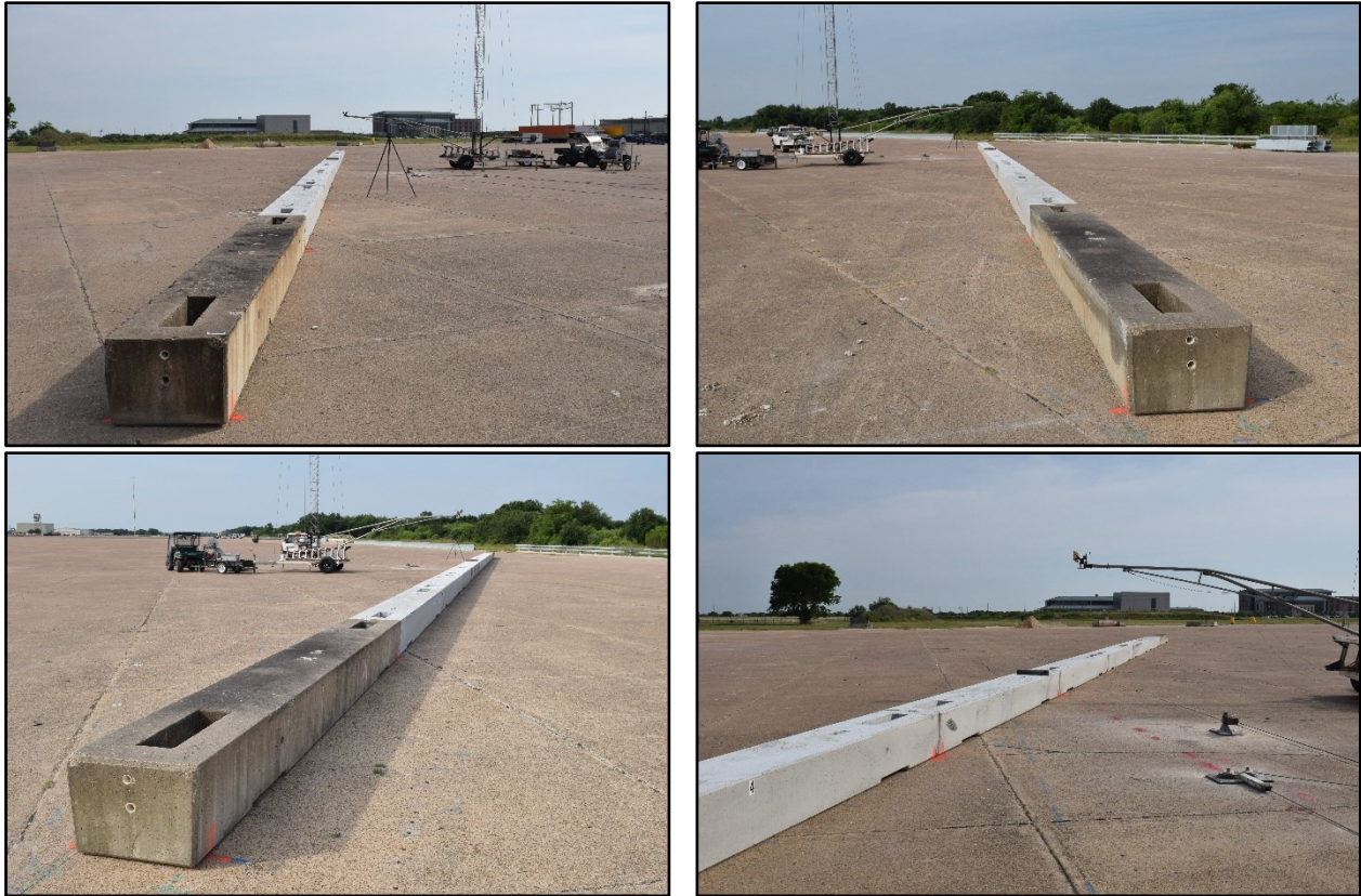
Figure 4.2. Low-Profile Barrier prior to Testing.
