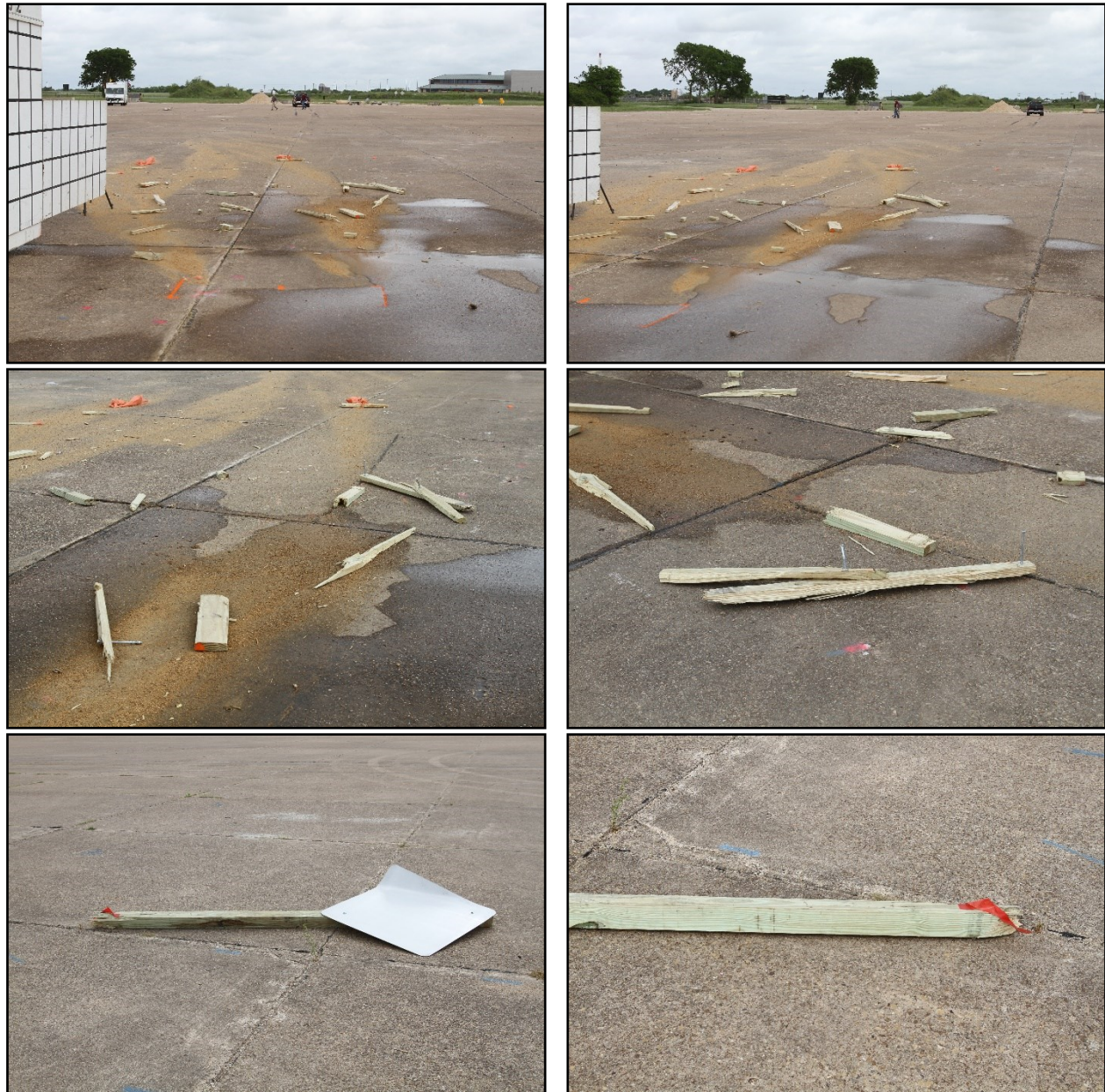
Figure 7.5. Single Wood Post Skid-Mounted Sign after Test No. 469469-06-02.
