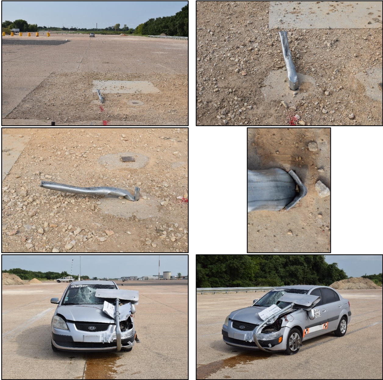
Figure 10.5. Burn Ban Sign on Wedge and Socket Support after Test No. 469469-09-01.
