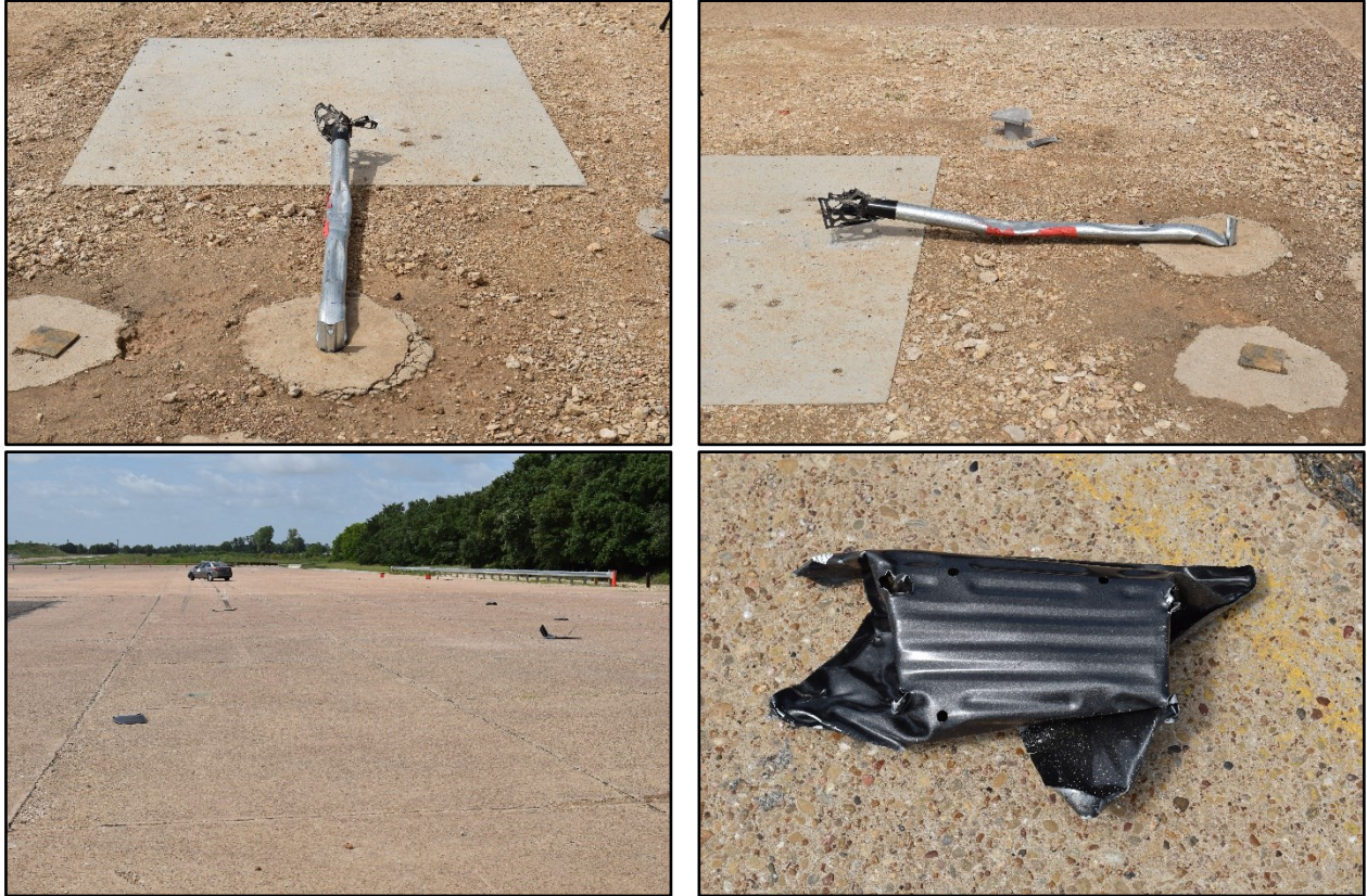
Figure 11.14. Extra-Large Mailbox on Thin-Wall Galvanized Tube with Type 2 Foundation after Test No. 469469-10-2.
