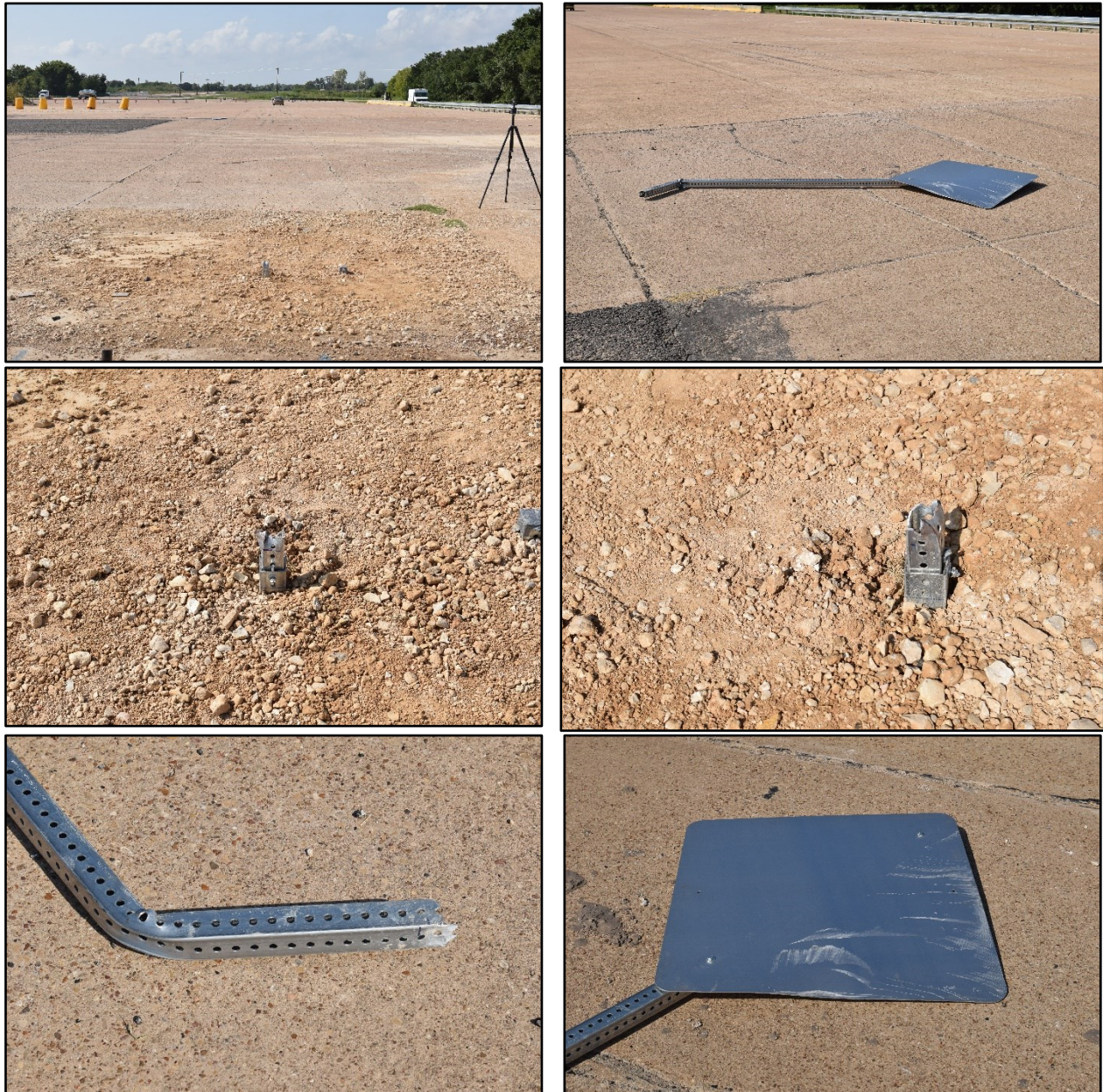
Figure 8.13. PSST Sign Support in Anchor Stub System after Test No. 469469-07-05.
