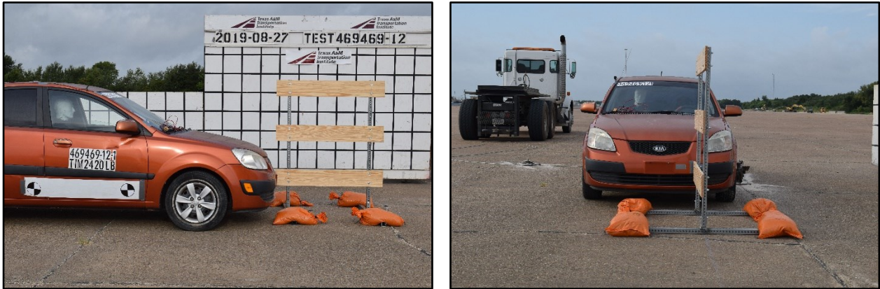
Figure 13.3. Type III Barricade/Test Vehicle Geometrics for Test No. 469469-12-01.
