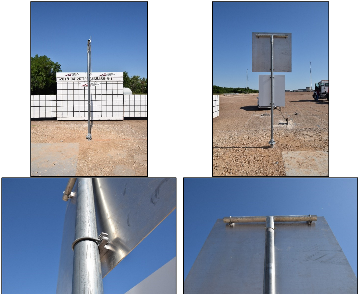
Figure 9.2. Burn Ban Sign on Slip Base Support prior to Test No. 469469-08-01.
