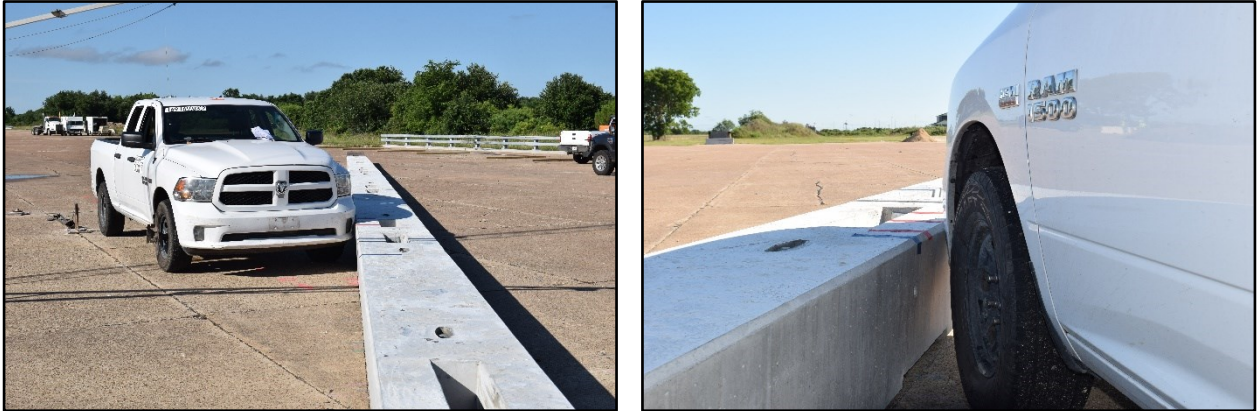
Figure 4.3. Low-Profile Barrier/Test Vehicle Geometrics for Test No. 469469-3-2.
