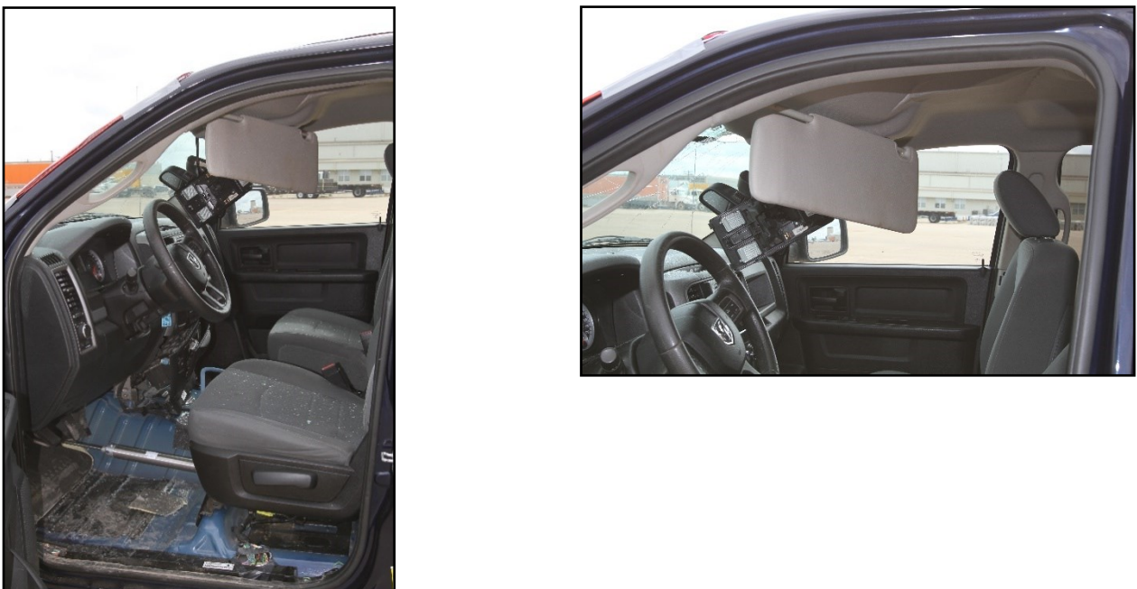
Figure 7.7. Interior of Test Vehicle after Test No. 469469-06-02.
