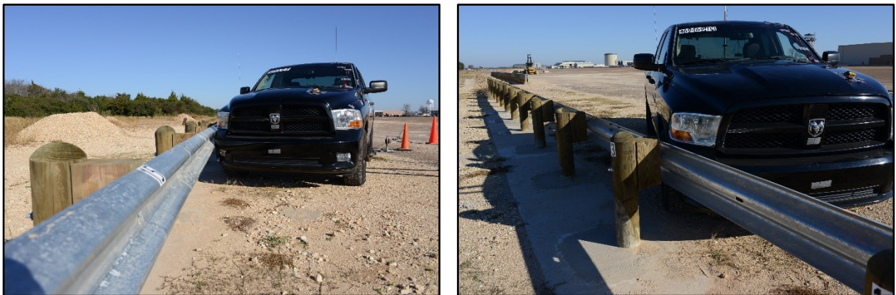
Figure 12.3. Round Wood Post Guardrail in Concrete Mow Strip/Test Vehicle Geometries for Test No. 469469-11.
