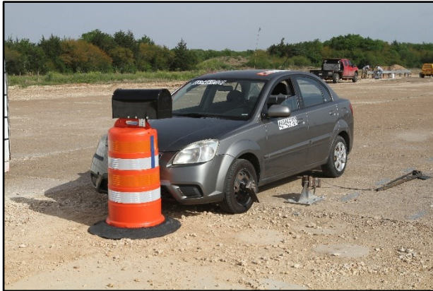
Figure 11.4. Single Temporary Mailbox on Plastic Drum/Test Vehicle Geometrics for Test No. 469469-10-1.
