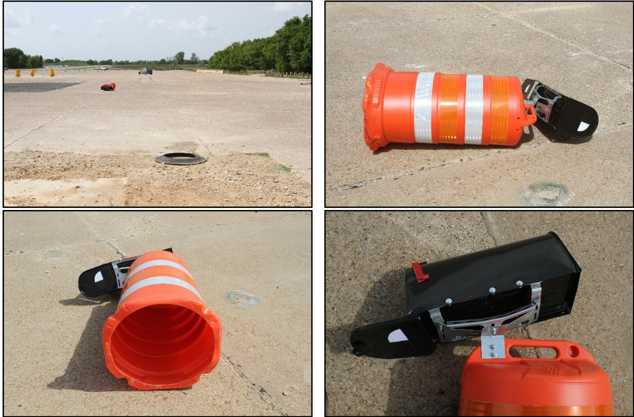
Figure 11.6. Single Temporary Mailbox on Plastic Drum after Test No. 469469-10-1.
