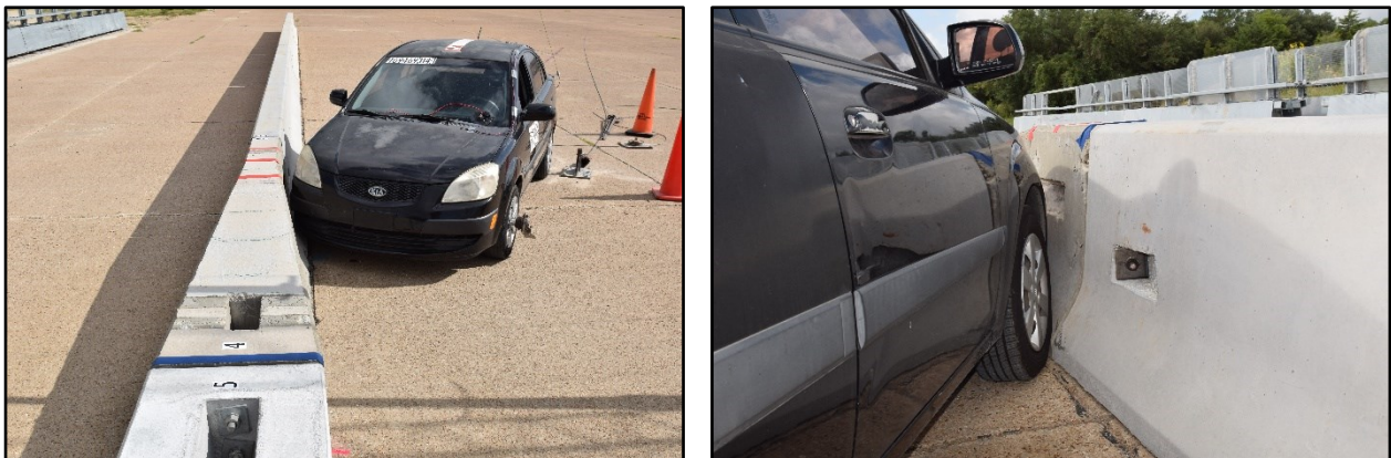
Figure 5.3. Low-Profile-to-F-Shape Transition/Test Vehicle Geometrics for Test No. 469469-4-1.
