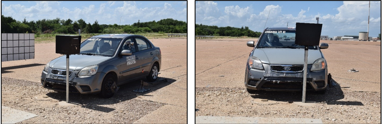
Figure 11.20. Lockable Mailbox on Thin-Wall Galvanized Tube with Type 2 Foundation/Test Vehicle Geometrics for Test No. 469469-10-3.
