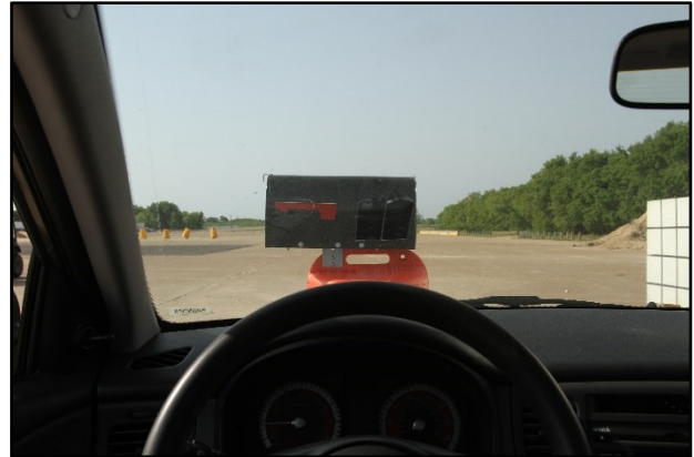
Figure 11.4. Single Temporary Mailbox on Plastic Drum/Test Vehicle Geometrics for Test No. 469469-10-1.
