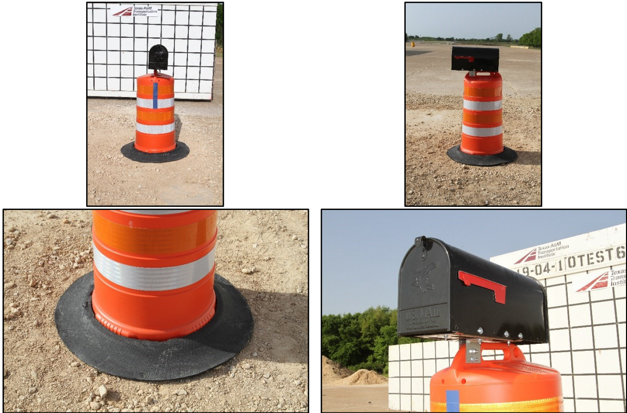
Figure 11.3. Single Temporary Mailbox on Plastic Drum prior to Testing.
