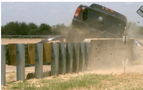
Figure E.2. Sequential Photographs for Test No. 469469-5 (Rear View).
