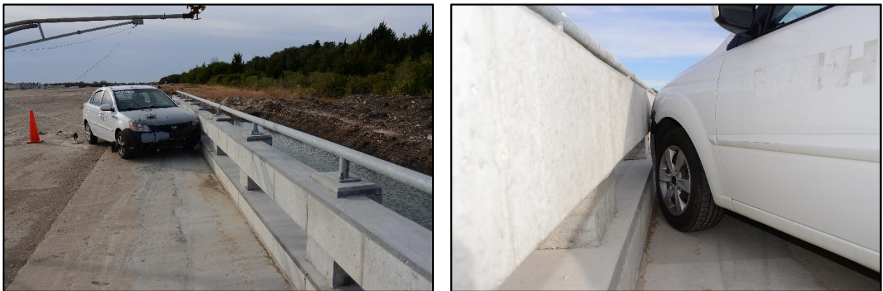
Figure 3.9. Modified C66 Bridge Rail/Test Vehicle Geometrics for Test No. 469469-2-2.
