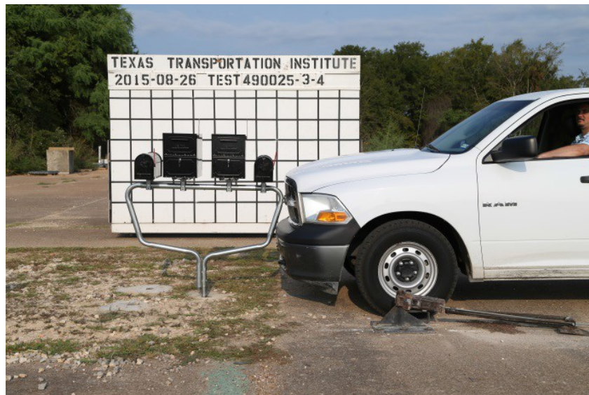
Figure 11.1. Mailbox Geometrics with 2270P Pickup Truck (9).
