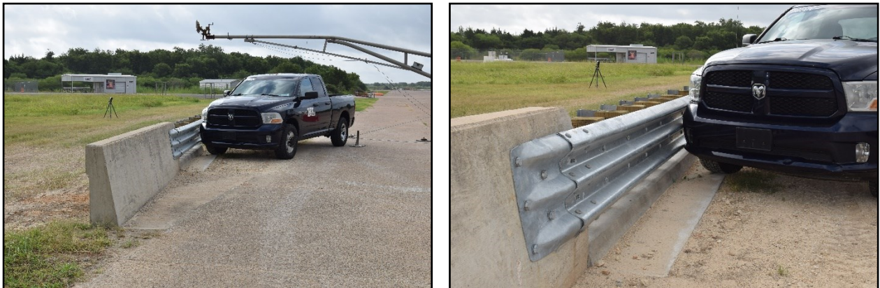
Figure 6.3. Thrie-Beam Transition without End Shoe Block/Test Vehicle Geometries for Test No. 469469-5.
