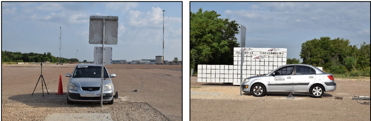
Figure 10.3. Burn Ban Sign on Wedge and Socket Support Test Vehicle Geometrics for Test No. 469469-09-01.
