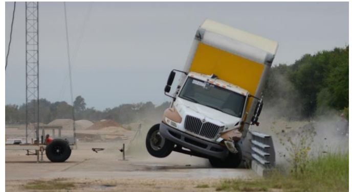
Figure 1. MASH Test 4-12 on the TxDOT C1W Bridge Rail.
