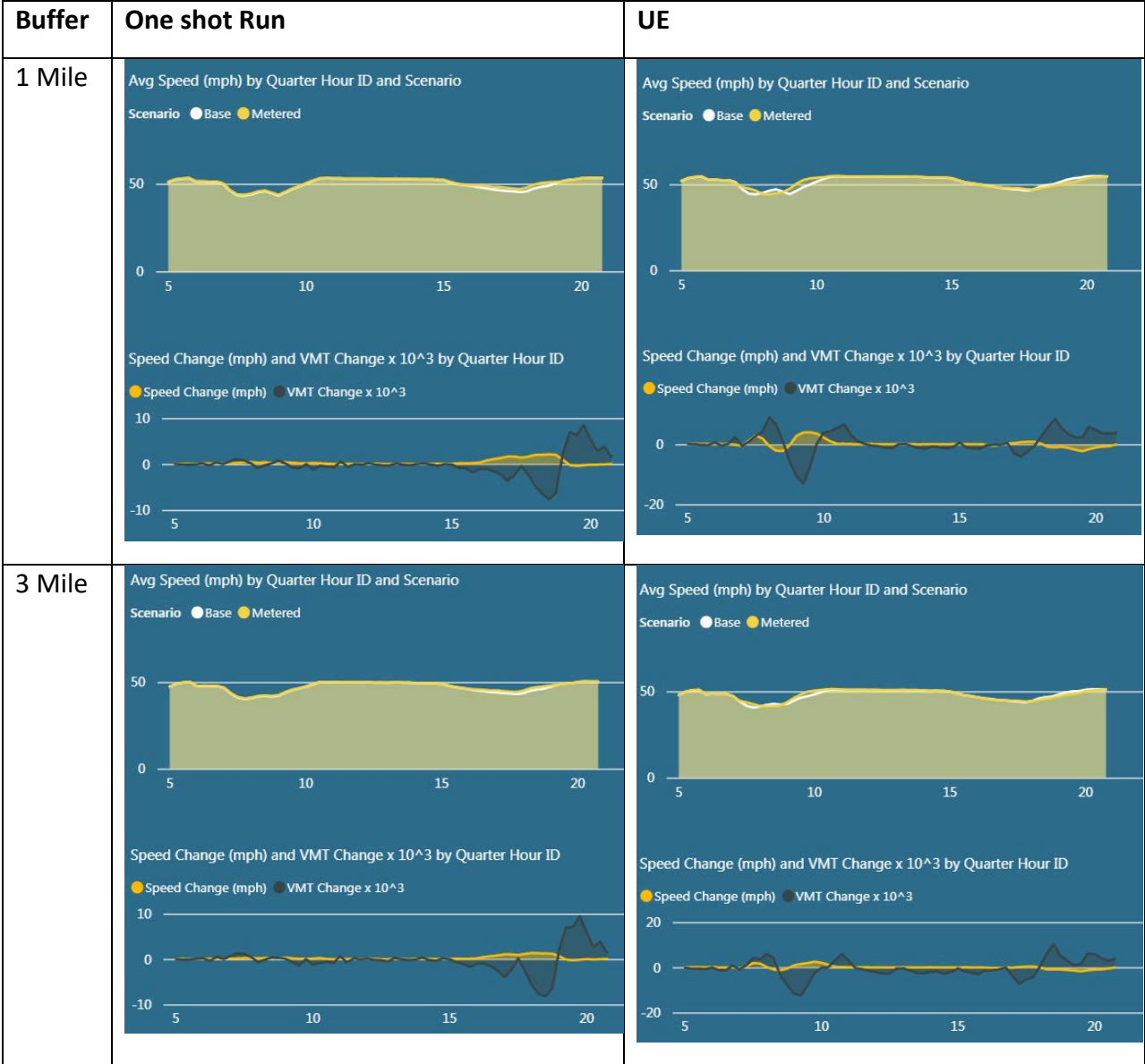
Figure D5. WB I-20 MOEs for Meso Limits and Buffer Size of 1- and 3-Miles.
