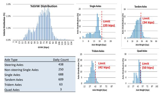
Figure C-16. Portable WIM Data Analysis (US 83 NB, RM 678-680, Webb County, LRD).
