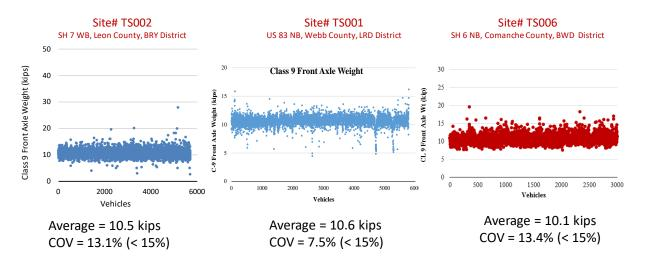
Figure 10. Portable WIM Data Variability Analysis (Class 9 Steering Axle-Wheel Weight).
