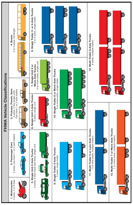
Figure C-1. FHWA Vehicle Classification System.
