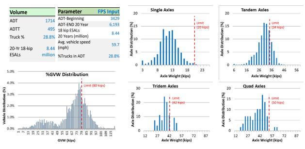
Figure C-13. Portable WIM Data Analysis (US 83 NB, LRD).
