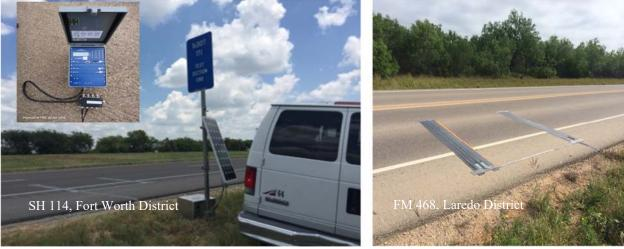
Figure 4. Portable WIM Setup—SH 114 and FM 468.
