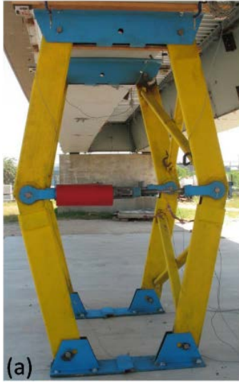
Figure 3.13. Scissor Jack with Explosive Tie Assembly (Neuman 2009).
