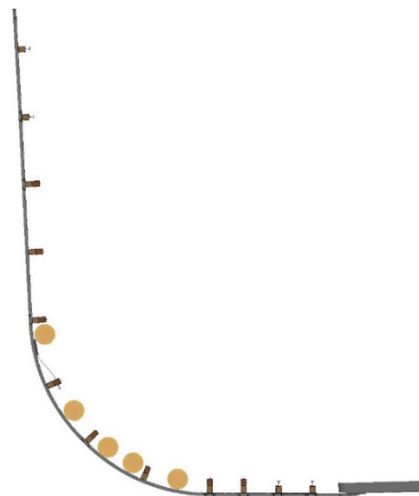
Figure 3.15. Tension Cable and Five 700-lb Sand Drums.
