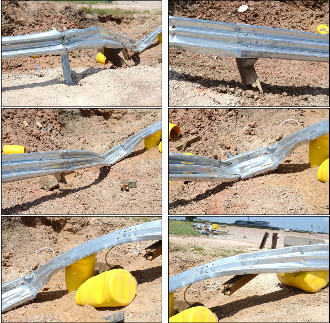
Figure 7.5. Damage to Nose after Test No. 469137-3-1.
