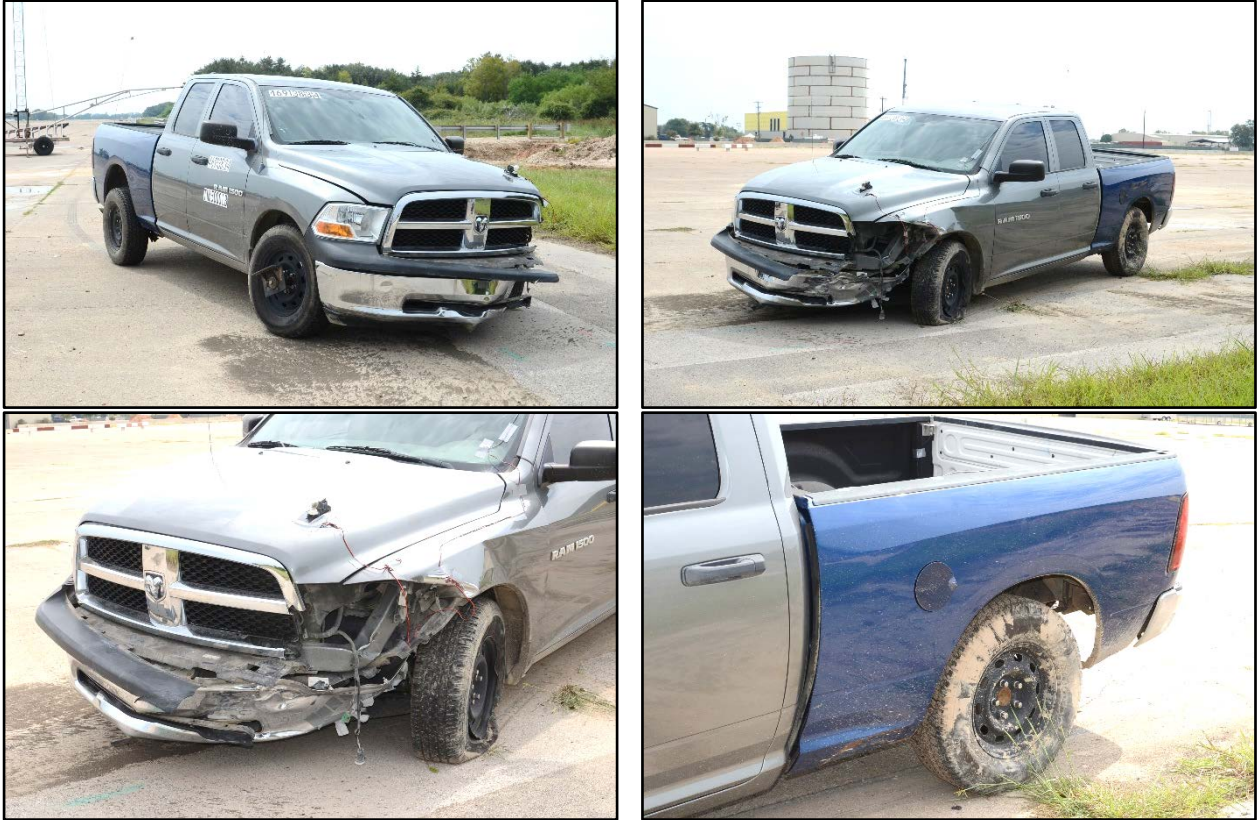
Figure 10.6. Test Vehicle after Test No. 469138-3-4.
