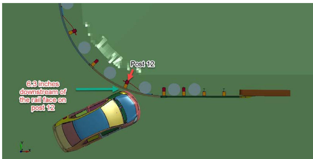
Figure 5.5. Target CIP for Modified MASH Test 2-34 on the TxDOT Low-Speed Short Radius Guardrail Treatment.
