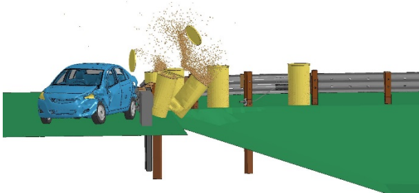
Figure 3.59. Sequential Images of Car Simulation with Two Tension Cables and Six 700-lb Sand Drums.
