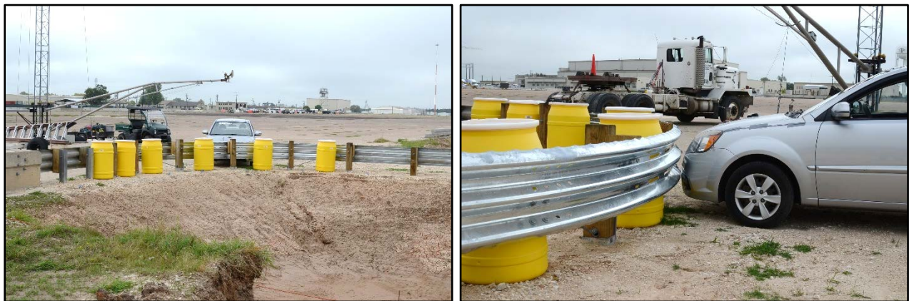
Figure 8.1. TxDOT Low-Speed Short Radius Guardrail Treatment/Test Vehicle Geometrics for Test No. 469137-3-2.
