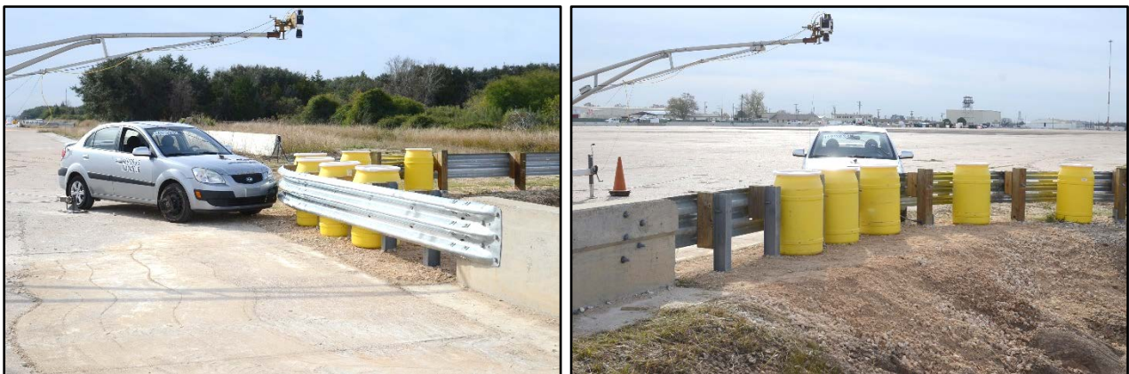
Figure 11.1. TxDOT Low-Speed Short Radius Guardrail /Test Vehicle Geometrics for Test No. 469138-3-5.
