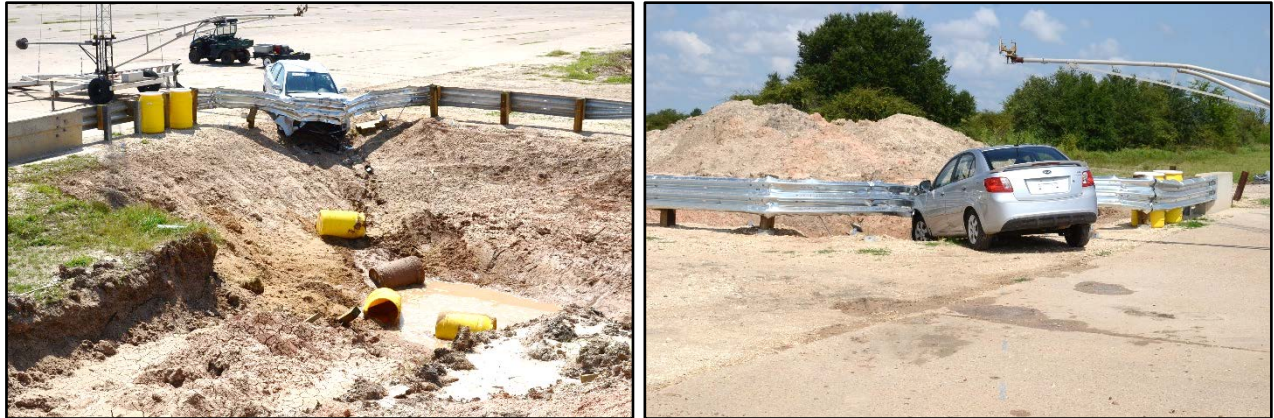
Figure 8.3. TxDOT Low-Speed Short Radius Guardrail Treatment and Test Vehicle after Test No. 469137-3-2.
