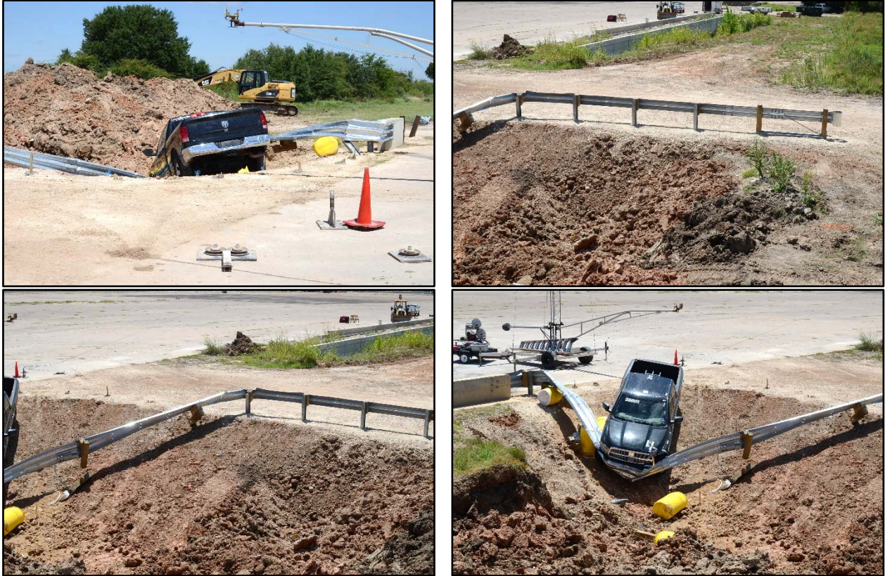
Figure 7.3. TxDOT Low-Speed Short Radius Guardrail Treatment after Test No. 469137-3-1.
