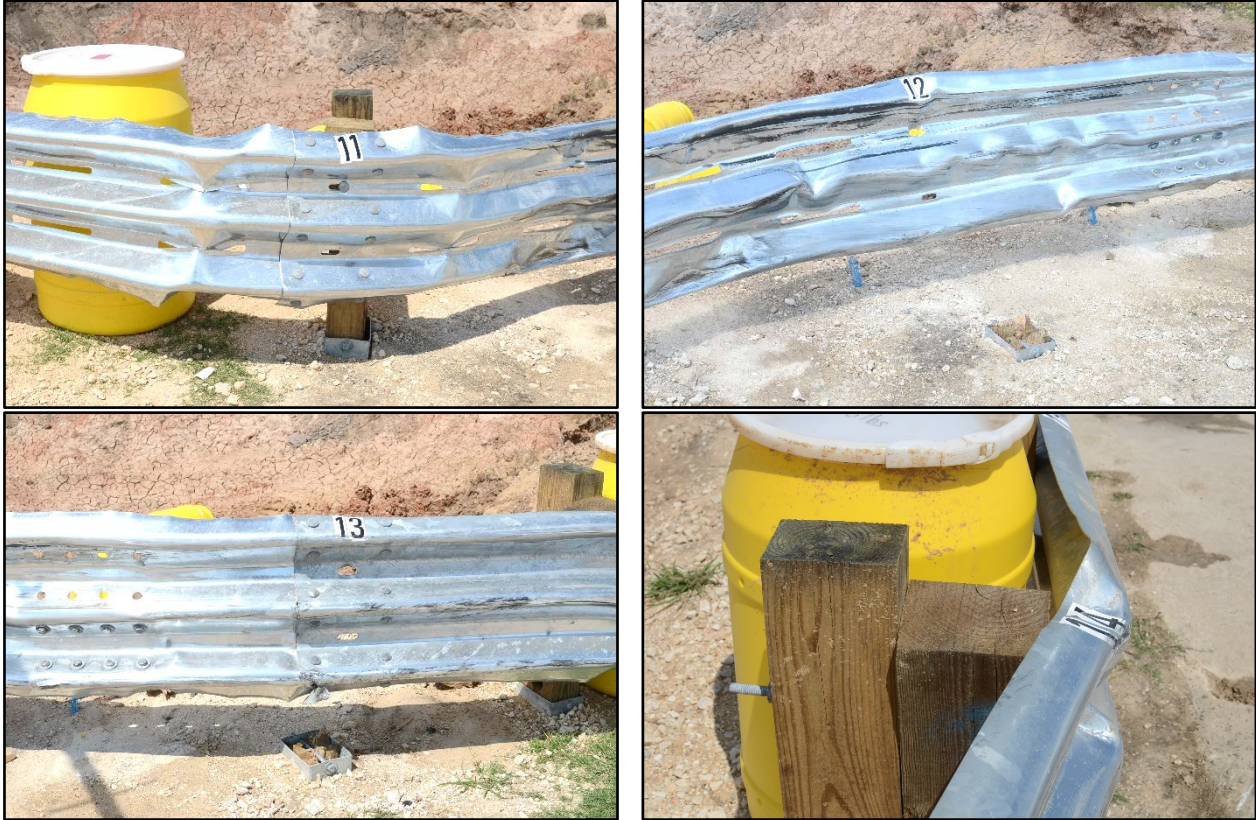
Figure 9.5. Damage to Rail Section Parallel to Roadway after Test No. 469138-3-3.
