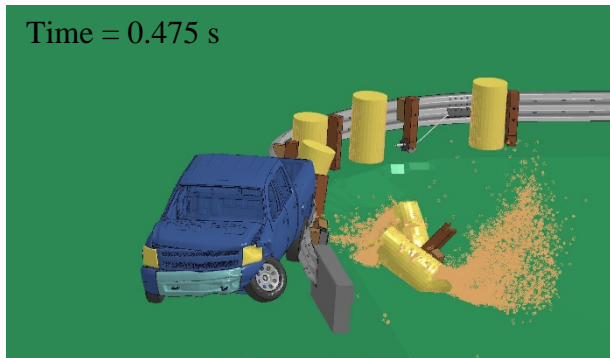
Figure 3.32. Sequential Images of Truck Simulation with Two Tension Cables and Six 700-lb Sand Drums.
