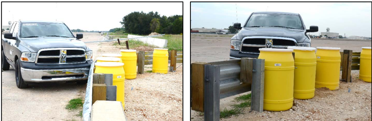
Figure 10.1. TxDOT Low-Speed Short Radius Guardrail Treatment/Test Vehicle Geometrics for Test No. 469138-3-4.
