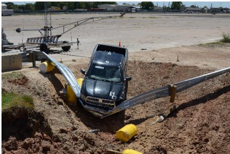
Figure 2. Pickup Truck Resting Position after Impacting the Nose of the New TL-2 Short Radius Design.
