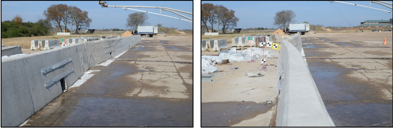
Figure 11.3. TxDOT Rubber Mounted Single Slope Barrier/Test Vehicle after Test No. 468958-3.
