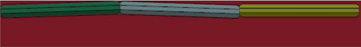
Figure 4.29. Deflection of Barrier System (Three 60-ft Segments – Two Rubber Fenders).
