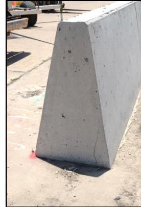
Figure 5.47. Right End and Field Side of Barrier after Test No. 468957-B10.
