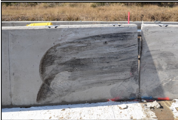
Figure 10.4. Damage to Barrier #1 after Test No. 468958-2.
