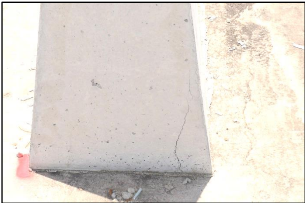
Figure 5.48. Left End and Traffic Side of Barrier after Test No. 468957-B10.
