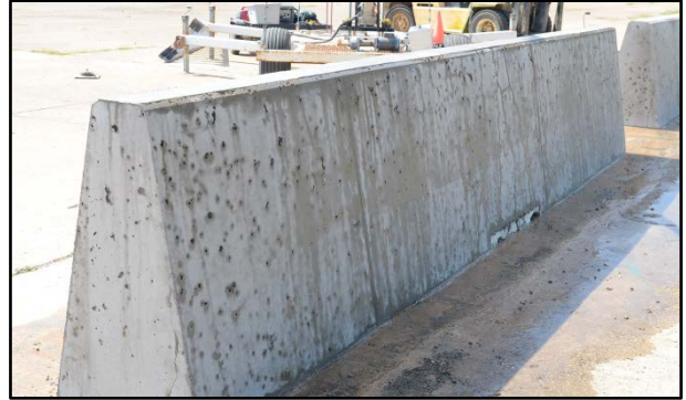
Figure 5.38. Right End and Field Side of Barrier after Test No. 468957-B9.
