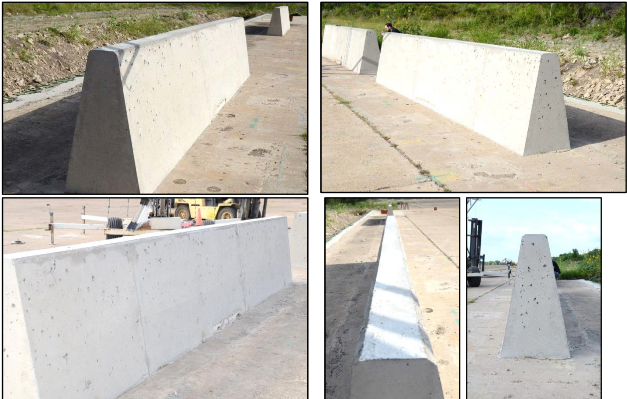
Figure 5.37. PR5FCR5F Mix Concrete Barrier before Test No. 468957-B9.
