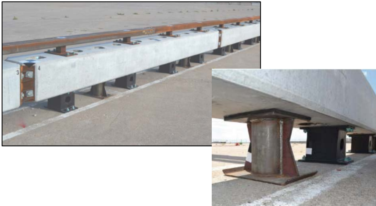
Figure 2.22. Concrete Beam Barrier with Alternating Steel and Rubber Post from MwRSF.
