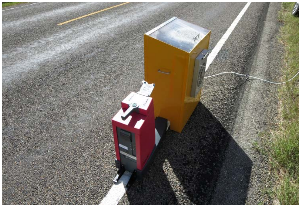
Figure 48. Continuous Wetting Test Setup on Profiled Marking.
