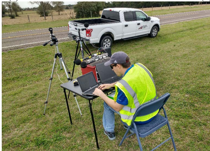
Figure 24. Noise Measurement Equipment: (a) Interior Microphone, (b) OBSI System (Only Leading Edge Enabled), and (c) Wayside Noise System.
