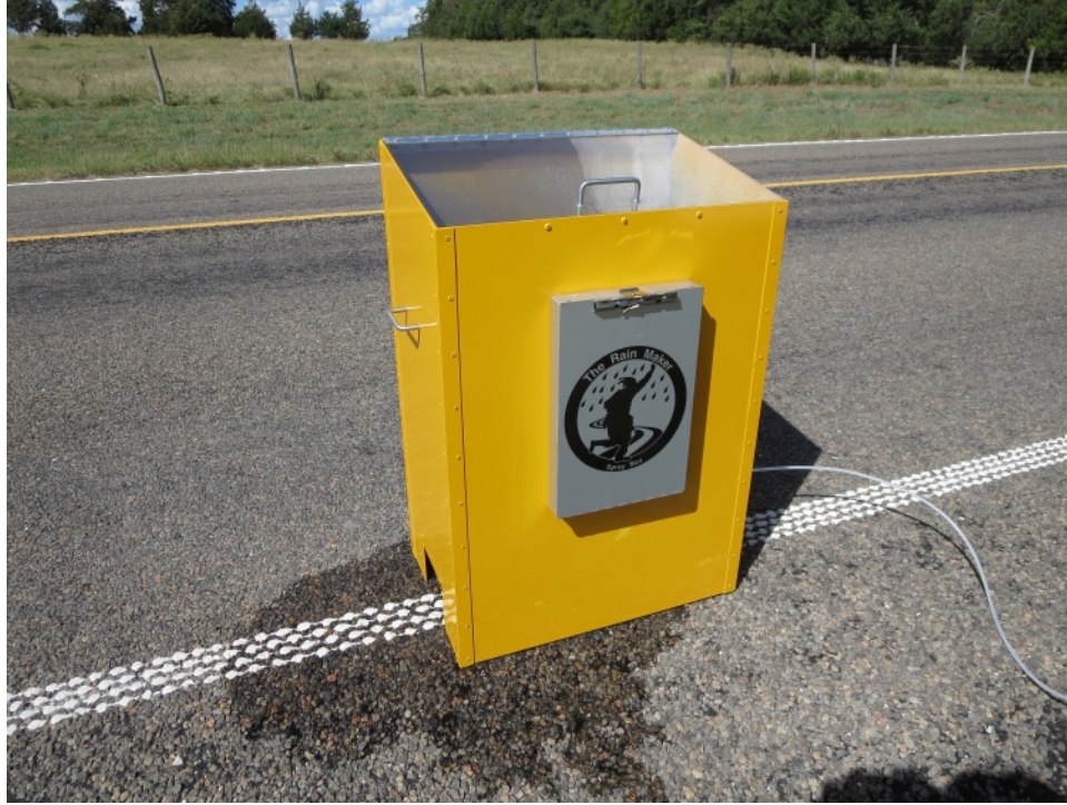
Figure 49. Continuous Wetting Setup after Test.
