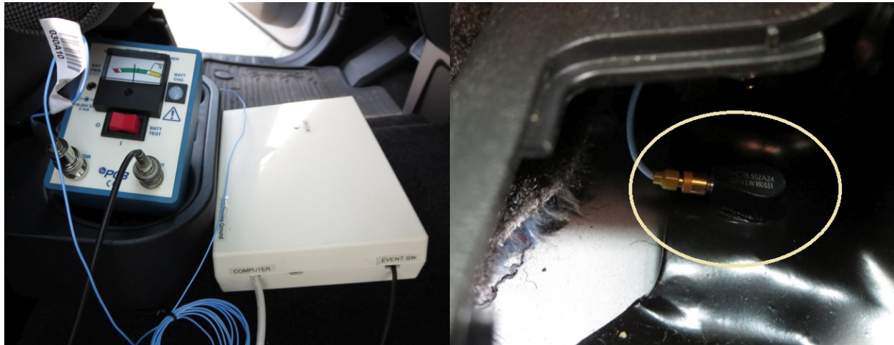
Figure 37. Vibration Data Collection Setup.
