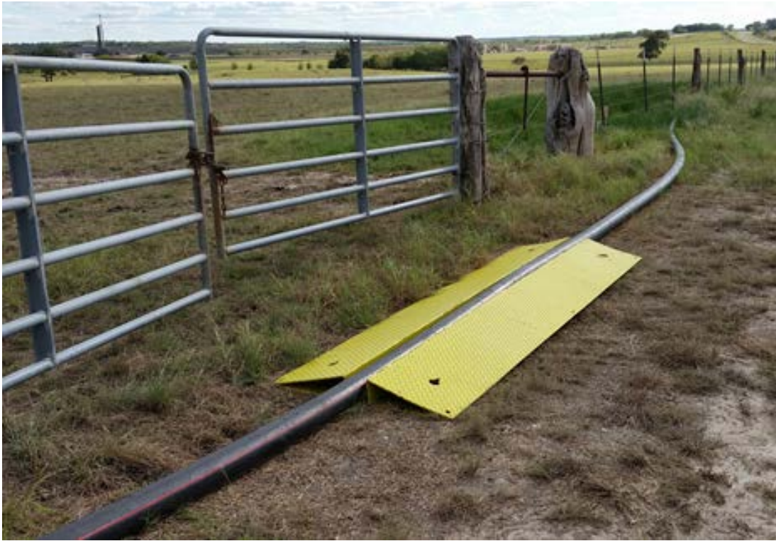
(a) Crossing ramp
