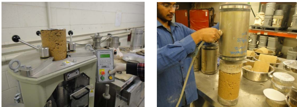
Figure 6. Extruding Sample from SGC and Placing a Triaxial Cell.
