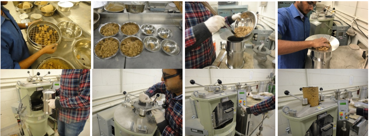
Figure 11. Key Steps in Compacting Base/Soil Materials with SGC.
