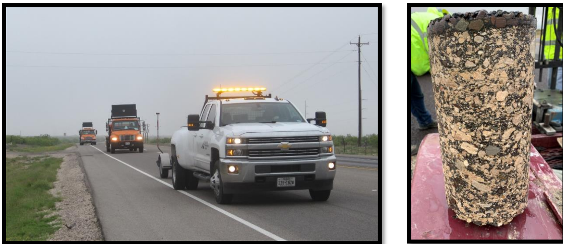
Figure 9. FWD Collection and Core from FDR Layer.
