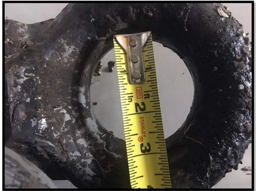
Loop at end of tow bars must mate to pintle hitch on transports
