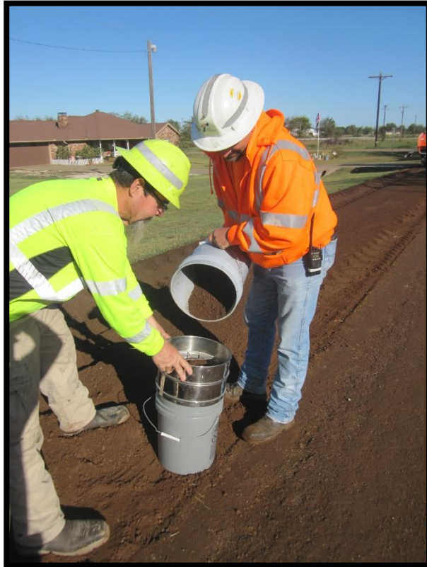
100% passing 1 \frac{3}{4} -in. sieve. 85% (min.) passing \frac{3}{4} -in. sieve
