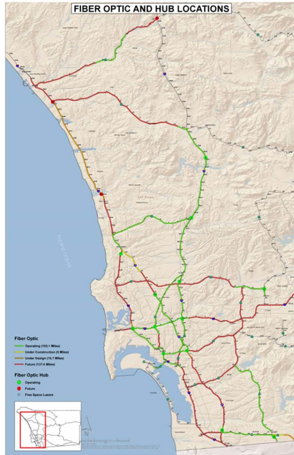
Figure 20. Fiber Optic and Hub Locations in District 11 TMC.
