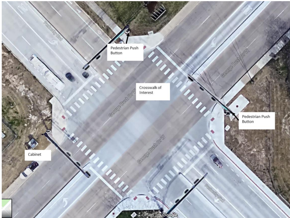
Figure 6. Pedestrian Push Button Locations at GBD/PB.
