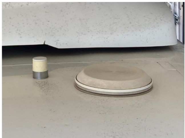
Figure 13. Radio Antennae Placement of Bus Roof.
