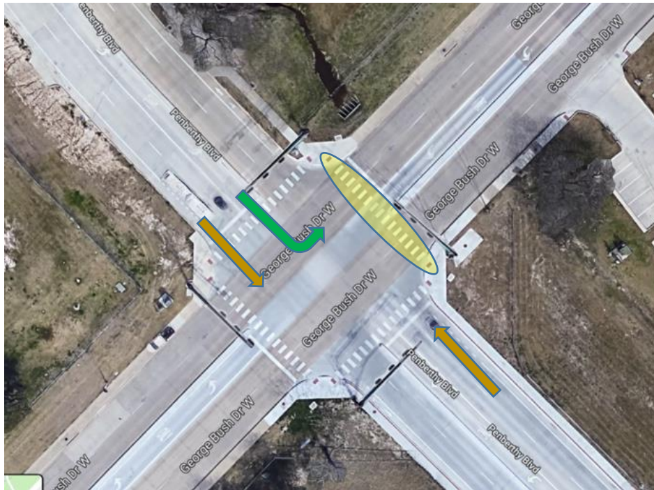
Figure 3. Crosswalk of Interest and Path of Left-Turning Buses.
