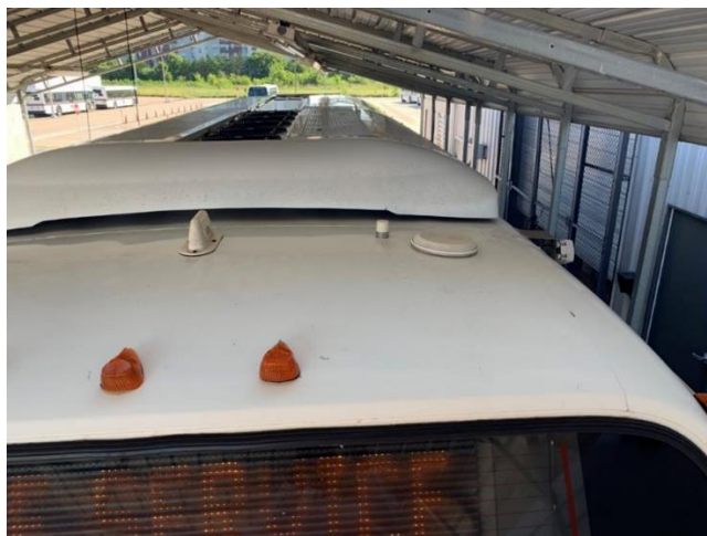
Figure 13. Radio Antennae Placement of Bus Roof.
