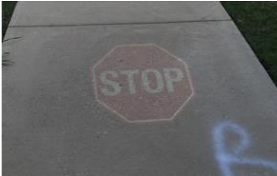
Figure 18. Projected Warning Sign.
