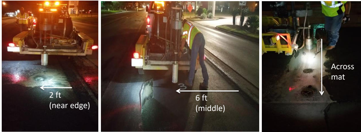
Figure 74. Extraction of field cores at different locations in the mat.
