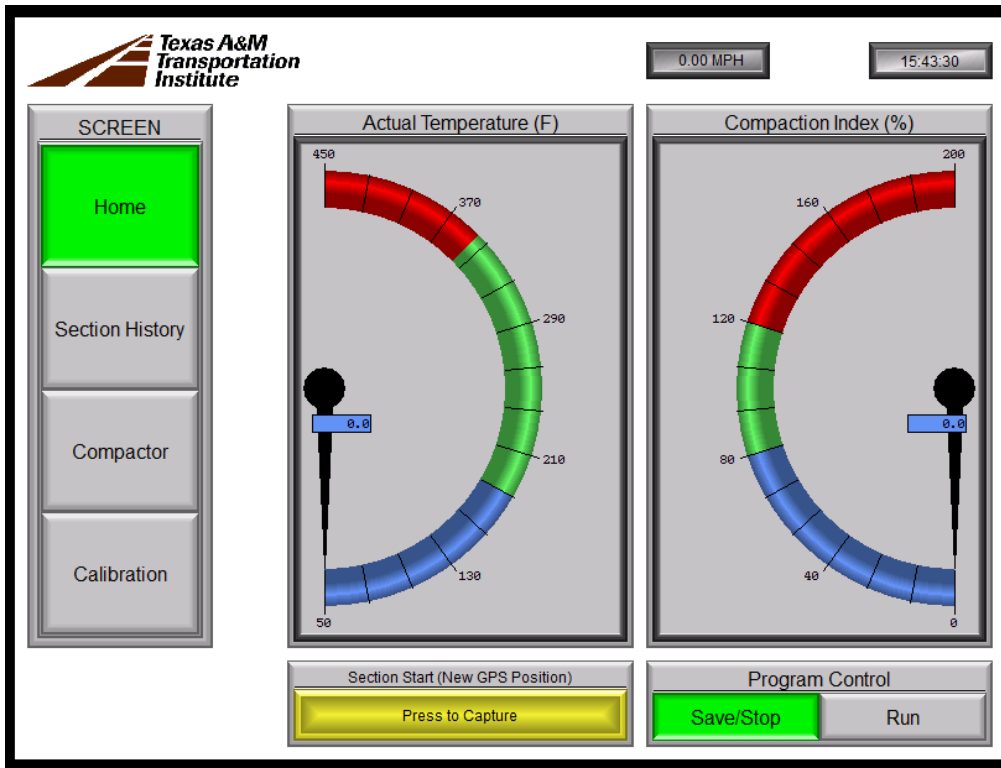
Figure 66. Version 3 (final) of HMI main (Home) screen (optimized for 6-inch HMI).
