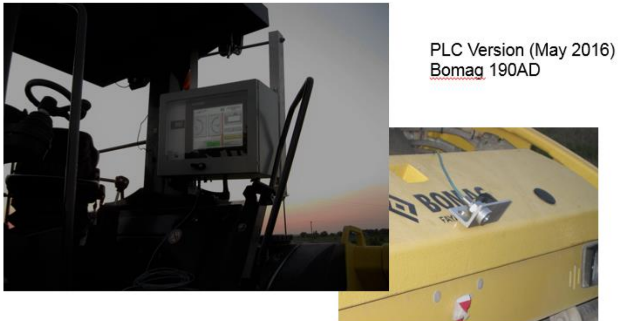
Figure 58. PLC version mounted on Bomag compactor.
