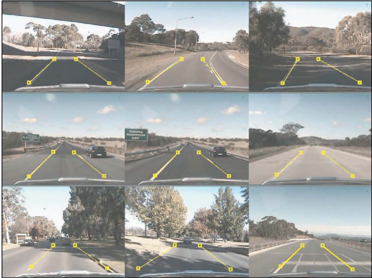
Figure 17. Lane Tracking Algorithms Showing the Estimated Lane Boundary against Shadows, Obstacles, and Misleading Markings (71).
