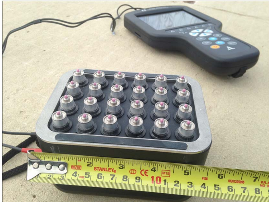
Figure 132. Transducer Array (Foreground) with EyeCon Handheld Computer (Background).
