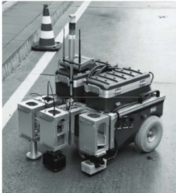
Figure 130. BetoScan Automated Robot (Reichling et al., 2009).
