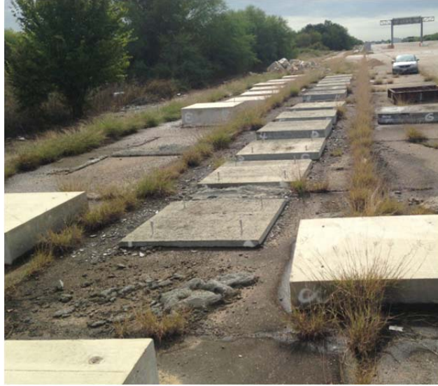
Figure 27. Concrete and Shotcrete Specimens at Texas A&M University Riverside Campus, Bryan, TX.
